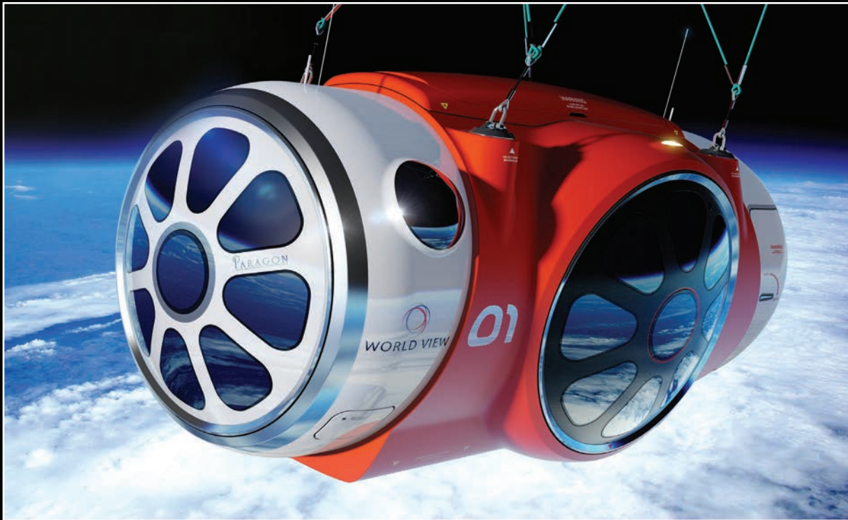
The cabin is a pressure vessel similar in design to the modules that form the living and working quarters of the ISS. Inspired by the space station's cupola, the expansive windows allow for maximum viewing.
