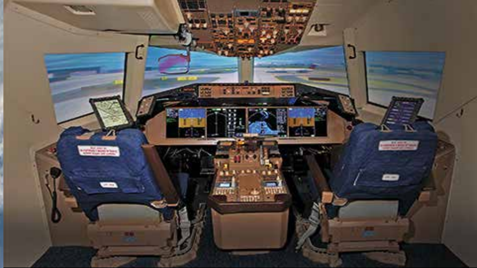
NASA has been working with Dimension Technologies Inc. on the development of a 2D/3D switchable display that could be used to help pilots better understand their position relative to other planes in the sky. This NASA flight simulator, where the display will be tested before it becomes available for use in commercial airliners, shows how the displays might be positioned.
