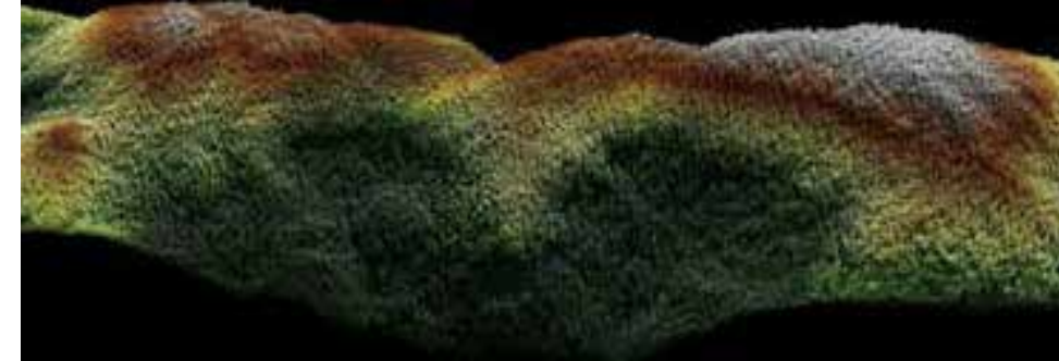
A Sigma imager captured this high-density lidar point cloud of a forested area in Sierra Nevada, California, in a single pass.
