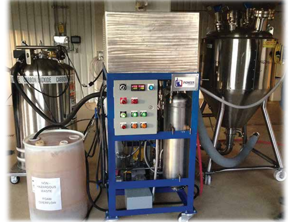
Pioneer Energy's CO 2 Craft Brewery Recovery System can recapture about five tons of carbon dioxide per month, enough for a brewery that generates up to about 60,000 barrels per year, and units can be stacked to increase that capacity.
