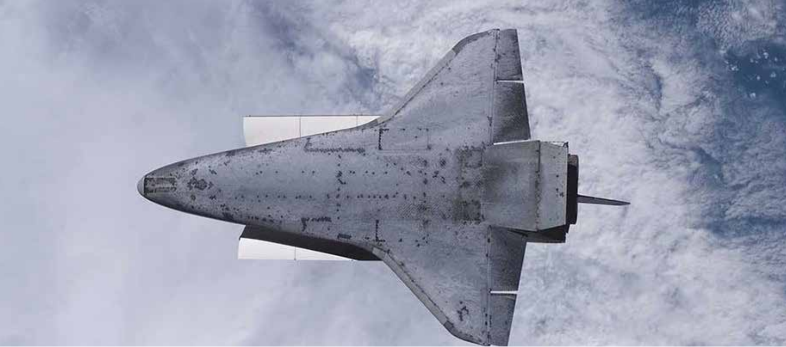
A view of the Space Shuttle Endeavour as the STS-118 crew puts the spacecraft through a rendezvous pitch maneuver, allowing the crewmembers on the nearby ISS to document the vehicle's thermal protection system condition.
