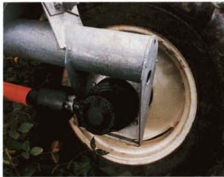
The Zimmatic irrigation system (above) consists of a series of wheeled spray towers rotating around a center pivot and watering hundreds of acres on a single swing. Electric motors drive the system through gear boxes on each wheel (left). The manufacturer improved the efficiency of the gear boxes through a redesign that incorporated NASA technology.
