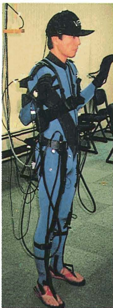
Wearing sensor-equipped DataGloves and a full-body DataSuit, a technician can virtually become part of a computer-generated environment. Sensor signals are picked up by the computer and the suit-wearer's motions, bends and gestures are replicated in the artificial environment.
