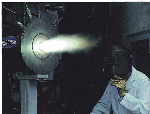
The electrically-powered plasma torch creates an ionized gas that superheats air entering the cupola to 10,000 degrees Fahrenheit. That great heat, three times higher than that attainable by oil or natural gas systems, is the key to making iron cheaper, cleaner and faster.
