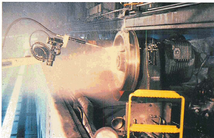
For the difficult railroad job of cleaning complex undercar equipment, Vadeko has designed a twin-robot system that automatically moves along a track beside the car and sprays a combination of water and compressed air.
