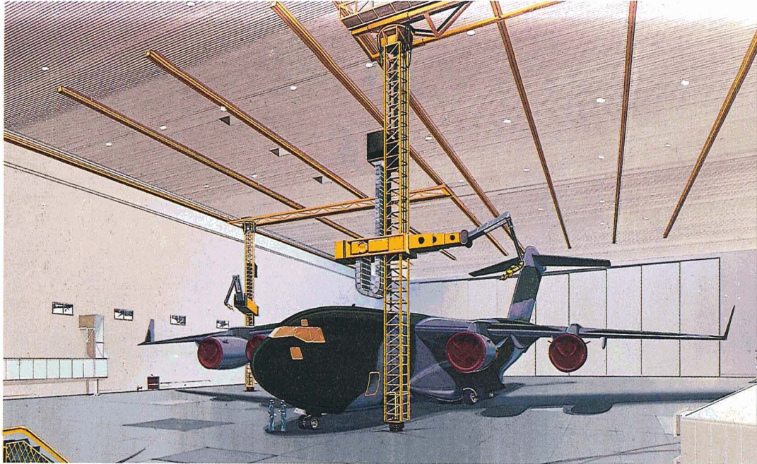
One of the largest robotic systems ever built is Vadeko's Automated Preparation and Paint Application System, designed and fabricated for McDonnell Douglas Corporation to apply all exterior coatings to large aircraft. The aircraft pictured is the C-17 military airlifter still in development.
