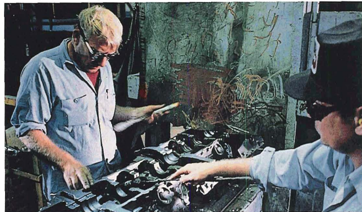
Employees at the Defiance foundry inspect castings manufactured from iron melted in the plasma melter. The Defiance plant annually produces 400,000 tons of castings for GM cars and trucks.
