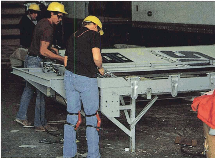
A tractor trailer frame is coated with IC 531 zinc silicate; the coating's fast cure to ceramic-like hardness allows movement of the frame directly from the coating shop to the assembly line.
