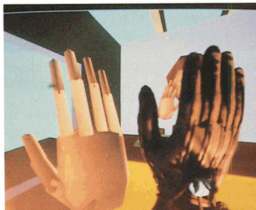
At top is the DataGlove developed for NASA by VPL Research, a computer input device for manipulating 3D environments. In the lower photo the movements of the gloved hand are duplicated on the screen by a computer-generated graphic hand.
