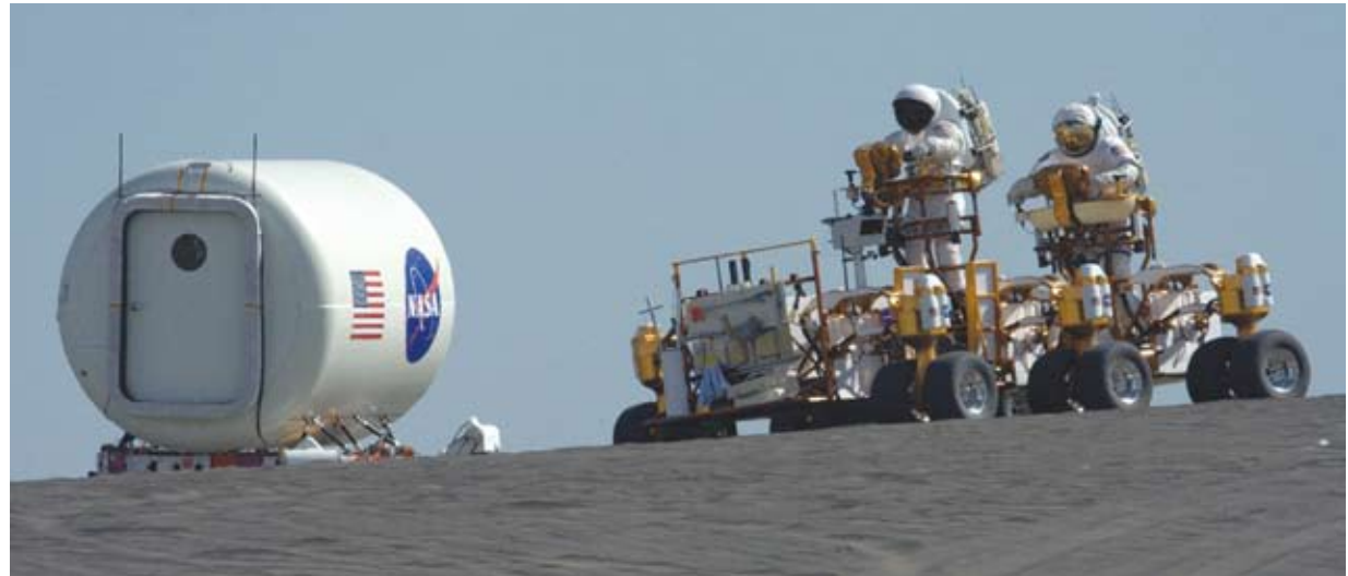
The concept for lunar rovers currently includes features such as all-direction crab steering with six wheels and a driver's perch that can pivot 360 degrees.
