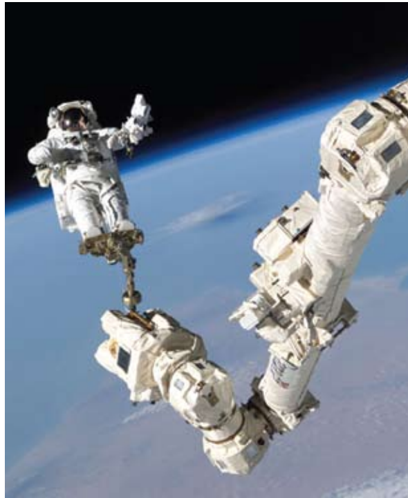
The Canadarm2 aboard the International Space Station has multiple joints and is capable of maneuvering payloads as massive as 116,000 kilograms, equivalent to a fully loaded bus. Pictured above, astronaut Stephen Robinson rides Canadarm2 during the STS-114 mission of the Space Shuttle Discovery to the ISS in August 2005.
