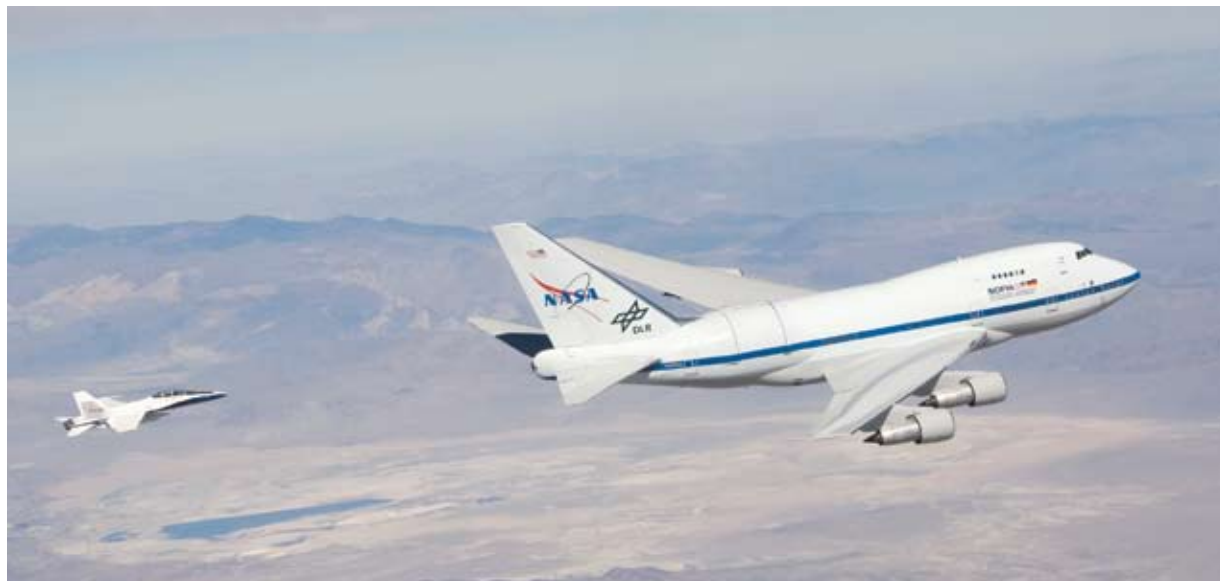
NASA's SOFIA infrared observatory and an F/A-18 safety chase during the first series of test flights to verify the flight performance of the modified Boeing 747SP.
