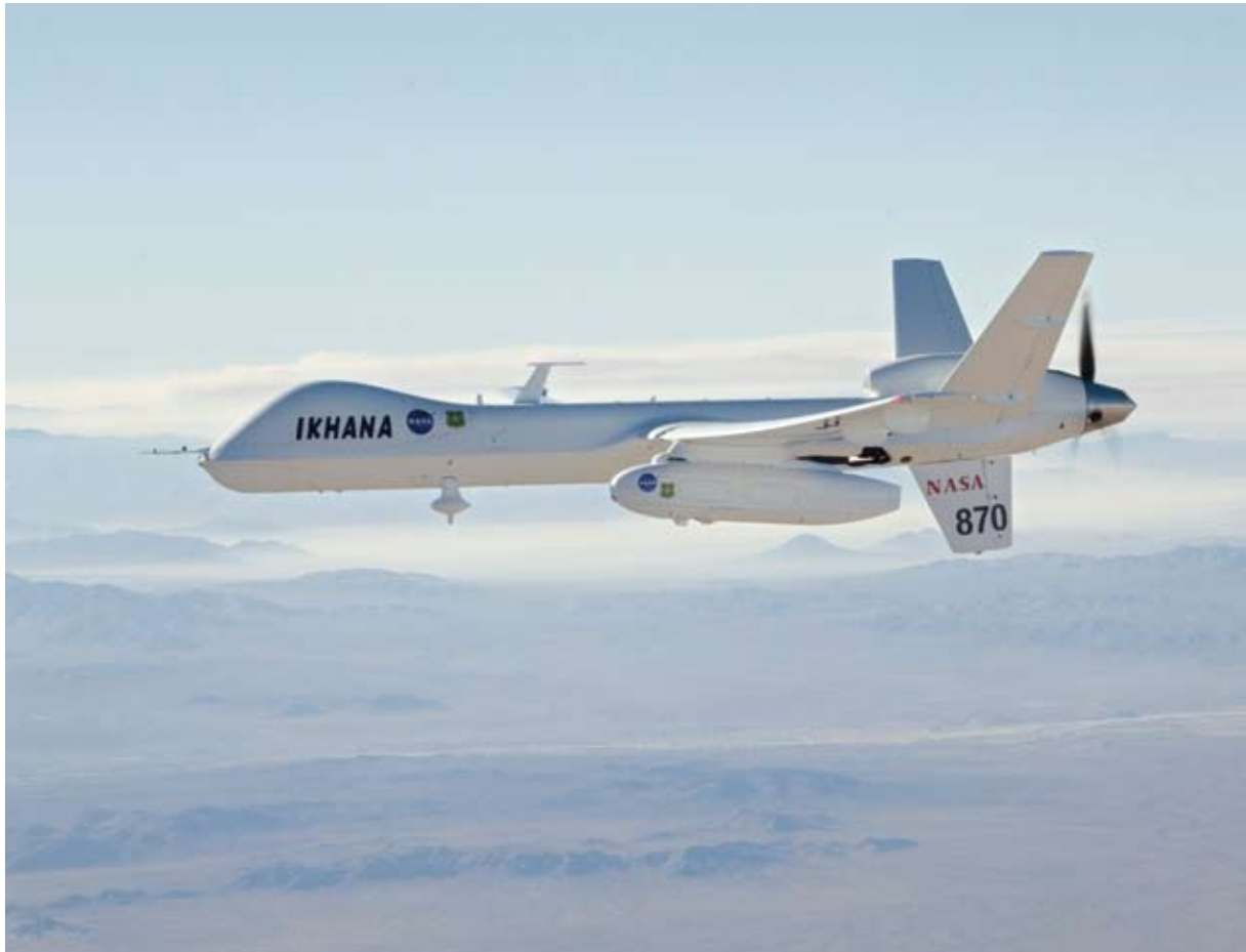
Ikhana carries the Autonomous Modular Scanner payload developed by NASA's Ames Research Center, equipment that incorporates a sophisticated imaging sensor and real-time data communications equipment. The sensor is capable of peering through thick smoke and haze to record hot spots and the progression of wildfires over a lengthy period.
