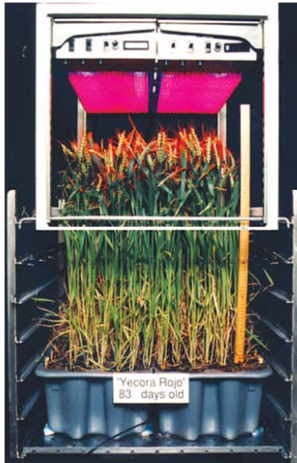
Studies have shown red LEDs are a viable light source for growing plants in space flight due to their small mass and volume, wavelength specificity, longevity, and safe operation.
