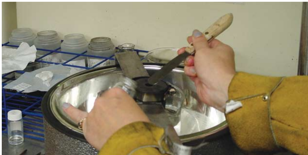
Retired Goddard Space Flight Center researcher Jeannette Benavides prepares her award-winning, low-cost process for manufacturing high-purity, single-walled carbon nanotubes. This innovative manufacturing process uses helium arc welding to vaporize a carbon rod (anode), with the nanotubes forming in the soot deposited onto a water-cooled carbon cathode.
