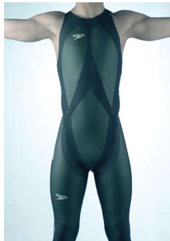
The LZR Racer reduces skin friction drag by covering more skin than traditional swimsuits. Multiple pieces of the water-resistant and extremely lightweight LZR Pulse fabric connect at ultrasonically welded seams and incorporate extremely low-profile zippers to keep viscous drag to a minimum.
