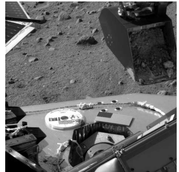
The Surface Stereo Imager captured this image on Sol 11 (June 5, 2008). The robotic arm carries a soil sample towards the partially open door of the Thermal and Evolved-Gas Analyzer's number four cell, or oven.
