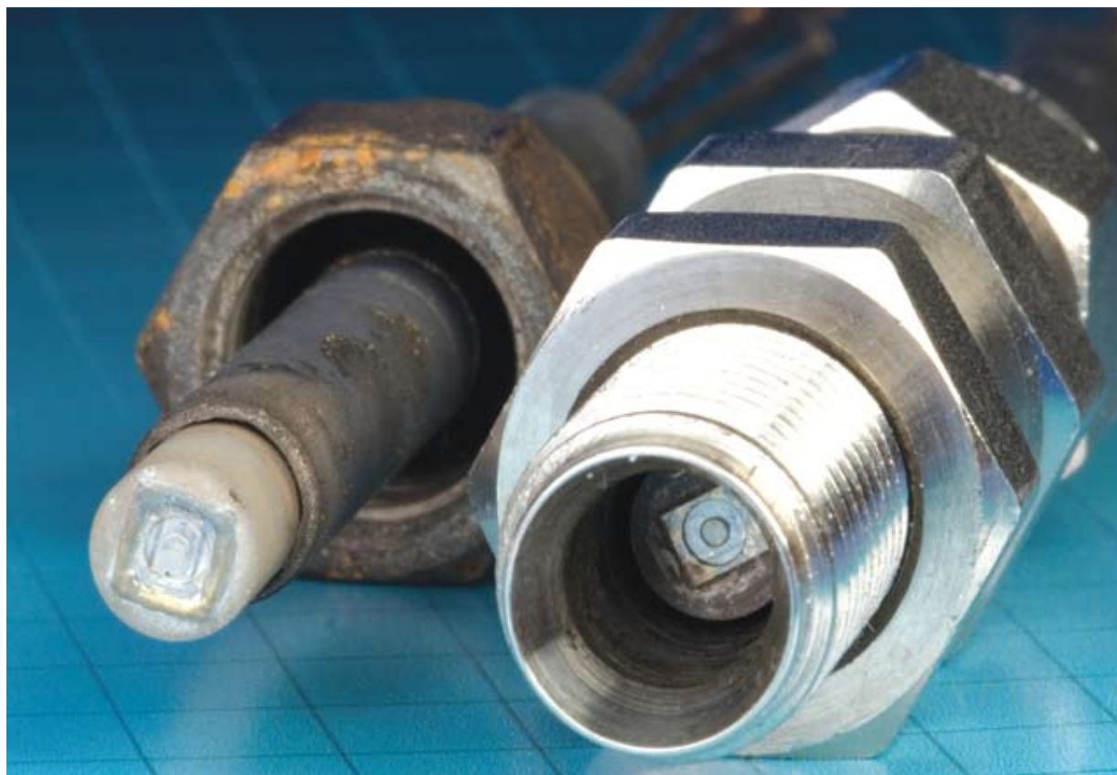
Glenn Research Center licensed three patents, covering high-temperature, harsh-environment, silicon carbide pressure sensors, to Endevco Corporation.
