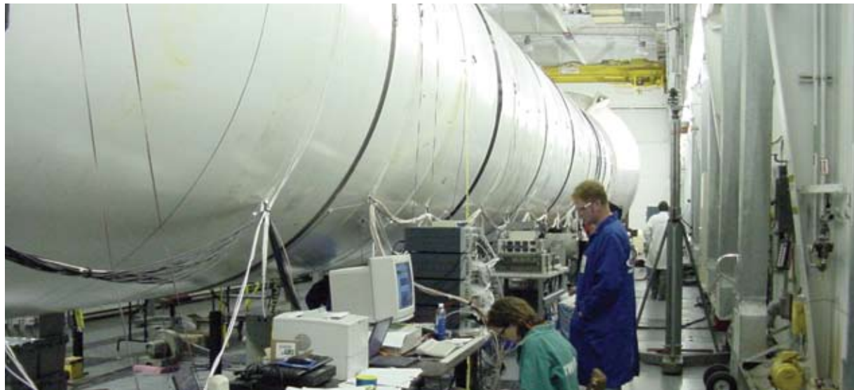
LMS software and data-acquisition hardware help test, analyze, and optimize a vehicle's ability to withstand the vibration loads experienced during missions.
