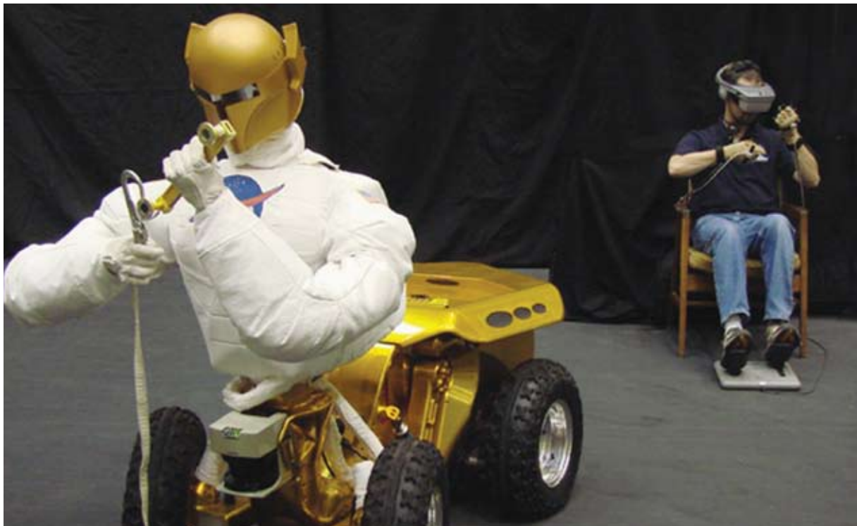
An operator in the background wears a head-mounted display that allows him to see through the Robonaut’s eyes (cameras) with a wide near-human field-of-view.
