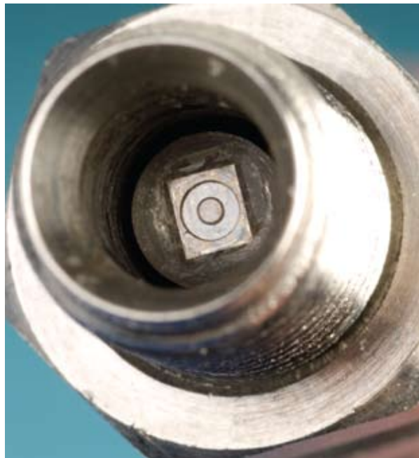
This breakthrough silicon carbide chip exceeded 5,000 hours of continuous operation at 500 °C.
