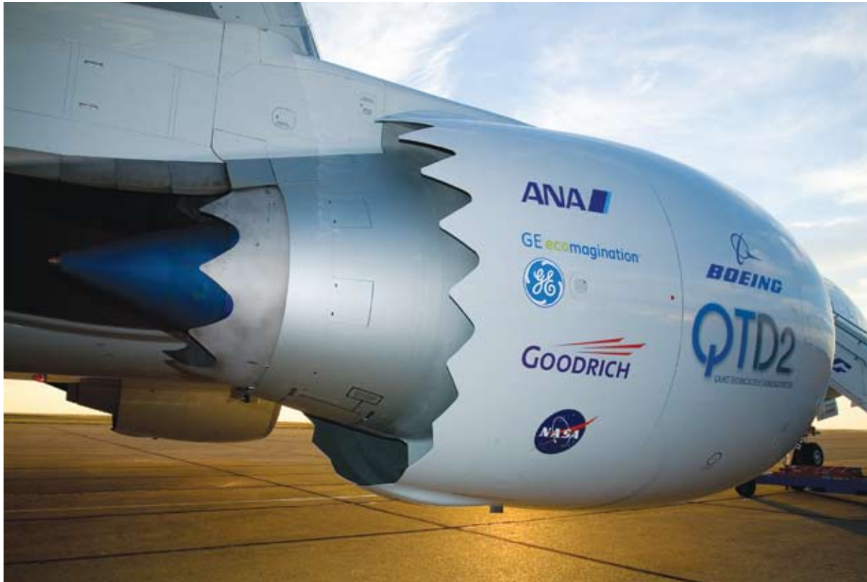
Newly developed high-temperature shape memory alloys are helping to reduce noise and improve efficiency in jet engines. NASA has sped the transfer of this technology from the laboratory to practical use worldwide.
