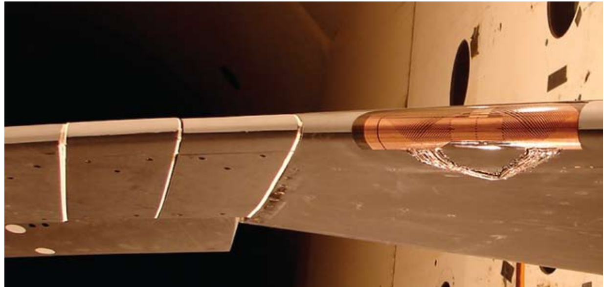
The Tao Systems sensor array, seen here on the leading edge of a Northrop Grumman SensorCraft flexible wing model, was used to successfully demonstrate gust load alleviation. Tao Systems' sensors could one day enable flexible wing aircraft that respond in real time to aerodynamic conditions, resulting in bird-like flight.
