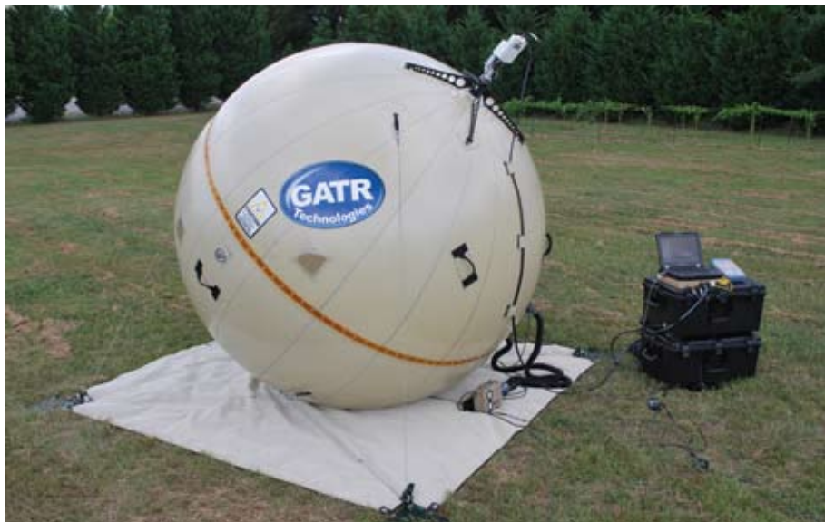
This complete satellite communication system takes about 45 minutes to set up and 15 minutes to take down. When deflated, the flexible antenna rolls up like a sleeping bag and fits in a case with the antenna bag, blower, hoses, and plates. A separate case holds the electronics, including a modem, spectrum analyzer, cables, computer, and power inverter. Each case weighs less than 90 pounds and can be checked as baggage on an airplane.
