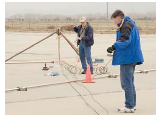
Langley Research Center's Bruce Anderson and United Technologies' David Liscinsky install tubing to connect pressure ports located on the exhaust inlet probe with sensors located in equipment trailers for the Alternative Aviation Fuel Experiment (AAFEX).
