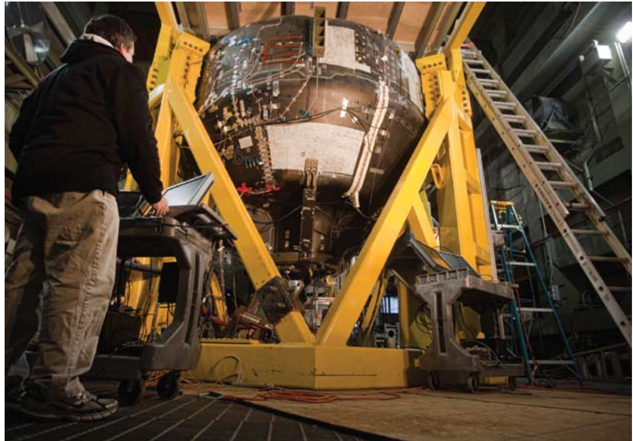
The Composite Crew Module (CCM) sits in the Test Frame in the Combined Loads Test System facility at Langley Research Center.
