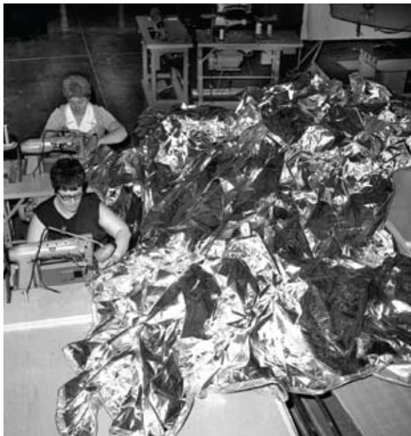
Seamstresses work on a sunshade for Skylab, which lost a thermal protection shield during its launch in 1973. The sunshade utilized a radiant barrier technology consisting of a thin plastic material coated with vaporized aluminum.
