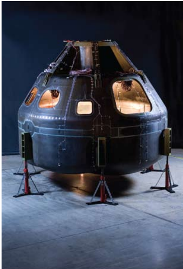
The Composite Crew Module (CCM) is a full-scale test version of the Orion spacecraft. As seen here, the CCM has fiber optic and traditional strain gauges attached.
