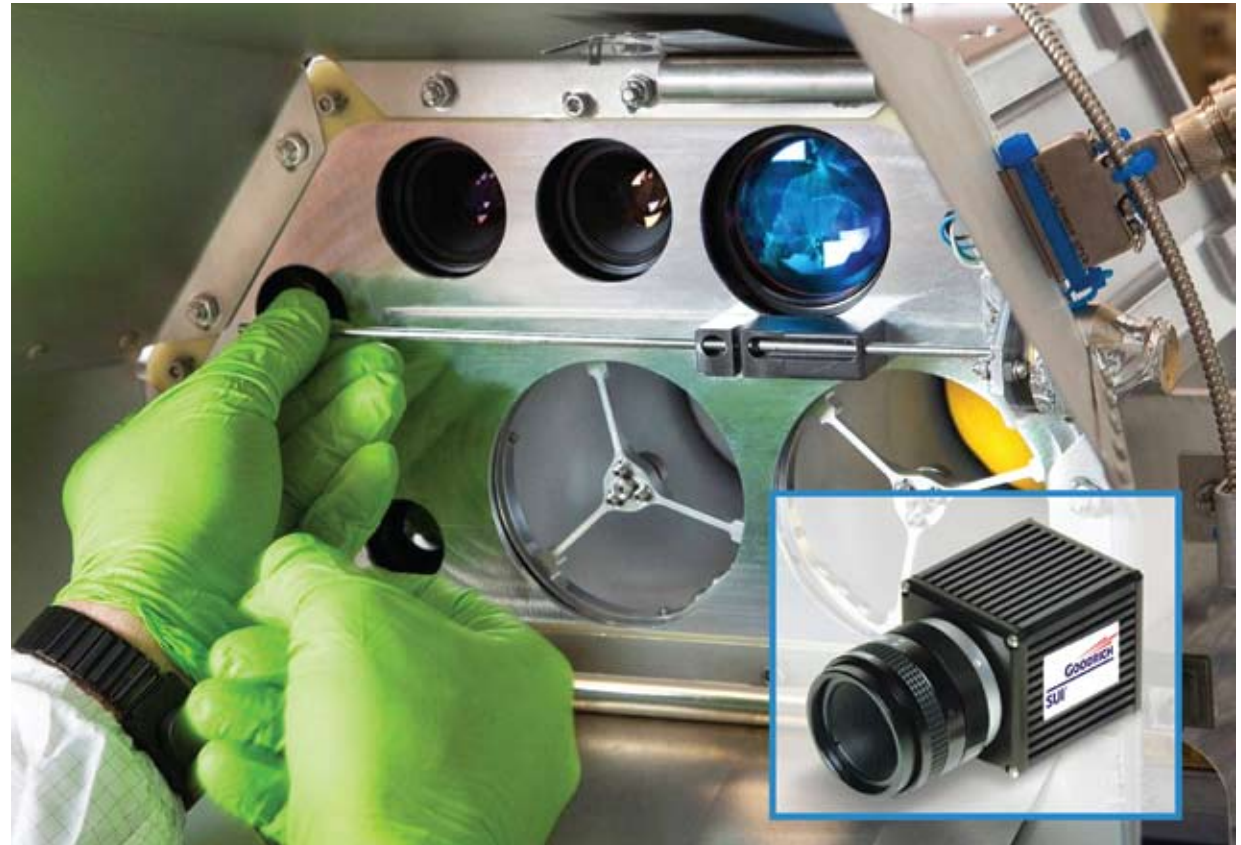
The imaging system shown here was used on NASA's Lunar Crater Observation and Sensing Satellite (LCROSS) mission. It incorporated several cameras to capture the impact of a rocket crashing into the Moon. Two of these cameras were Goodrich Corporation short wave infrared (SWIR) cameras, like the one shown in the lower right-hand corner.
