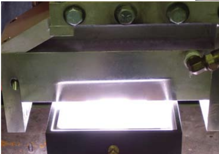
MesoCoat Inc.’s CermaClad technology uses a high-density infrared arc lamp (above) to bond the cladding material to metal surfaces, preventing corrosion for up to 100 years. While this technology extends the lifespan of infrastructure like steel beams and pipes, the company’s ZComP 844 TBC extends the life of gas turbine engine components (right) and hardly adds any cost to normal maintenance cycles.
