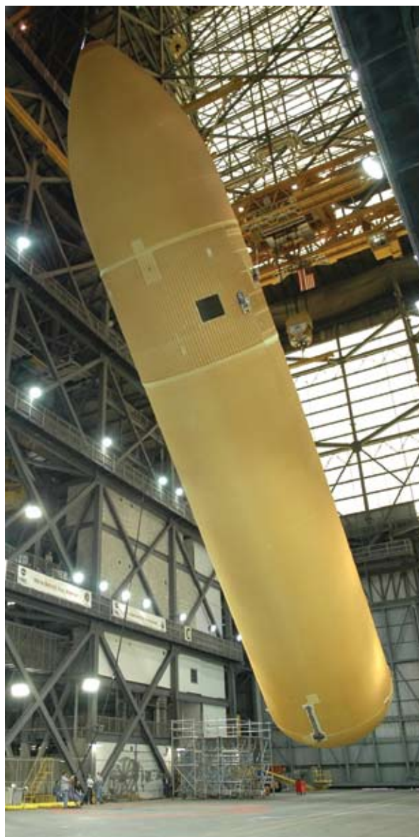
The space shuttle's external tank is coated in insulating foam that must be checked for defects. To accomplish this, NASA turned to the developing field of terahertz imaging.
