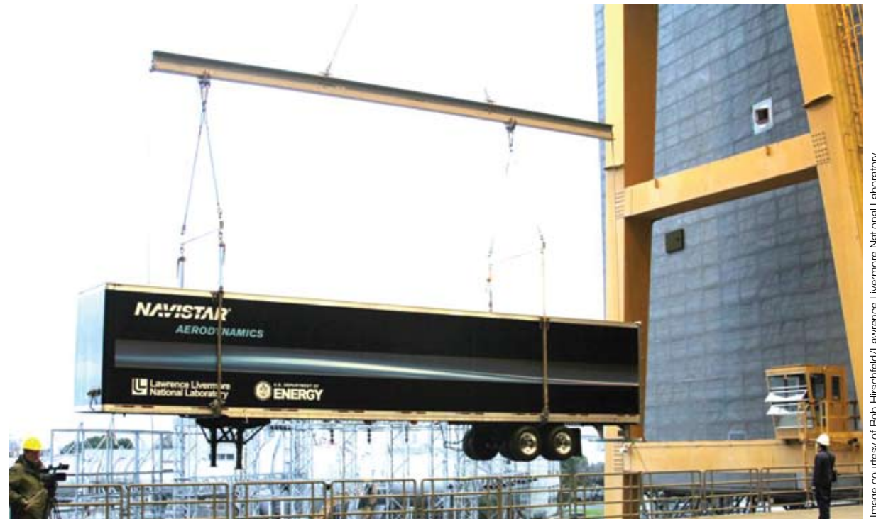
A truck trailer is prepped to be placed inside the world's largest wind tunnel, Ames Research Center's National Full-Scale Aerodynamics Complex. Testing in the facility of aerodynamic devices designed to reduce drag on tractor-trailers could ultimately result in millions of gallons of diesel fuel saved per year.
