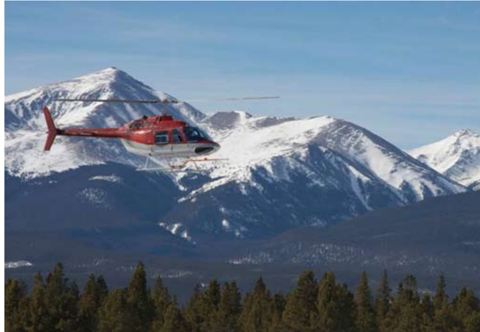
Employing the NASA-developed RC(4)-10 airfoil design, the VHA 206 rotor blade provides a high-performance aftermarket option for the popular Bell 206 series helicopter.
