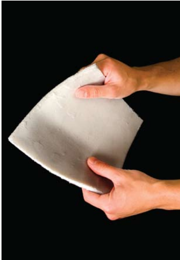
Aspen Systems Inc. worked with NASA to manufacture a more durable form of aerogel. The flexible material is made by filling the spaces of a fiber web with silica aerogel.
