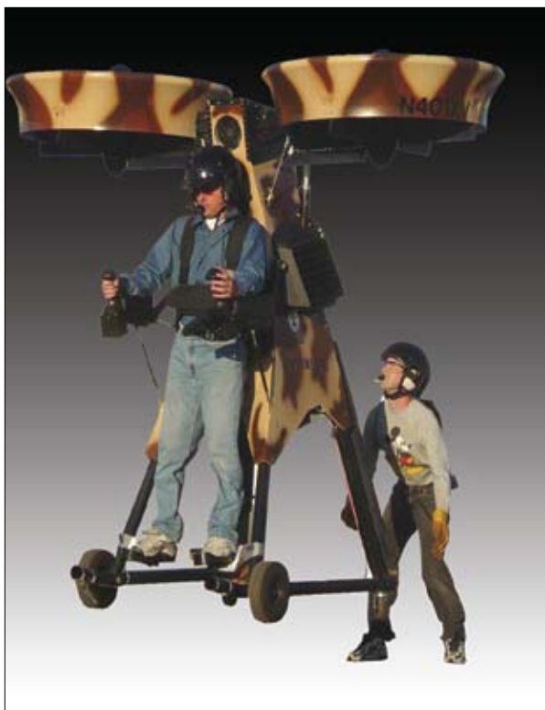
Trek Aerospace's Springtail EFV is a single operator powered-lift vehicle that supports the operator/pilot in a standing position.
