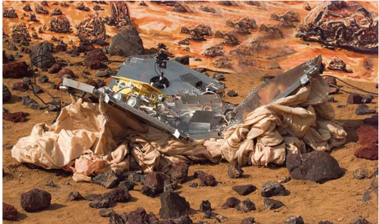
This photo, taken during Mars Pathfinder testing, shows the Pathfinder lander opening its petals to expose the yellow Sojourner rover (on left petal). Just like robotics and other hardware, control software must be extensively tested to ensure proper execution of commands.
