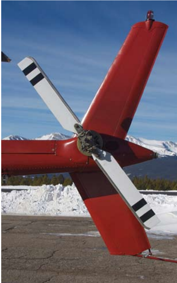
VHA's NASA-derived 206 tail rotor is made of composite material with additional features like a titanium root fitting, swept tip, nickel abrasion strip, and new pitch bearing design.
