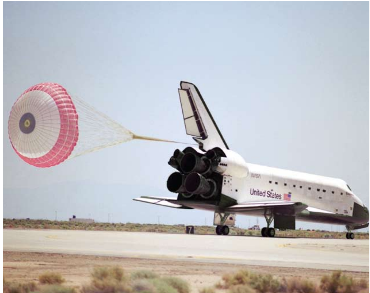
Space Shuttle Endeavour concludes a mission at Dryden Flight Research Center in 1992. The three liquid-propelled main engines, seen at the back of the vehicle, help to power the shuttle into low Earth orbit.
