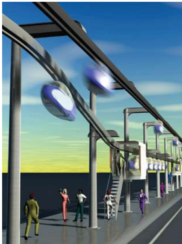
With aid from a NASA collaborative agreement, SkyTran may one day become an environmentally friendly transportation system, ferrying commuters in small, three-person pods along magnetically levitated guideways.
