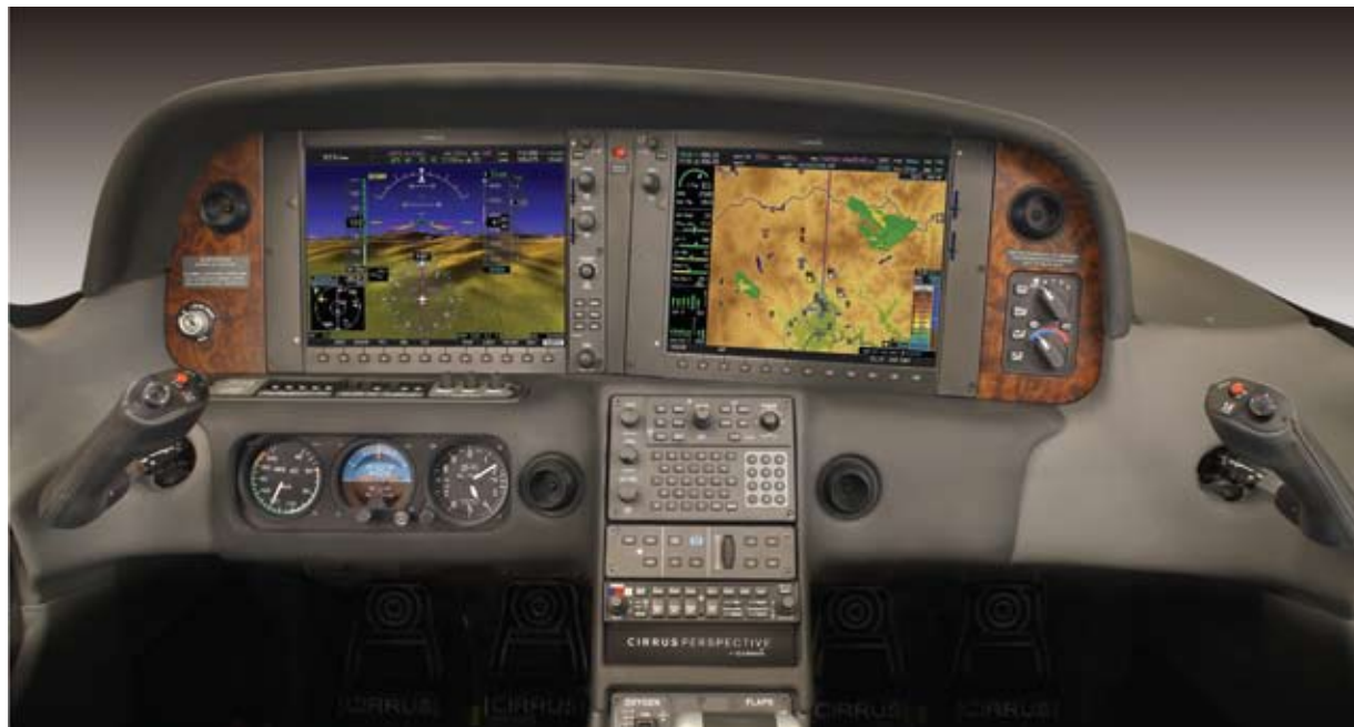
Cirrus' synthetic vision systems trace their roots to innovations in glass cockpit technology developed under the NASA-led Advanced General Aviation Transport Experiments consortium.
