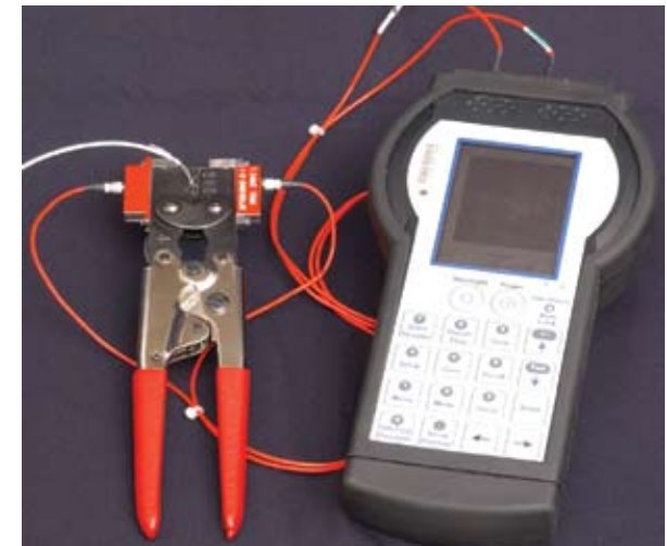
The 2009 "NASA Government Invention of the Year"—Ultrasonic Wire Crimp Inspection Technology—provides reliable testing of critical electrical connections.
