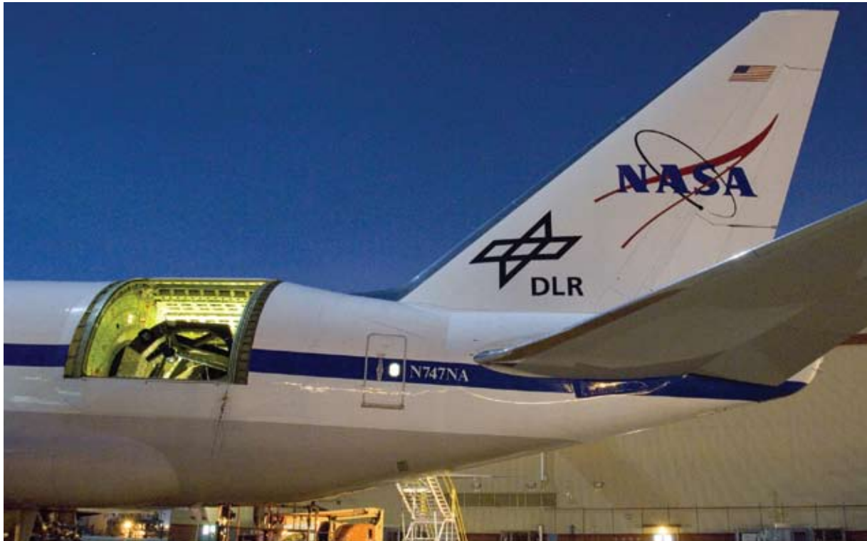
The SOFIA telescope peers out of the fuselage of its Boeing 747 mothership. The telescope will provide infrared imagery of a range of astronomical objects during flights at 40,000 feet—above the atmosphere's infrared-disrupting veil of water vapor.
