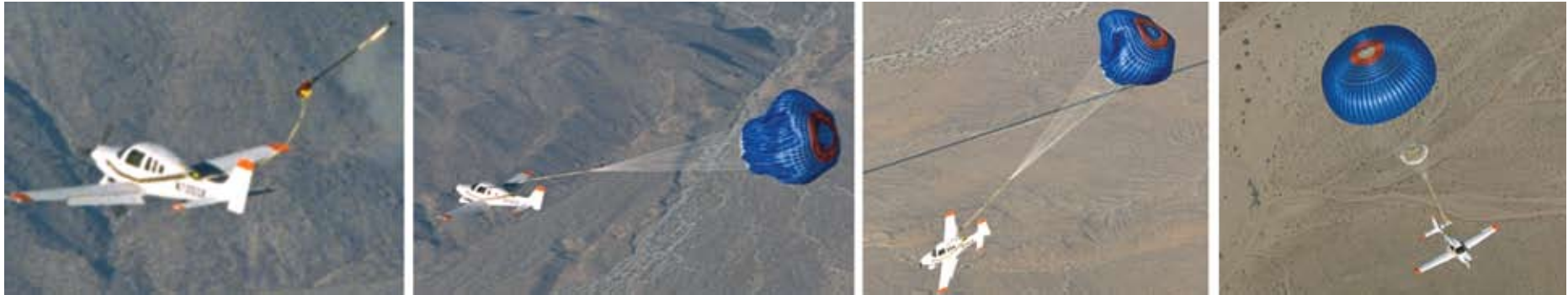
With the help of NASA funding, BRS developed parachutes that have saved hundreds of small aircraft—and their pilots and passengers. Here, a Cirrus SR20's parachute deploys at over 100 miles per hour, arresting the plane's descent. BRS parachute systems are standard equipment on Cirrus aircraft.
