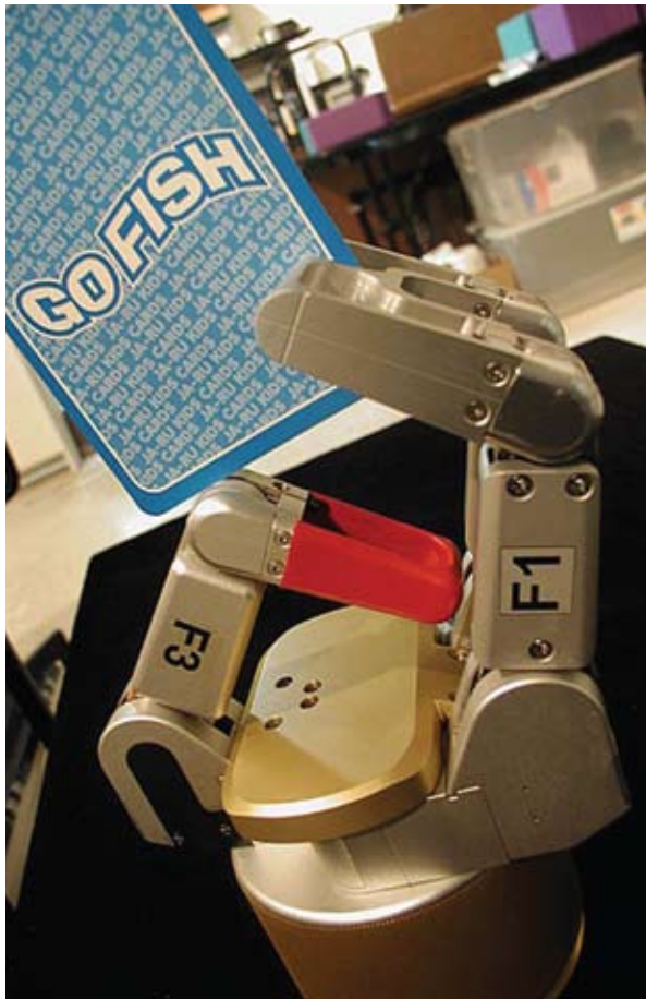
A robotic hand designed for conducting precision repairs on the ISS has found applications in surgical settings here on Earth.
