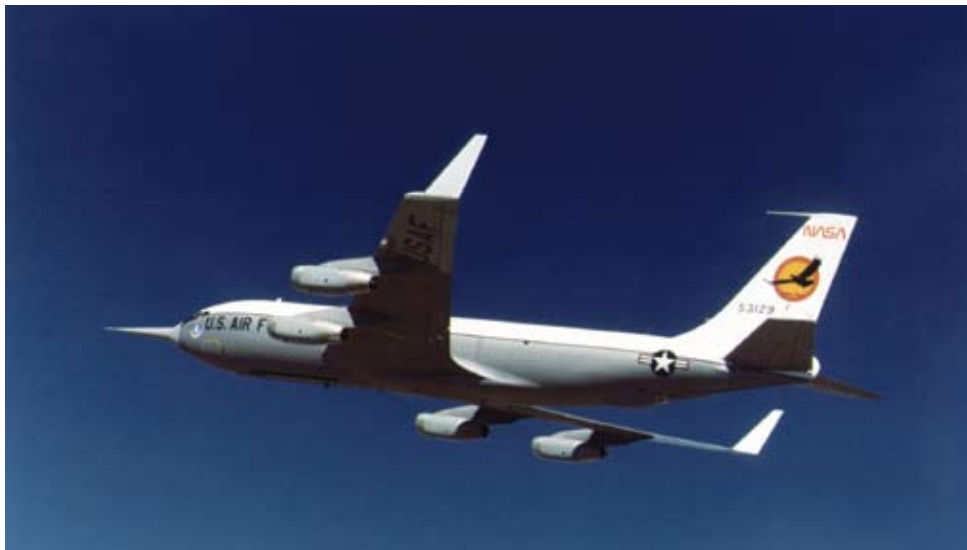
During the 1970s, the focus at Dryden Flight Research Center shifted from high-speed and high-altitude flight to incremental improvements in technology and aircraft efficiency. One manifestation of this trend occurred in the winglet flight research carried out on this KC-135 during 1979 and 1980.
