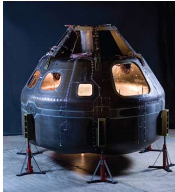
It took approximately 5 months for 50 people to fabricate the CCM, which was manufactured in 2 pieces: an upper half and a lower half.
