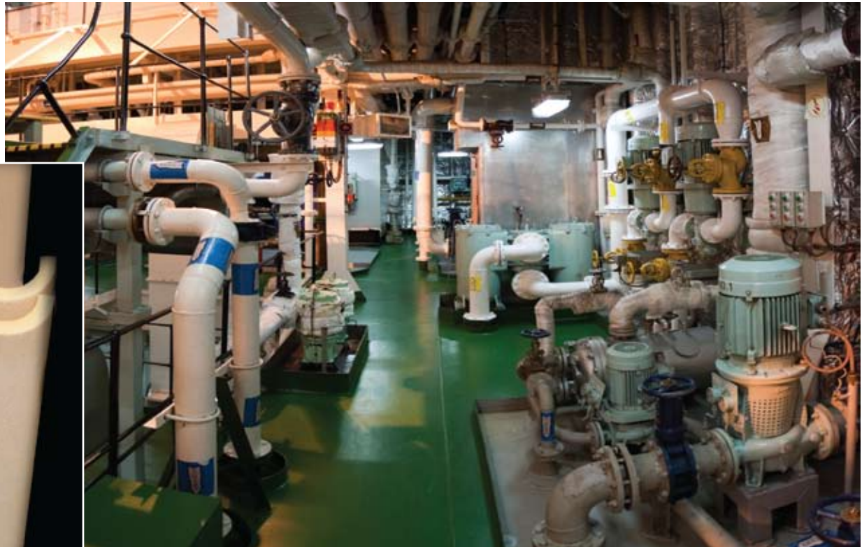
GFT’s NASA-derived foams (seen as preformed clamshells in the inset image) find significant use in engine rooms and other areas of marine vessels that require highly durable pipe insulation.
