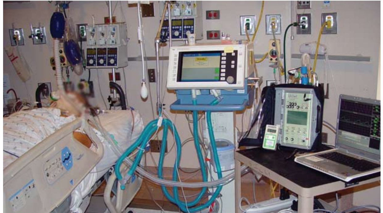
Impact Instrumentation Inc.'s 754-AP medical ventilator, on the cart and next to the laptop in the right side of the image, is tested in a clinical trial. The technology was developed through a NASA partnership.
