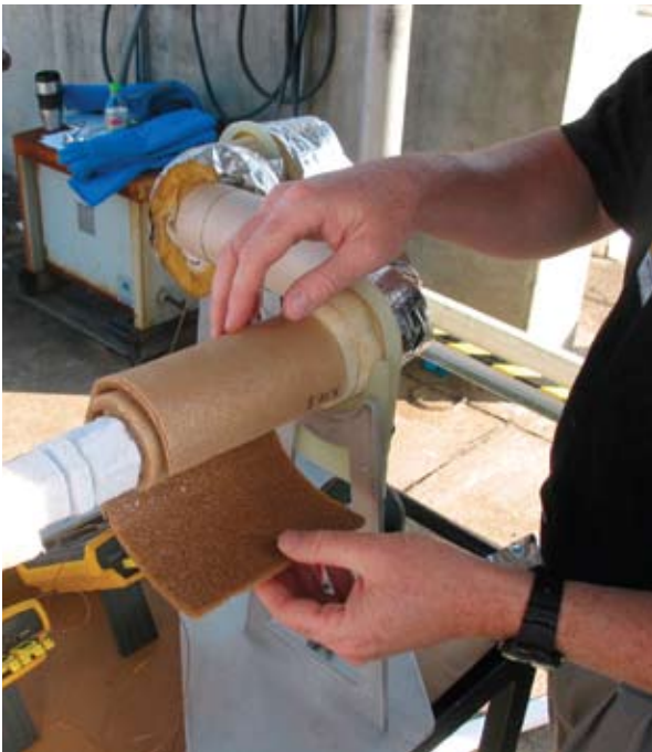
GFT LLC’s highly flexible polyimide foam—seen here during testing at Kennedy Space Center—provides an ideal insulation for pipes in cryogenic and other industrial and marine applications.
