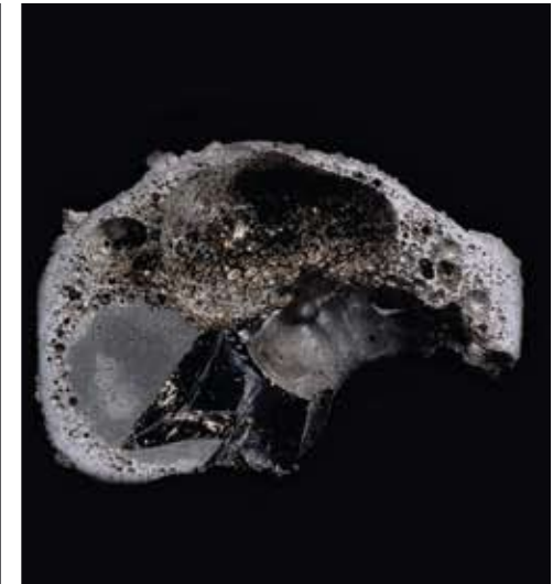
Through an SBIR with Kennedy Space Center, Ceralink Inc. demonstrated a microwave system that could heat lunar soil enough to solidify it. The images above show simulated lunar soil before, during, and after Ceralink's microwave heating. As a result of the SBIR, Ceralink refined a computer modeling program that is now offered as part of Ceralink's commercial services.
