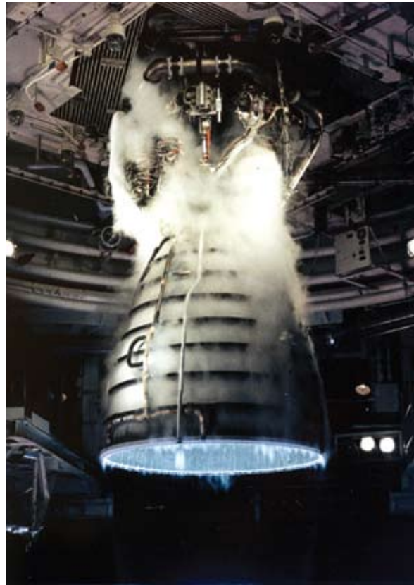
A Space Shuttle Main Engine, built by Rocketdyne under contract to NASA, undergoes test firing in 1981. Marshall Space Flight Center was responsible for the shuttle's propulsion elements, including the main engines.
