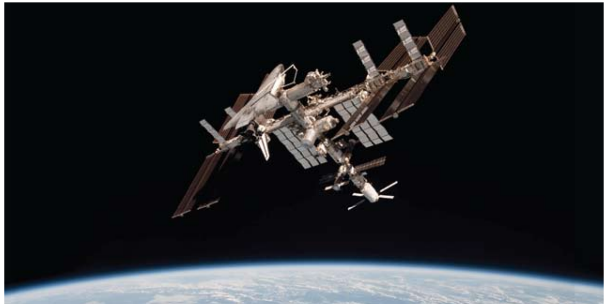
Space radiation can interfere with the electronics on the International Space Station (ISS). High-energy particles switch electronics off and can cause them to enter a hung state. Here, the ISS is shown with Space Shuttle Endeavor on May 23, 2011.
