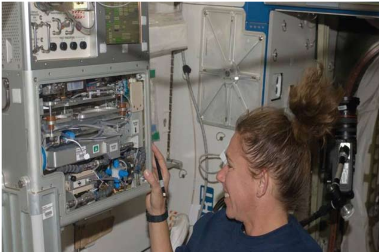
Astronaut Sandy Magnus examines the International Space Station's total organic carbon analyzer (TOCA). The technology was developed for NASA by OI Analytical and monitors the quality of the crew's water supply.
