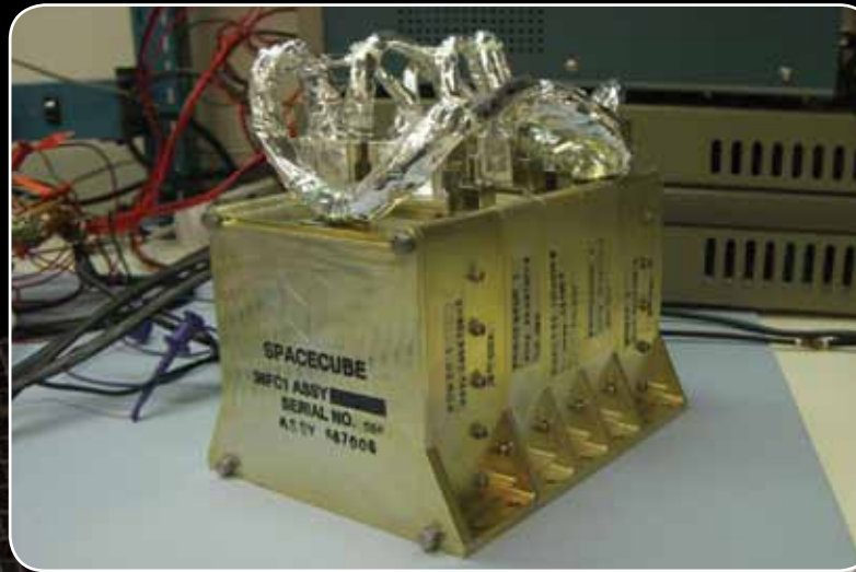
SpaceCube, pictured here, deployed on the International Space Station to test special software techniques that can make computers more immune to the problems caused by radioactive particles in space.
