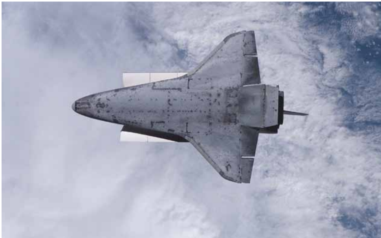
Crewmembers on the International Space Station captured this image of the Space Shuttle Endeavour while checking the condition of the shuttle’s exterior thermal protection system (TPS).
