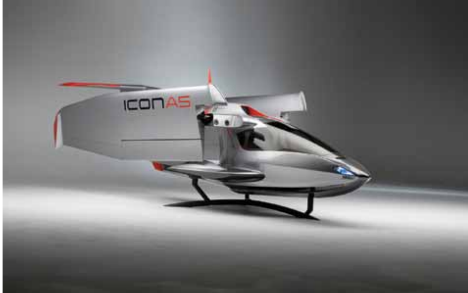
The wings of ICON Aircraft's A5 fold back so it can fit on a custom towing trailer or in a residential garage. It runs on aviation or automotive gasoline and can fly up to 120 miles per hour.
