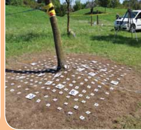
Research trees were whitewashed and black dots were applied so computer-imaging equipment could capture the stress points as the tree was pulled by a winch. Matt Melis (bottom right), an engineer at Glenn Research Center, designed the demonstration.
