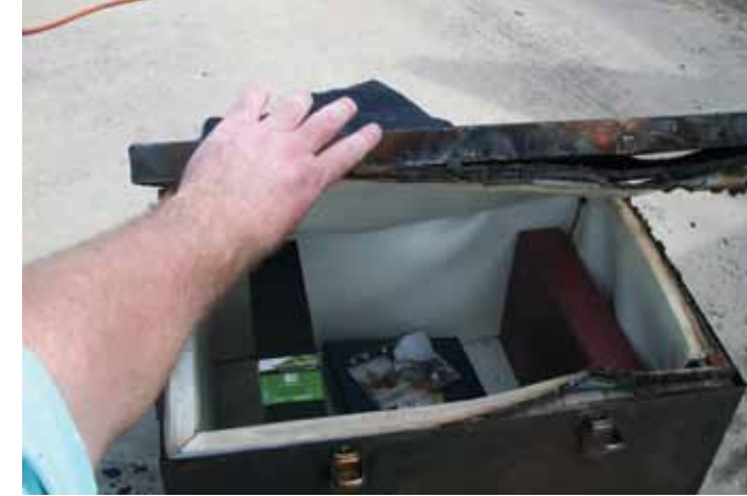
DreamSaver's Home Protection System was constructed with knowledge from a NASA astronaut and engineer who helped to develop the repair techniques for the Space Shuttles' TPS. In the images above, the box is shown before and after a 15-minute burn test at 3,400 °F.
