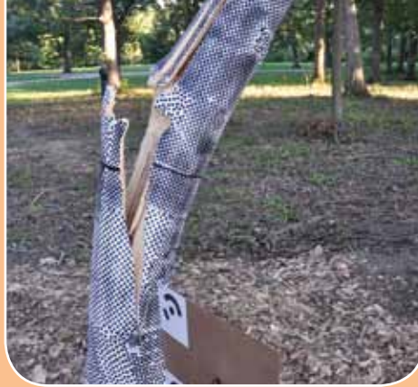
Research trees were whitewashed and black dots were applied so computer-imaging equipment could capture the stress points as the tree was pulled by a winch. Matt Melis (bottom right), an engineer at Glenn Research Center, designed the demonstration.
