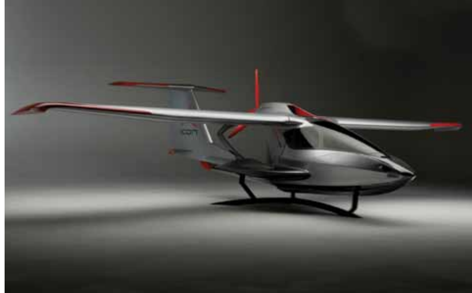
The wings of ICON Aircraft's A5 fold back so it can fit on a custom towing trailer or in a residential garage. It runs on aviation or automotive gasoline and can fly up to 120 miles per hour.
