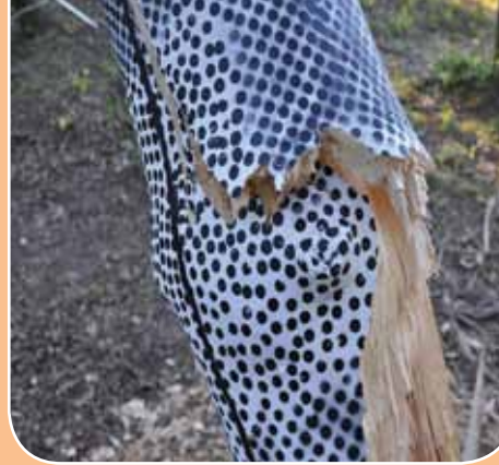
Research trees were whitewashed and black dots were applied so computer-imaging equipment could capture the stress points as the tree was pulled by a winch. Matt Melis (bottom right), an engineer at Glenn Research Center, designed the demonstration.
