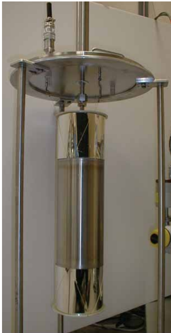
QinetiQ NA licensed the Cryostat 2, shown here, from Kennedy Space Center. Manufacturers now have an option for testing high-performance insulation materials in relevant conditions on-site at their production or lab facilities.
