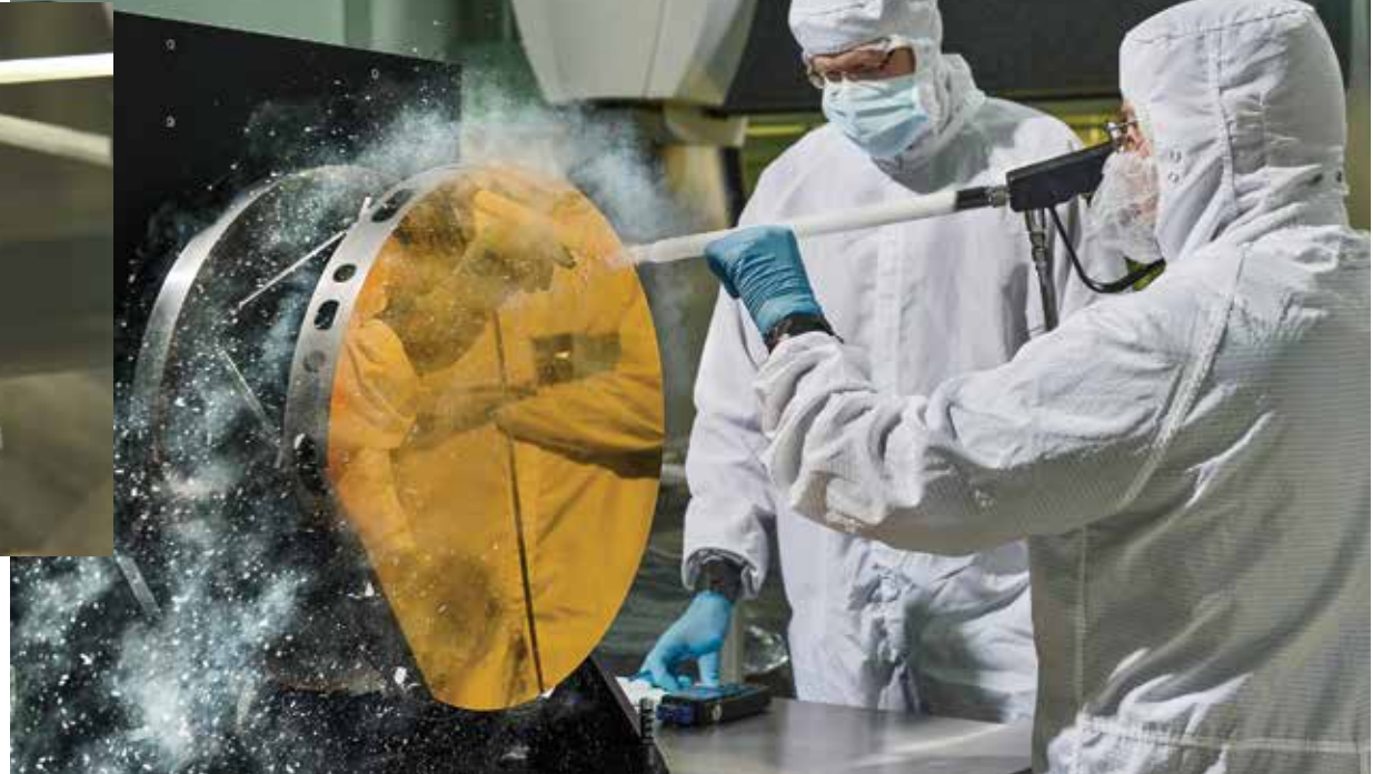
Engineers at Goddard Space Flight Center use carbon dioxide “snow” to clean a test mirror for the James Webb Space Telescope. Because they’re cold, components like mirrors and lenses, which have to be completely clean and flawless in space imagers, are among the first places any volatile compounds outgassed from a spacecraft’s materials will condense, causing fogging. To prevent this, all materials used in spacecraft have to demonstrate extremely low outgassing.
