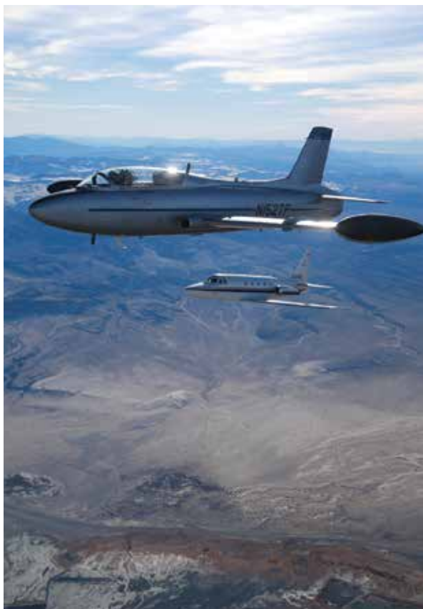
Two planes from IFTI’s fleet fly over the Mojave Desert, where the institute is located. Top is a MB-326 Impala used for high acceleration and unusual attitude flight, and below is a Rockwell Sabreliner, used for the zero-gravity experiences that are part of the organization’s spaceflight curriculum.
