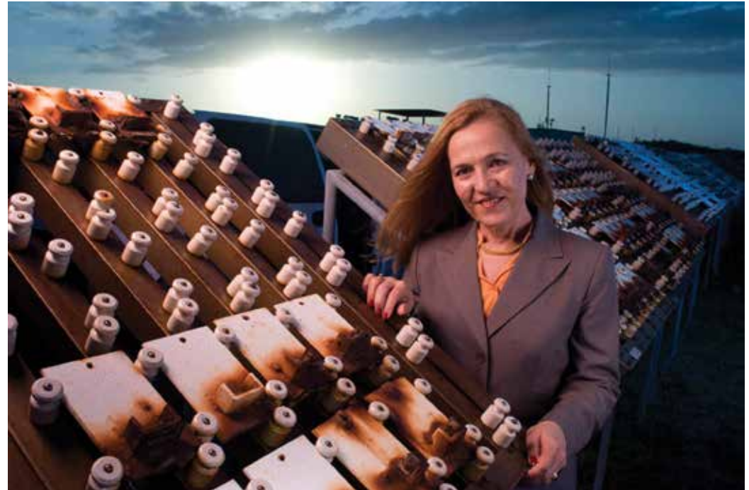
Luz Calle, the technical lead for Kennedy Space Center's Corrosion Technology Laboratory, checks out sample tiles at the Kennedy's Beachside Corrosion Test Facility.
