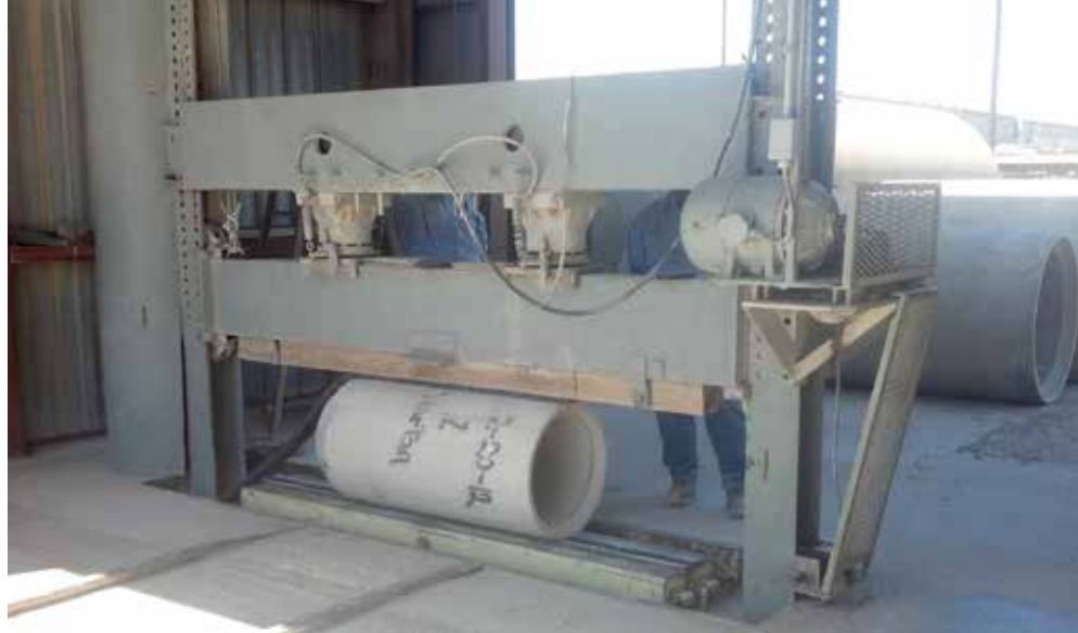
After the successful Stennis tests, the Louisiana Tech team founded Alchemy Geopolymer Solutions, leveraging their expertise in designing concrete made with fly ash. A pipe-maker in Texas was interested because of the material's high resistance to corrosion and its impressive compression strength.
