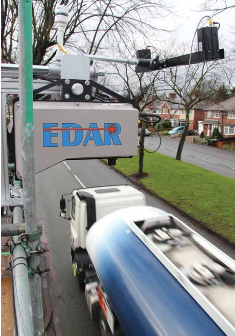
Hager Environmental and Atmospheric Technologies' Emissions Detection and Reporting (EDAR) system has been purchased and installed by four states for various programs related to validating vehicle emissions compliance. In the future, EDAR could make drive-in emissions tests obsolete, replacing them with remote, laser-based sensors that can scan cars and trucks as they pass underneath.
