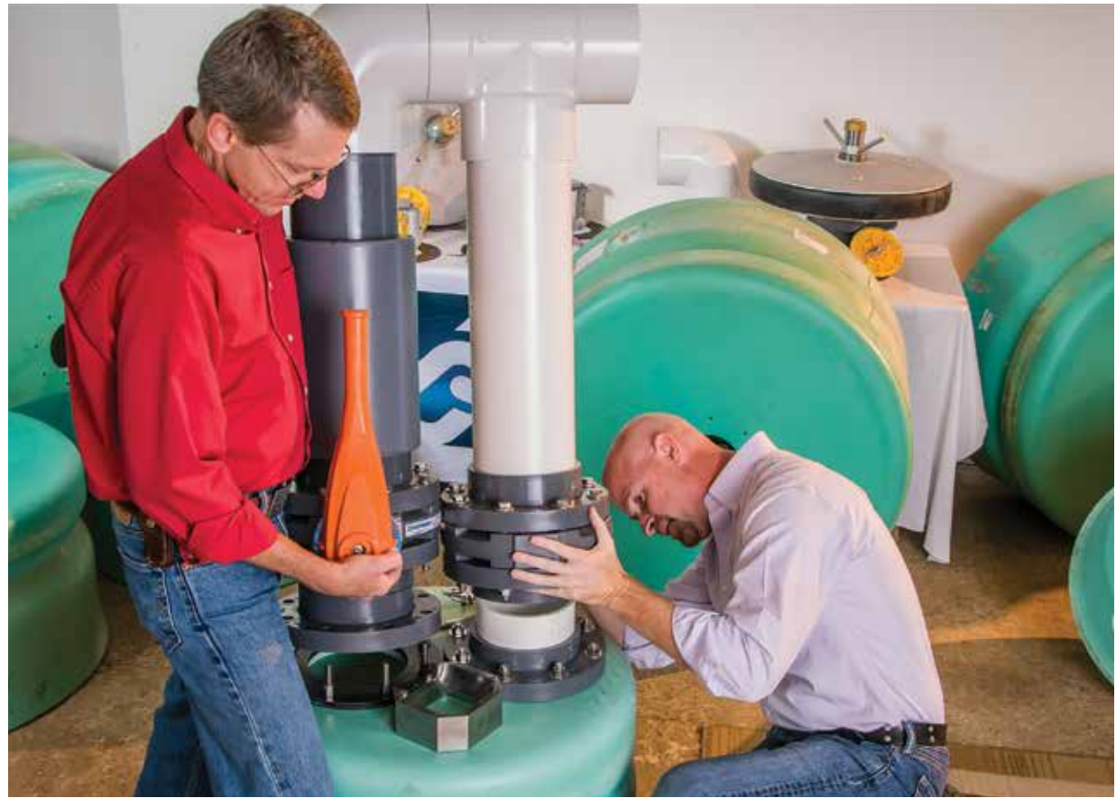
Engineers Rob Berry and Jeff Lindner work on pipes that will contain the disruptive tuned mass device they first helped create for the Ares 1 program. Now they are adapting it for future NASA use and for commercial use, such as in buildings, bridges, or oil rigs.
