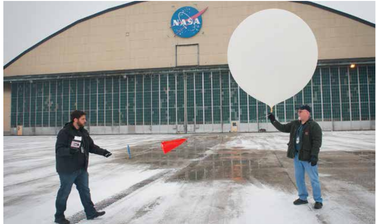
Glenn Research Center icing expert Michael King (left) prepares to launch a weather balloon equipped with a supercooled liquid water sensor designed by Anasphere Inc. Results from balloon launches such as this one will help verify whether a ground-based NASA system can effectively predict icing conditions aloft.
