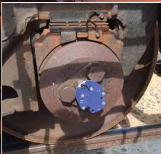
Ridgetop Group's RailSafe sensor fits on the ends of a train's axles, where it monitors for vibrations caused when the wheels roll over anomalies in the rails.
