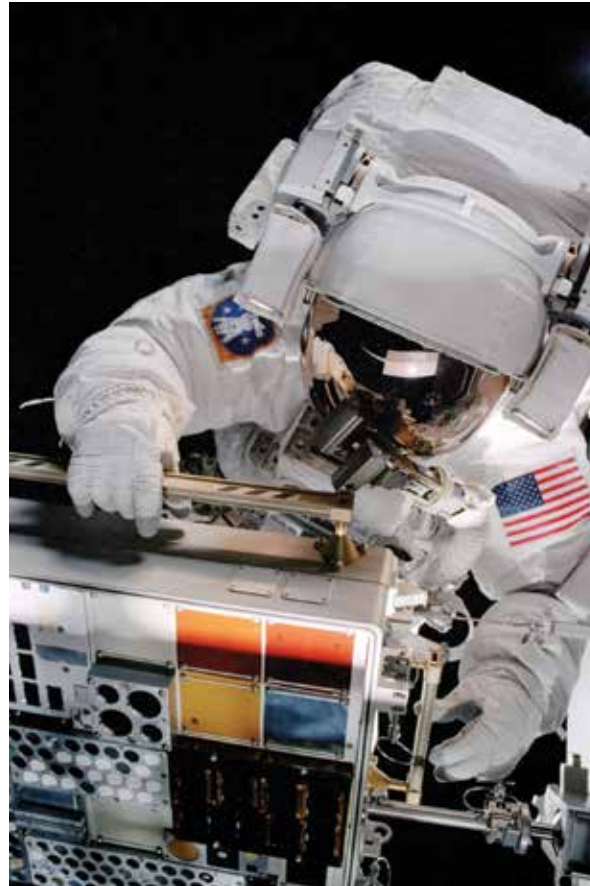
An astronaut installs a Materials International Space Station Experiment (MISSE) facility on the exterior of the ISS during a spacewalk in 2001. Future iterations of MISSE, handled by Alpha Space, will be installed and maintained via robotic arm, eliminating reliance on spacewalks.
