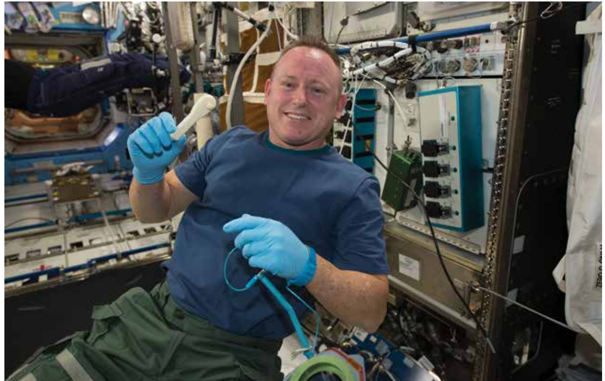
In 2014, astronauts printed a functional ratchet on the ISS from a design created on Earth and emailed into space. NASA is interested in developing 3D technology to help supply long-duration missions with items the crew didn't, or couldn't, bring with them.
