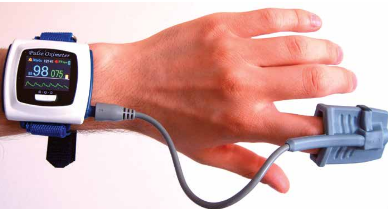
One of the many medical uses for TracePro is validating designs for blood oximeter pulse monitors. The monitors measure oxygen in the blood by observing how light travels through the fingertip.
