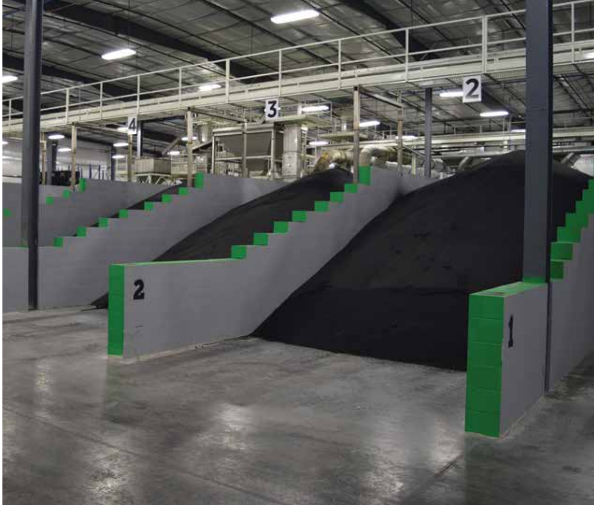
Here, large batches of the Florikan fertilizers await quality control testing before being bagged up and sold. The high-tech process to coat the fertilizer in a porous polymer to control how quickly the nutrients dissolve in water was perfected with help from NASA.
