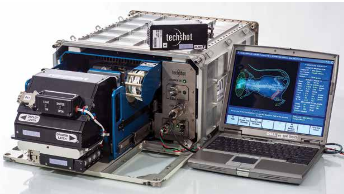
Techshot worked with NASA and the Center for the Advancement of Science in Space to develop a commercial bone densitometer suitable for operation on the ISS. The device, dubbed Bone D, is primarily used by companies to study the effects of microgravity on mice.
