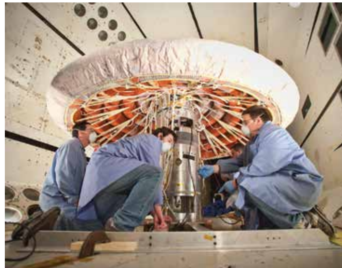
Engineers examine an inflated heat shield after it was tested in a vacuum at NASA's Langley Research Center. These Hypersonic Inflatable Aerodynamic Decelerators, or HIADs, may prove more economical and efficient for carrying heavy loads to planets with an atmosphere.
