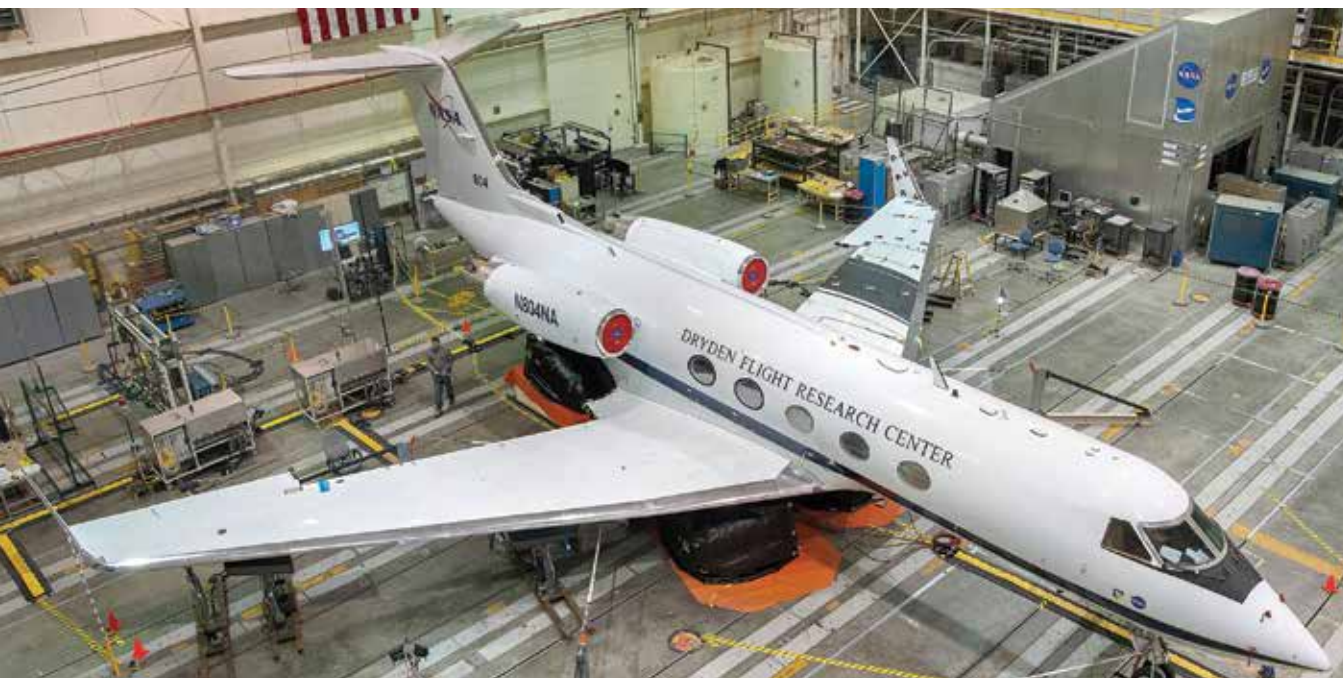
The Flight Loads Laboratory at Armstrong Flight Research Center (formerly Dryden Flight Research Center) tests the strength and endurance of aircraft structures, using hydraulic actuators to apply forces that simulate the stresses of takeoff, flight, and landing. The testing involves many cables, hoses, and wires, which the lab minimized by requesting a fleet of hydraulic carts that can be parked near the aircraft and connect to a front-end computer with just two wires. Two of the carts can be seen to the left rear of the plane above.
