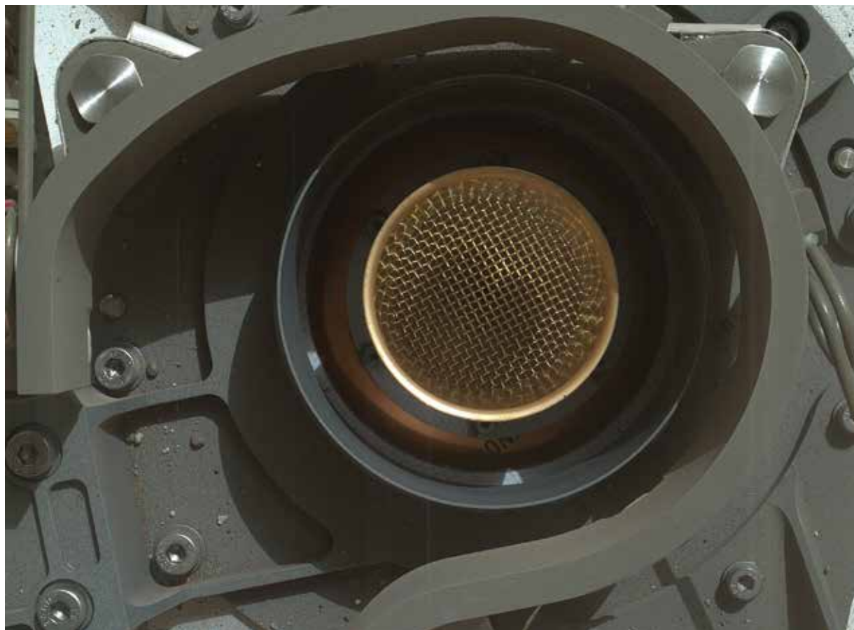
The key innovation of CheMin was that it didn't require samples to be finely ground into powder. In fact, the rock grains need only to be small enough to fit through this screen installed on Curiosity, through which the Mars rover funnels the samples it collects with its robotic arms.
