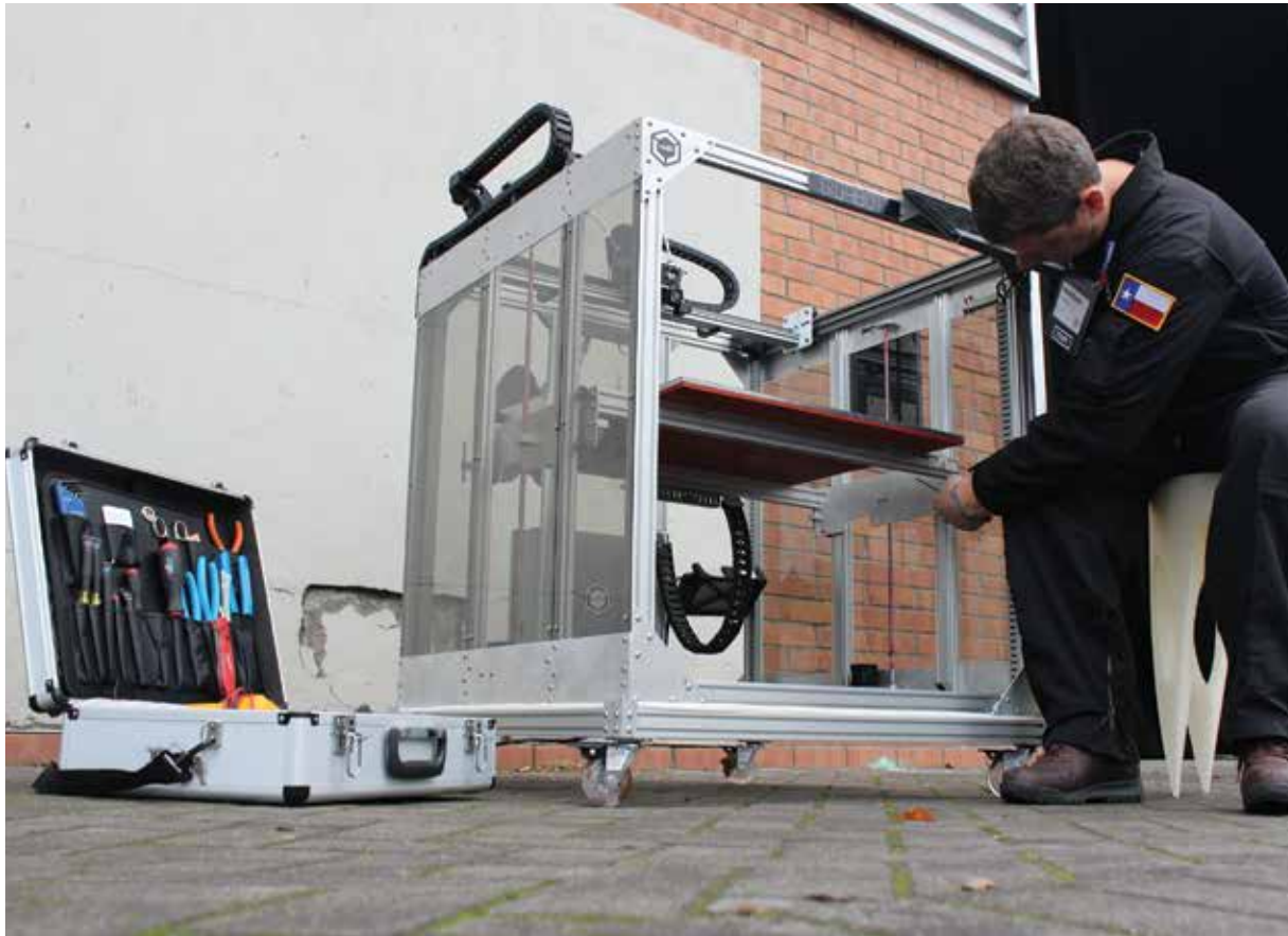
The founders of re:3D drew on experience at Johnson Space Center to design and sell a large-scale 3D printer at a low cost. The standard configuration prints items up to eight cubic feet, or 30 times larger than competing desktop models.
