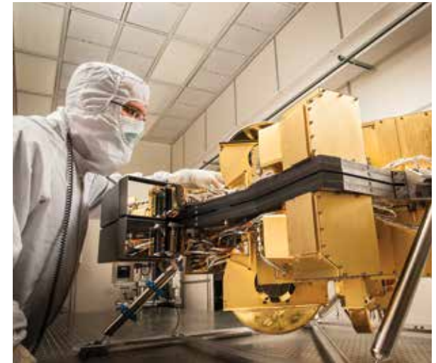
Materion Precision Optics developed a whole new lens-coating process to produce the unprecedented uniformity and wavelength positioning required for the James Webb Space Telescope's Near Infrared Camera, pictured here. It's a process the company now uses to create standard products on a daily basis.
