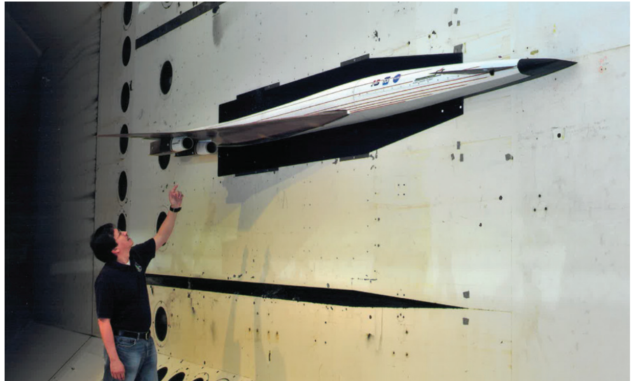
Aeroelasticity engineer Walt Silva examines an aircraft model undergoing testing in the Transonic Dynamics Tunnel at Langley Research Center. Silva created innovative software that speeds up computational modeling of aircraft to reduce the need for costly wind tunnel tests.
