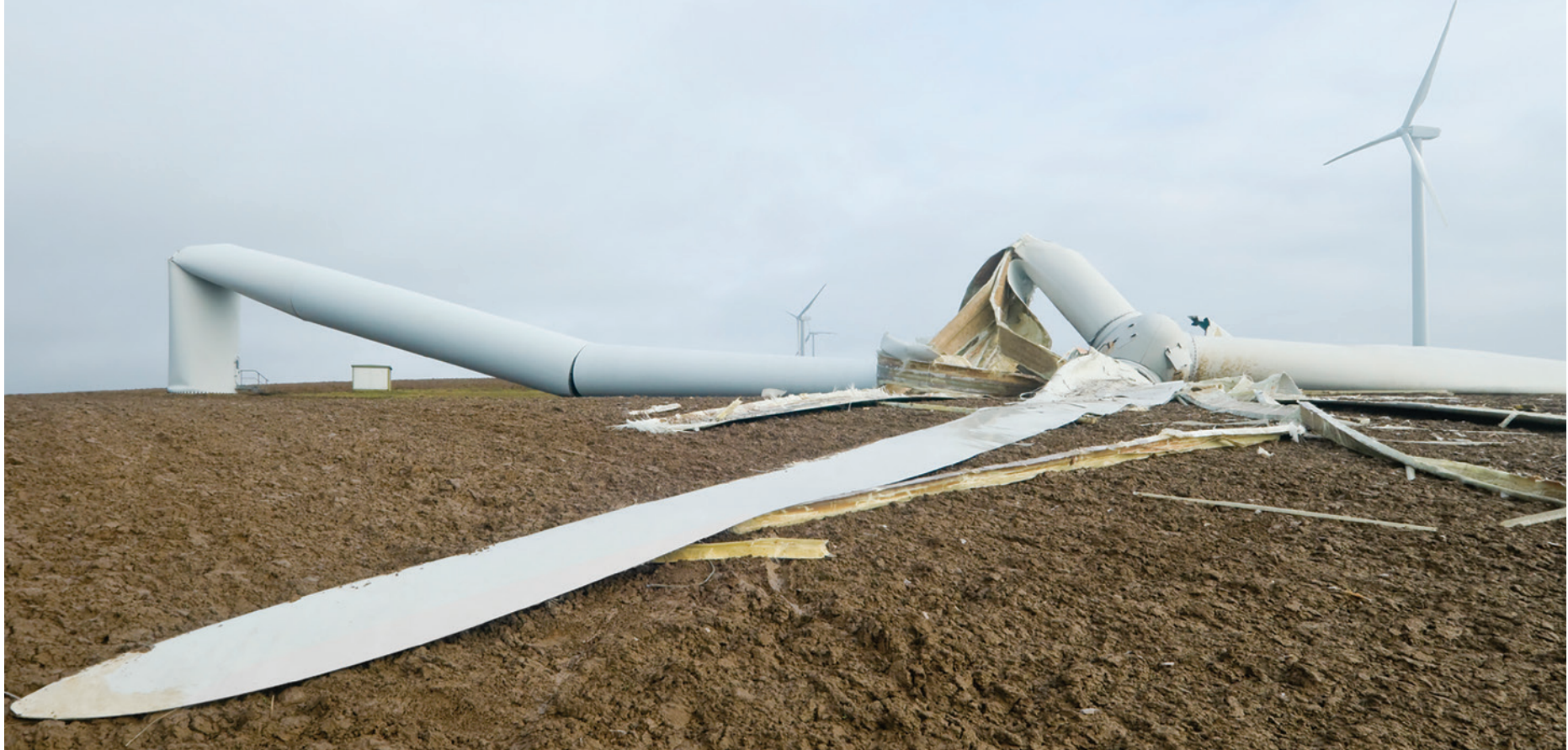
One application for the Optical Jupiter lightning detection system is on wind farms. Amid acres of turbines, it can be hard to pinpoint where damage occurred, but if you are able to identify which one was struck, you can shut it down before it catastrophically fails.
