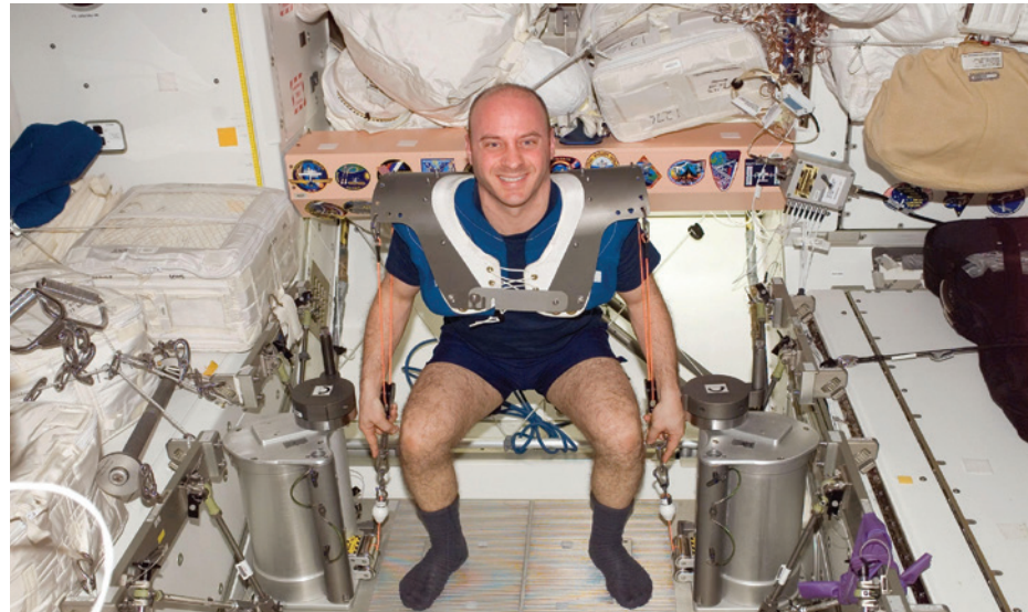
In zero gravity, the human body quickly loses significant muscle and bone mass, making a rigorous workout schedule crucial to long-term health. OYO Fitness founder Paul Francis worked with NASA to develop a resistive exercise device suitable for use on the space station, pictured here in use by NASA astronaut Garrett Reisman. The innovation led to several lines of Earth-bound exercise devices, most recently OYO Fitness’ DoubleFlex Silver portable gym.
