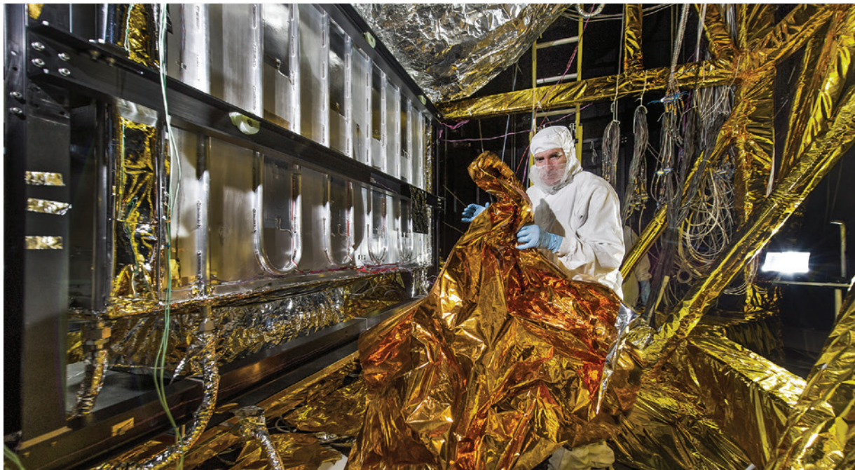
In Goddard Space Flight Center’s Space Environment Simulator, an engineer lays radiant barrier insulation over wires on the floor, keeping the heat they generate from contaminating the chamber, which is used to mimic the environmental conditions of space.
