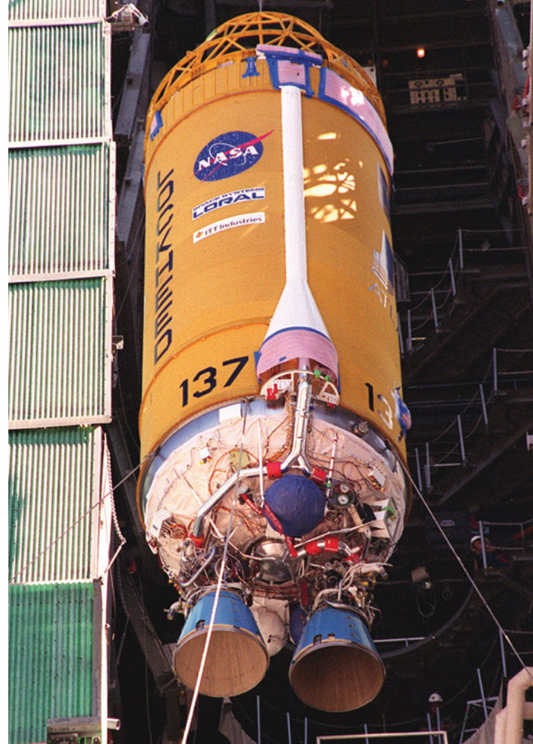
The Centaur upper-stage rocket, always powered by one or two RL10 engines, remains the country's most-used upper stage more than half a century after its first flight.
