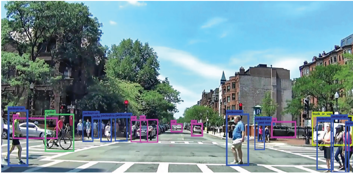
This screenshot shows a self-driving car's view when powered by Neurala's software. The vehicle can automatically identify pedestrians, cars, cyclists, trucks, and more on a Boston street in real time.
