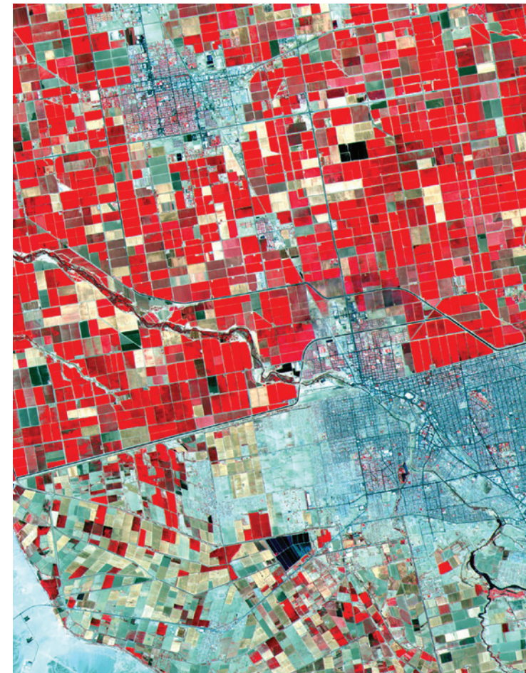
This image of the U.S.-Mexico border from 2000, combining visible and infrared bands, shows lushly growing, gridded fields (in red) on the U.S. side, compared to more sparse and irregular growth in Mexico. Tunable liquid crystal filters help focus in on different light wavelengths, which can reveal insights like which plants need more water or which might be diseased.
