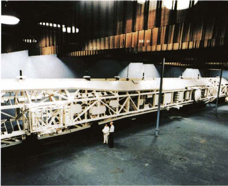
At left, Space Station Freedom is shown in its Permanently Manned Capability (PMC) Configuration. Initial PMC is targeted for year 2000. Shown above is a mockup of the central truss assembly, which will be built and launched in sections and joined in orbit to provide the structural framework that stiffens and stabilizes the station.
