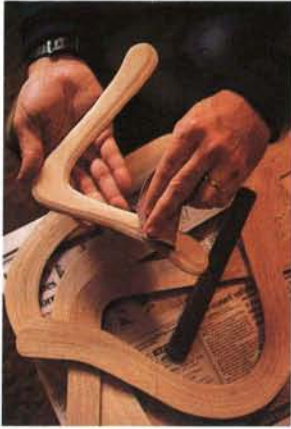
Ted Bailey's trendsetting designs, based on NASA technology, are very popular in the U.S. and abroad. Bailey's booms are handcrafted from Finnish birch plywood, filed and drum-sanded to a predetermined aerodynamic shape, then hand-sanded and finished.
