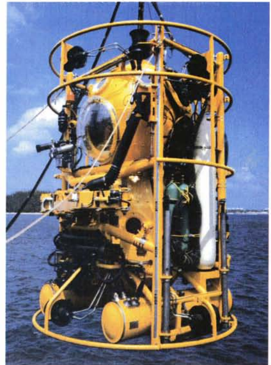
At left is a Videospection Model 2531-A Color Camera in a military fighter installation and below is a Videospection underwater camera used aboard the Perry oceanographic research vessel to provide high reliability in high pressure environments; the photo shows a pan and tilt unit with a camera and a light assembly attached, mounted just in front of the diver's viewing portal. ●
