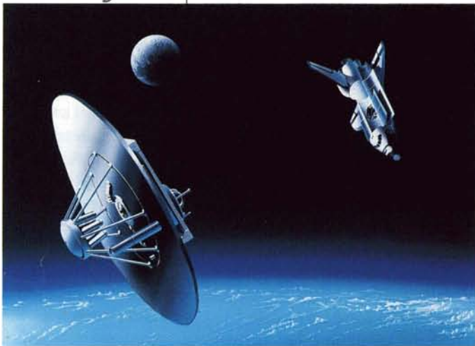
Representative of the broad variety of projects being conducted by NASA's Centers for the Commercial Development of Space is the Wake Shield Facility; a free flying laboratory for growing high purity crystals in space (see page 37).
