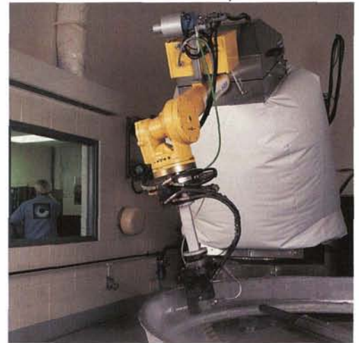
Above is an ARMS robotic workcell operated by Delta Air Lines to remove coatings from jet engine components during overhauls. At right is a closeup of the business end of the robot arm—the end effector—removing the liner (the waffle-like substance).
