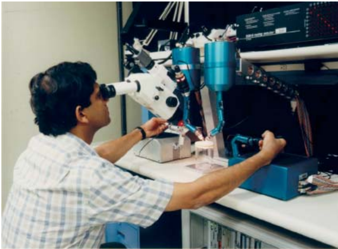
The Robot Assisted MicroSurgery workstation enables new procedures for the brain, eye, ear, nose, throat, face, and hand. The device uses computer compensated motion control to dramatically reduce the effects of operator muscle tremor.
