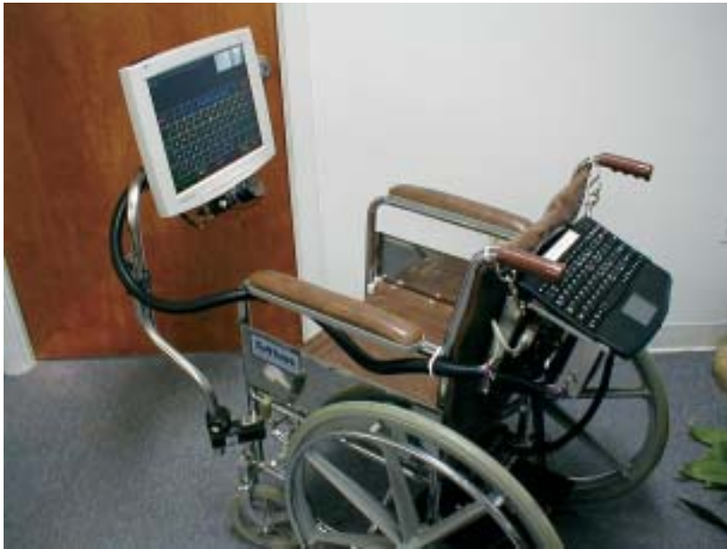
LCT's collaboration with NASA's Jet Propulsion Laboratory reduced the size and weight of the Portable Eyegaze System, which can be conveniently mounted on a wheelchair.
