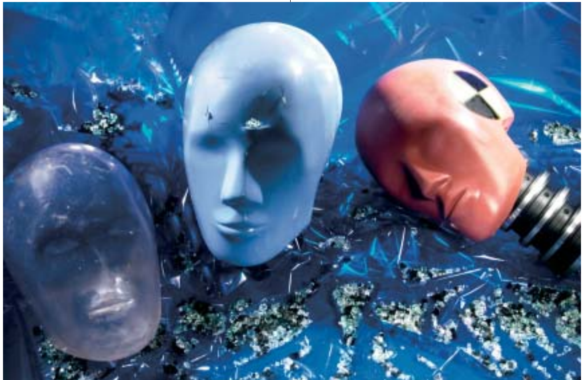
The Transparent Rigid Mask, Facial Laceration Mask, and Hybrid III-50 th percentile Head and Neck simulate effects of kibbled windshield glass on a Laceration Mask.
