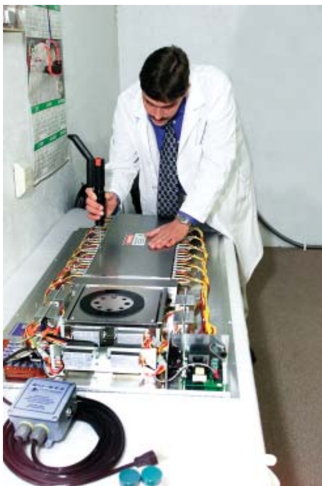
A technician at KES Science & Technology, Inc., assembles the AiroCide TiO 2 , an air purifier that kills 93.3 percent of airborne pathogens that pass through it, including anthrax spores.
