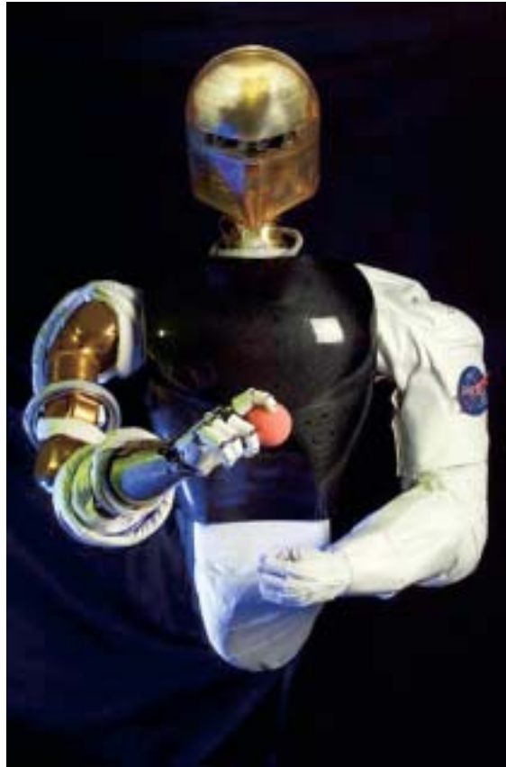
Robonaut is a humanoid robot being developed to function as an astronaut assistant. The dexterous manipulation technology in its hands might one day be used in applications such as human prosthetic development.
