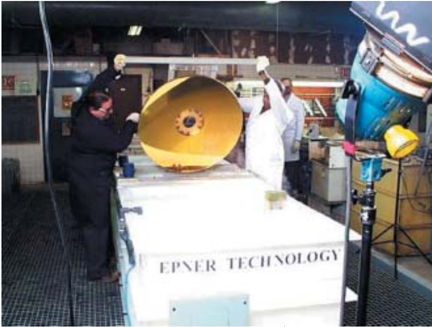
NASA's Vegetation Canopy Lidar mirror was carefully gold-coated to provide it with the sensitivity necessary for operation.
