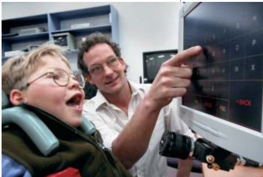
The Eyegaze System enables this boy to communicate using only the movement of his eyes. A video camera focuses on the pupil of the user’s eye, tracking its movement. To “press” a key on the screen, the user looks at the key for a specified time, prompting the computer to take the appropriate action.
