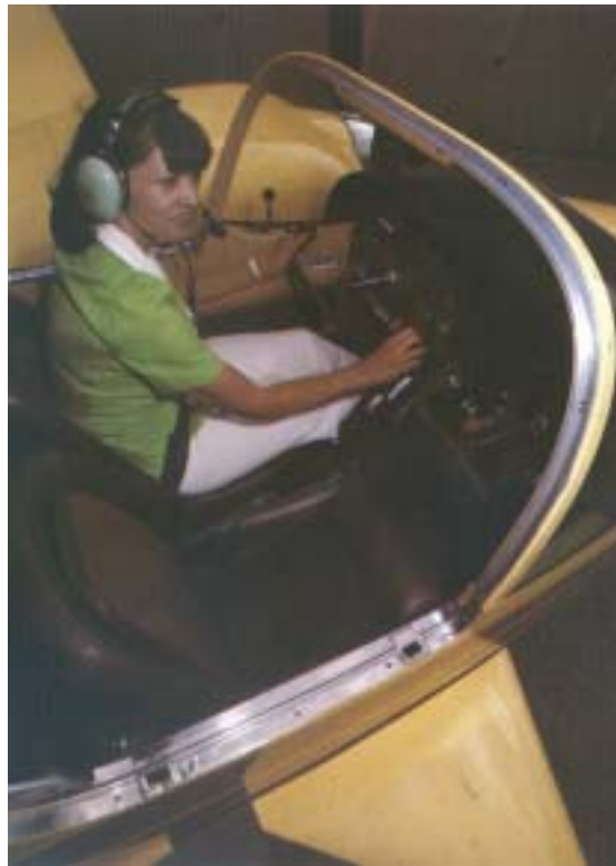
Seats in the cockpit of the Wing Derringer twin-engine lightplane have temper foam padding to reduce pilot and passenger fatigue on long flights.
