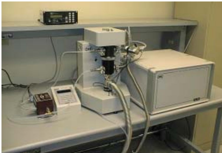
The Force-Balanced Piston Gauge tests and calibrates instruments that operate in the low pressure range.
