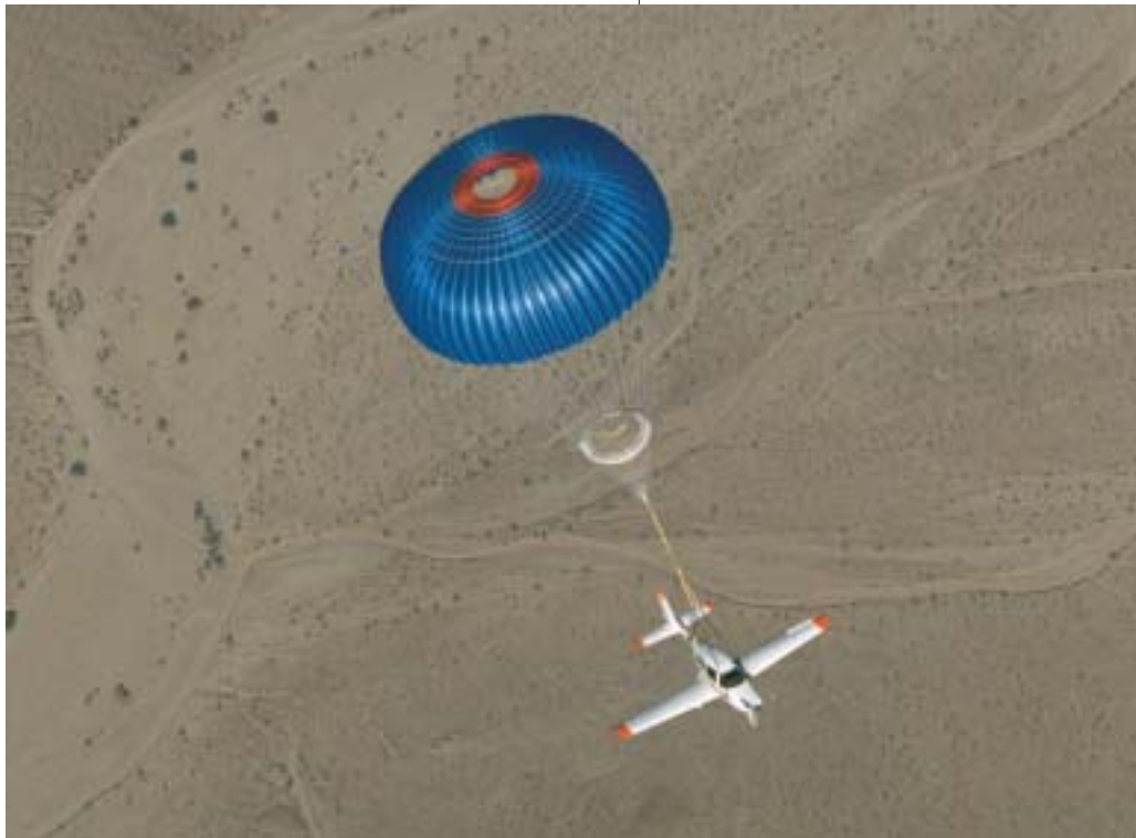
BRS parachutes are lifesavers in cases of engine failure, mid-air collisions, pilot disorientation or incapacitation, unrecovered spins, extreme icing, and fuel exhaustion.
