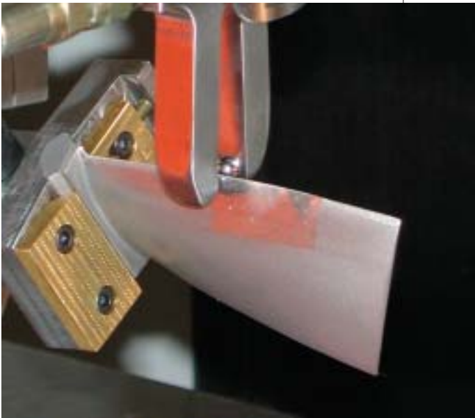
A smooth, free-rolling ball comes into contact only with the surface being burnished.
