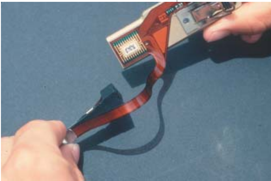
Langley's high-temperature, polyimide adhesive is used to bond film to copper foil conductor materials in flexible circuits produced by one of the Nation's largest circuit board manufacturers.
