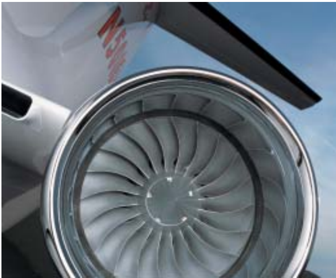
The EJ22 engine, which has a low noise level, light weight, and low fuel consumption, delivers over 770 pounds of thrust while only weighing approximately 85 pounds.
