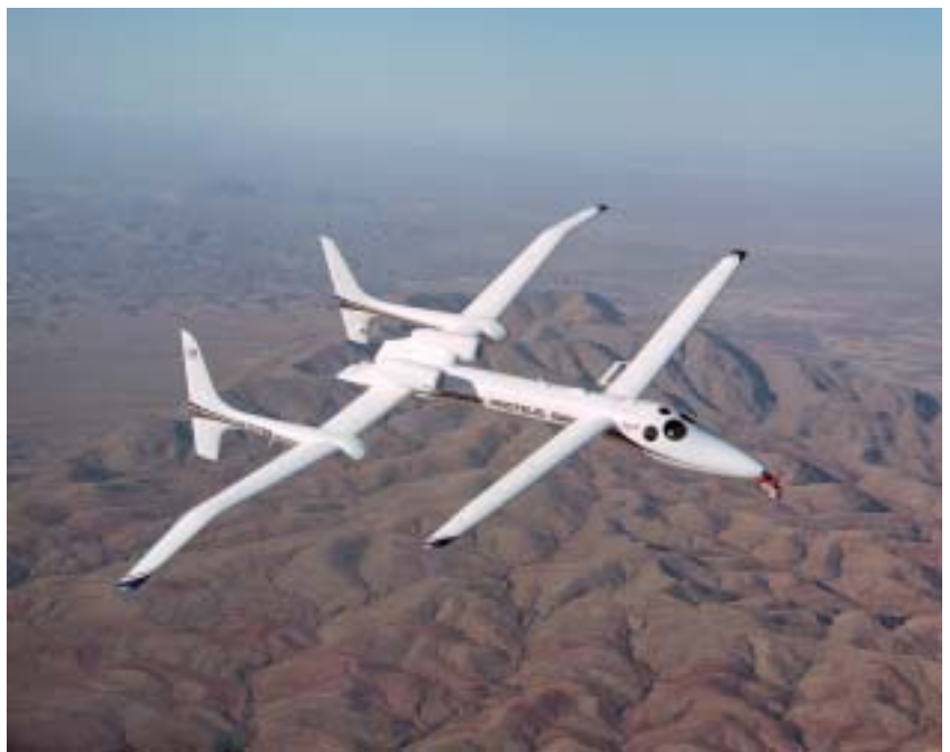
The unique Proteus aircraft served as a test bed for NASA-sponsored flight tests designed to validate collision-avoidance technologies proposed for uninhabited aircraft. The tests, flown over southern New Mexico in March 2002, used the Proteus as a surrogate uninhabited aerial vehicle.
