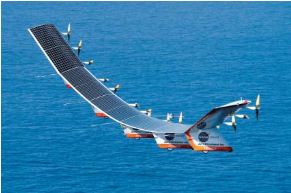
The solar wing Helios aircraft spent about 7 hours above 50,000 feet on its record-breaking, high-altitude flight August 13, 2001.
