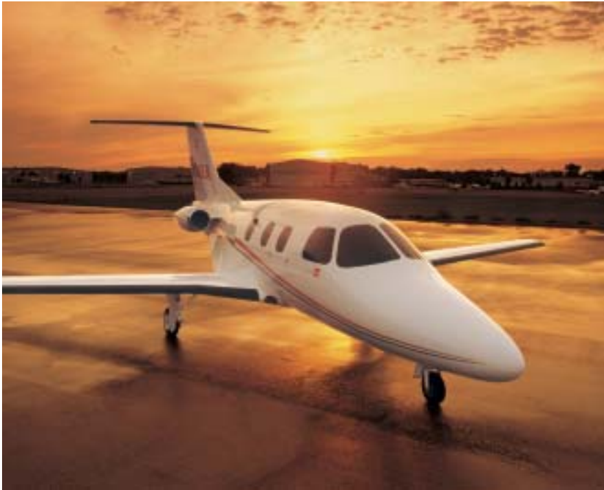
Powered by the EJ22 engine, the Eclipse 500 aircraft is intended to provide “point-to-point” air taxi travel.
