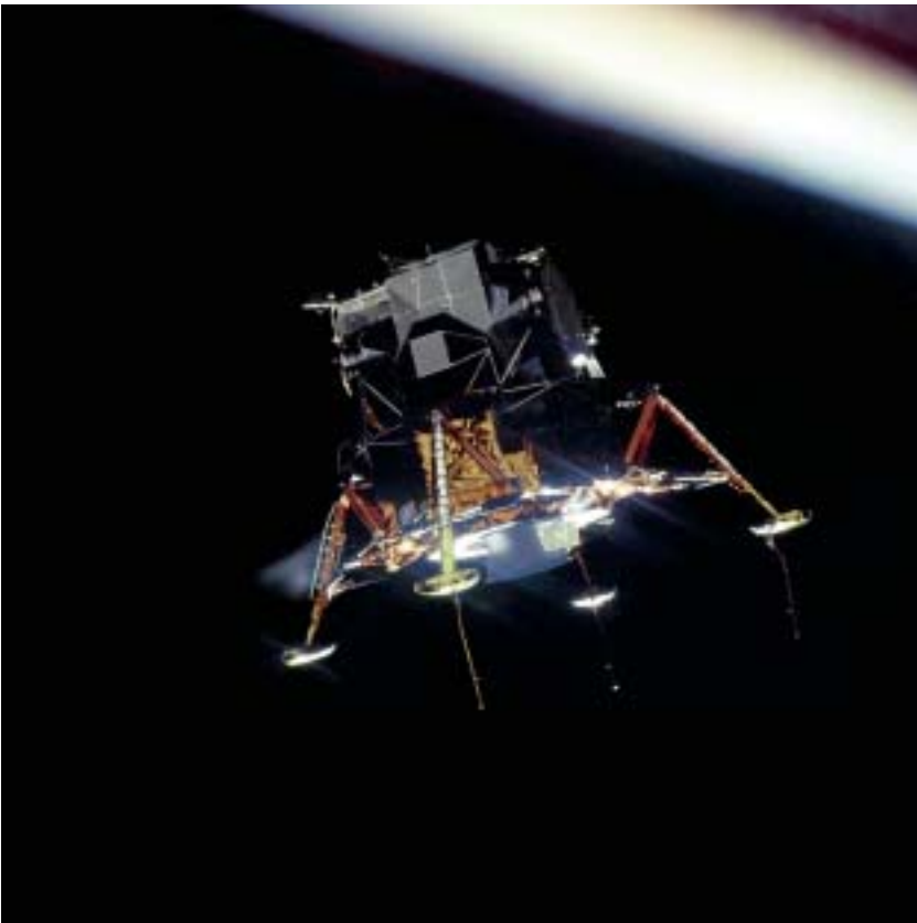
The Apollo 11 Lunar Module "Eagle," in a landing configuration is photographed in lunar orbit from the Command and Service Modules "Columbia."
