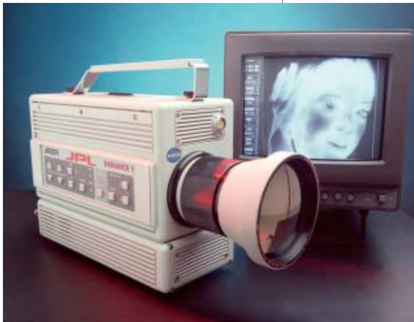
The JPL camera features a large-area, long wavelength QWIP focal plane array, which gives it greater sensitivity, resolution, and stability than previous infrared cameras.
