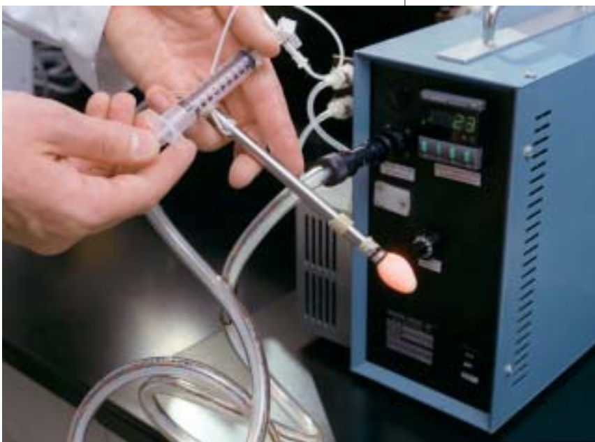
The probe, which is approximately 9 inches long and about one-half inch in diameter, was developed for photodynamic cancer therapy under a NASA Small Business Innovation Research program grant.
