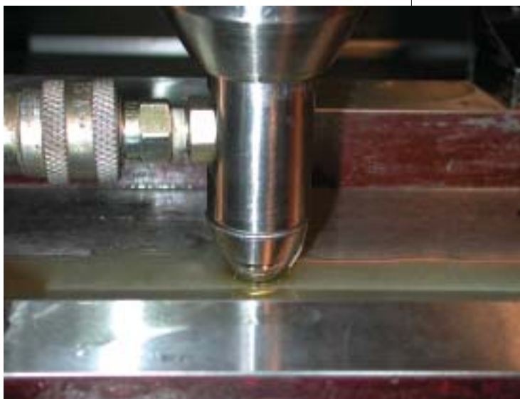
The low plasticity burnishing process improves a surface's resistance to fatigue and damage.
