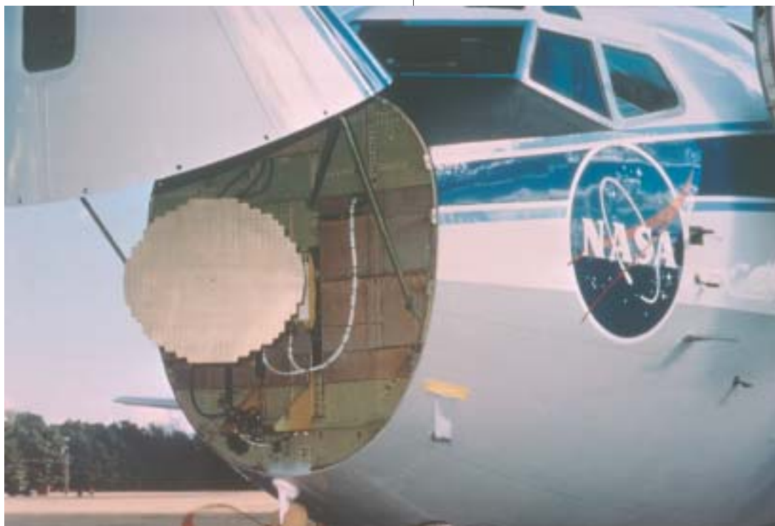
Langley's Boeing 737 research aircraft is fitted with a Doppler radar wind shear detection system that sends a beam well ahead of the airplane to detect microbursts, evidenced by sudden large changes in raindrop velocities.
