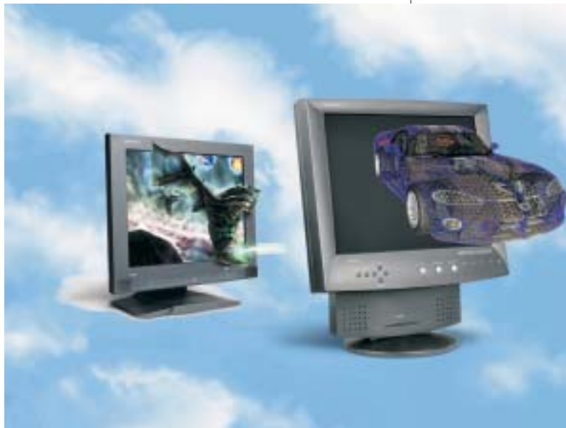
The Virtual Window ™ system tricks the brain into seeing 3-D by creating two images of an object as seen from two slightly different angles. The image appears to leap off the screen as a result.
