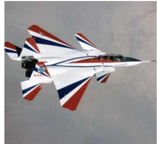
Originally an F-15 fighter, NASA's NF-15B Intelligent Flight Control System aircraft has validated adaptive control concepts that may improve commercial aviation safety.
