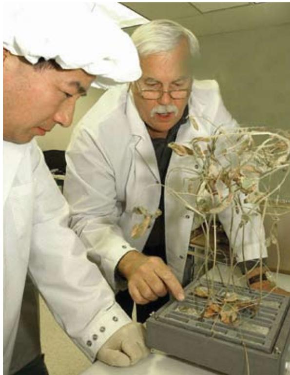
Dr. Weijia Zhou (left), director of the Wisconsin Center for Space Automation and Robotics at the University of Wisconsin-Madison, inspects soybeans grown in the plant growth unit aboard the International Space Station (ISS). Coating technology used inside the miniature plant greenhouse removes ethylene, a chemical produced by plant leaves that can cause plants to mature too quickly.
