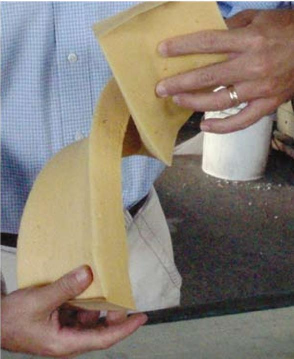
foam is formed at room temperature and then cured using large microwaves, which reduces costs and increases the company's production rates. The finished product can be flexible or rigid, structural or non-structural, and is always highly durable. This affordable insulating foam can also be applied to gaskets and seals, vibration damping pads, spacers in adhesives and sealants, extenders, and flow-leveling aids.
