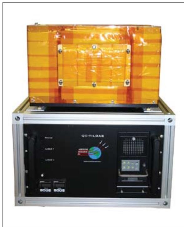
In 2002, ARI introduced a line of thermoelectrically cooled quantum cascade (QC) TILDAS instruments for use in its mobile laboratories. The QC-TILDAS instruments are incorporated into a system that contains the tunable laser, infrared detectors, power electronics, a microcomputer with integrated control and data analysis software, and an astigmatic multiple pass absorption cell.
