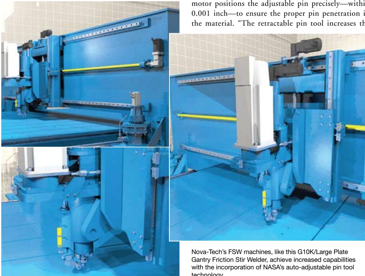
Nova-Tech’s FSW machines, like this G10K/Large Plate Gantry Friction Stir Welder, achieve increased capabilities with the incorporation of NASA’s auto-adjustable pin tool technology.
