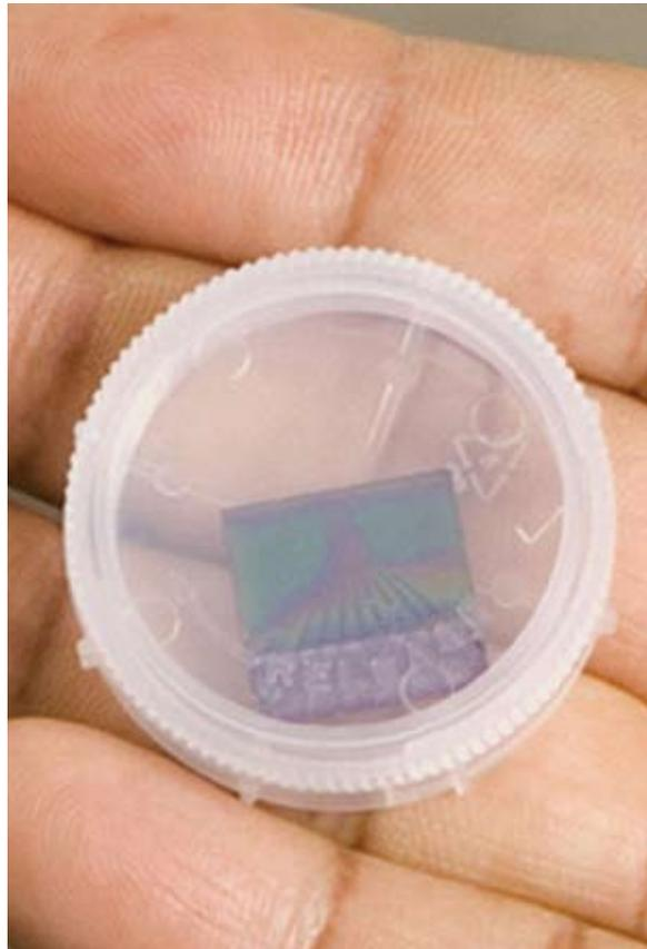
Containing millions of carbon nanotubes, the NASA biosensor can alert inspectors to minute amounts of potentially dangerous organic contaminants.
