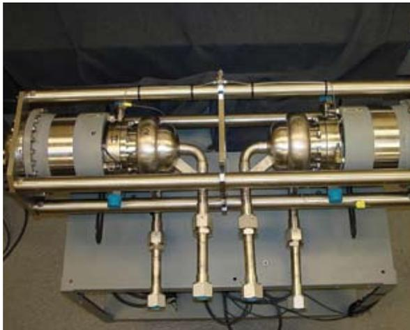
With the ability to generate electricity from heat, Stirling converters could provide new possibilities for sustainable energy.
