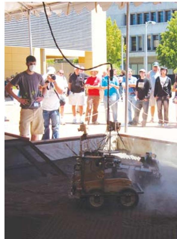
This year, the Regolith Excavation Challenge was held on the campus of the California Polytechnic State University. The competition required teams to build a roving excavator that could autonomously navigate, excavate, and transfer 150 kg of simulated lunar regolith (lunar soil) into a collector bin within 30 minutes.
