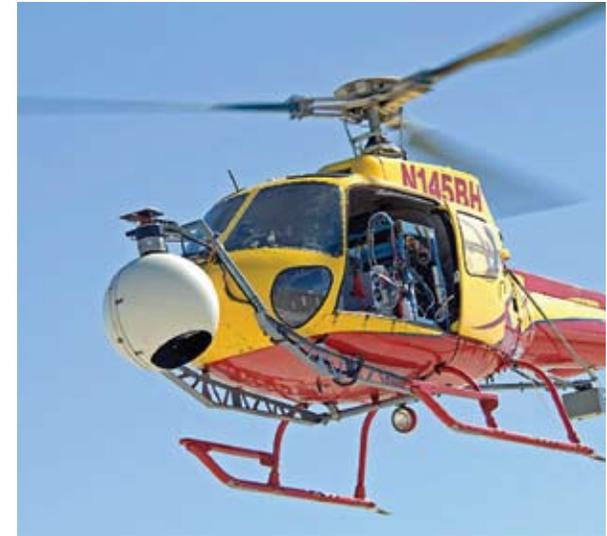
The flash lidar technology mounted on the nose of this helicopter may one day enable automated space docking and precise lunar landings.
