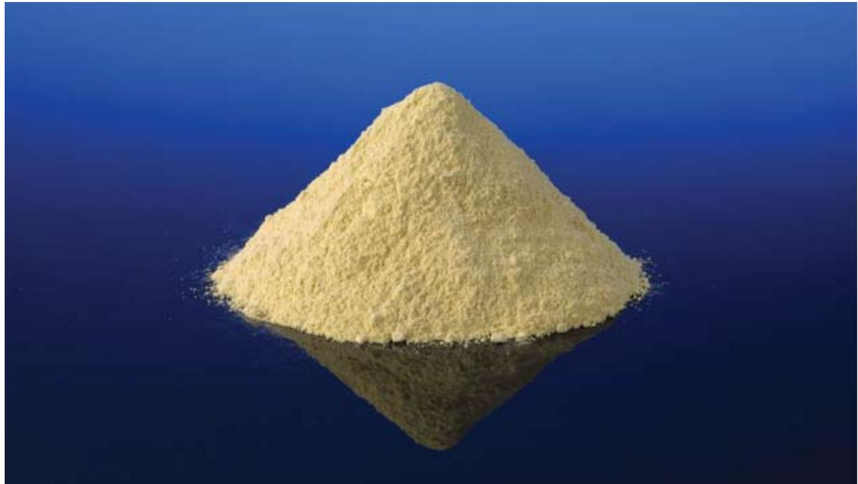
PETI-330 is the first resin created specifically for high-temperature composites formed with resin transfer molding and resin infusion. Offering processability, toughness, and high-temperature performance, the resin has a low-melt viscosity and, when cured, a high glass transition temperature.
