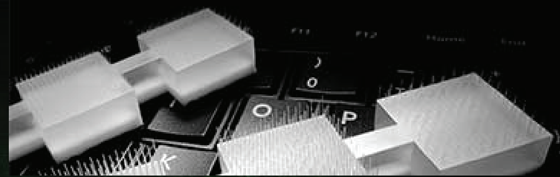
Not limited to lasers, Potomac Photonics also fabricates tiny, plastic parts with a high-precision 3D printer. These molds the company made for Johns Hopkins University were used to make high-aspect ratio wells in a polymer material.
