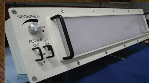
NASA's solid state lighting module, which was flown to and used on the ISS in place of traditional fluorescent lighting. The LED module could be controlled from the ground and uses different colors of light in an attempt to induce focus and alertness or rest and relaxation as needed.
