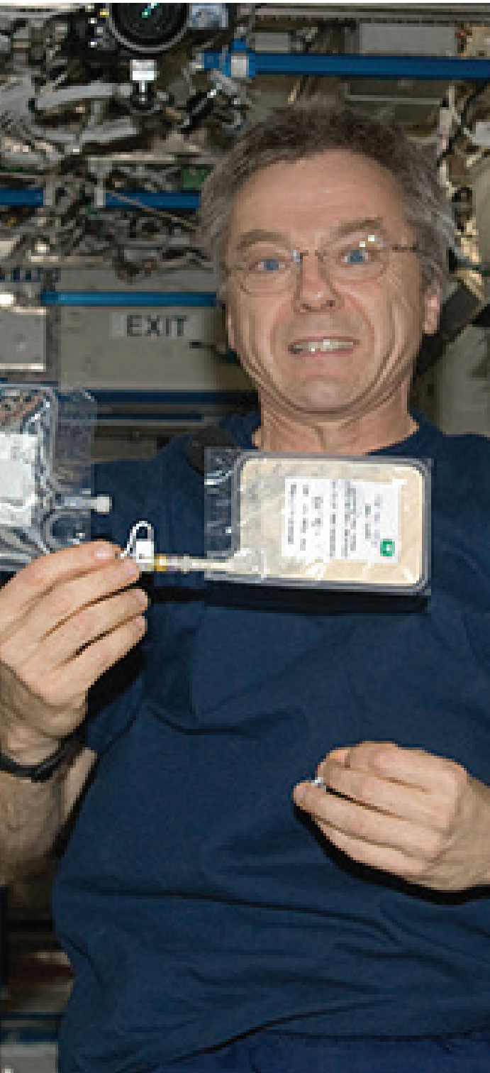
Canadian astronaut Robert Thirsk shows the coliform bacteria test kit that is used onboard the International Space Station. The test is designed to be lightweight and simple yet accurate.
