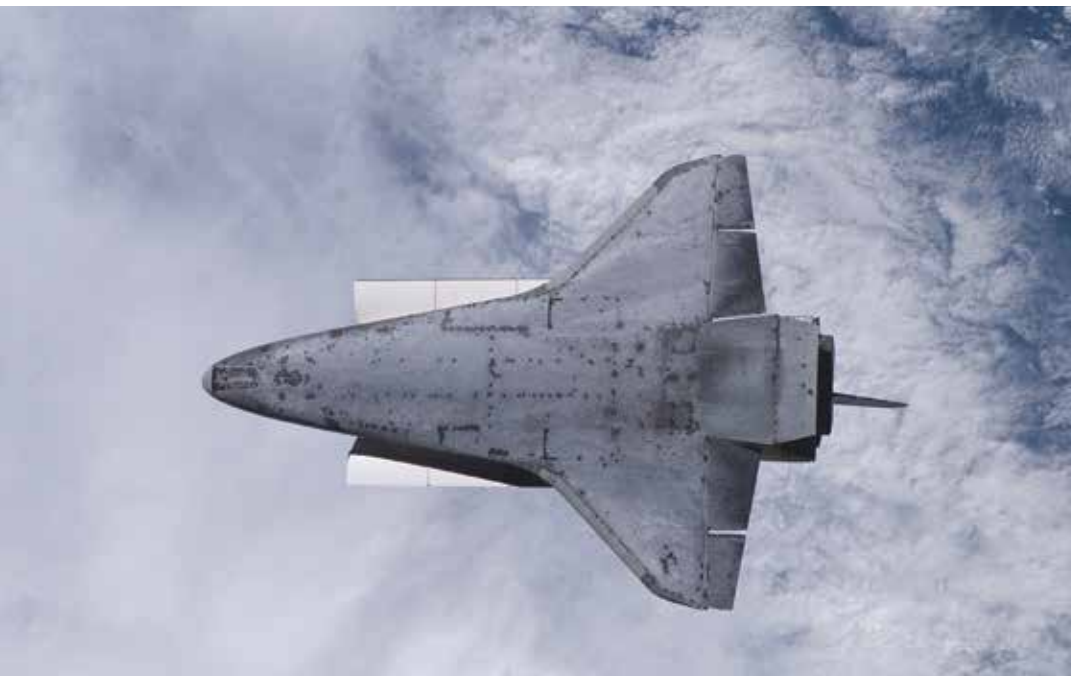
A view of the Space Shuttle Endeavour as the STS-118 crew puts the spacecraft through a rendezvous pitch maneuver, allowing the crewmembers on the nearby ISS to document the vehicle's thermal protection system condition.
