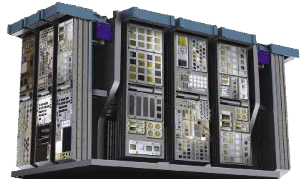
This is a prototype of Alpha Space's MISSE facility. With containers facing in four directions and able to open and close independently, the facility can customize space exposure for different samples.
