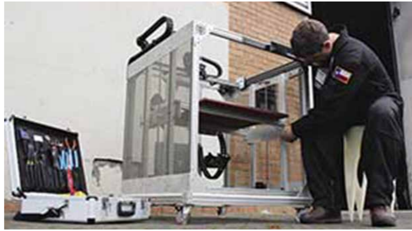
The founders of re:3D drew on experience at Johnson Space Center to design and sell a large-scale 3D printer at a low cost. The standard configuration prints items up to eight cubic feet, or 30 times larger than competing desktop models.
