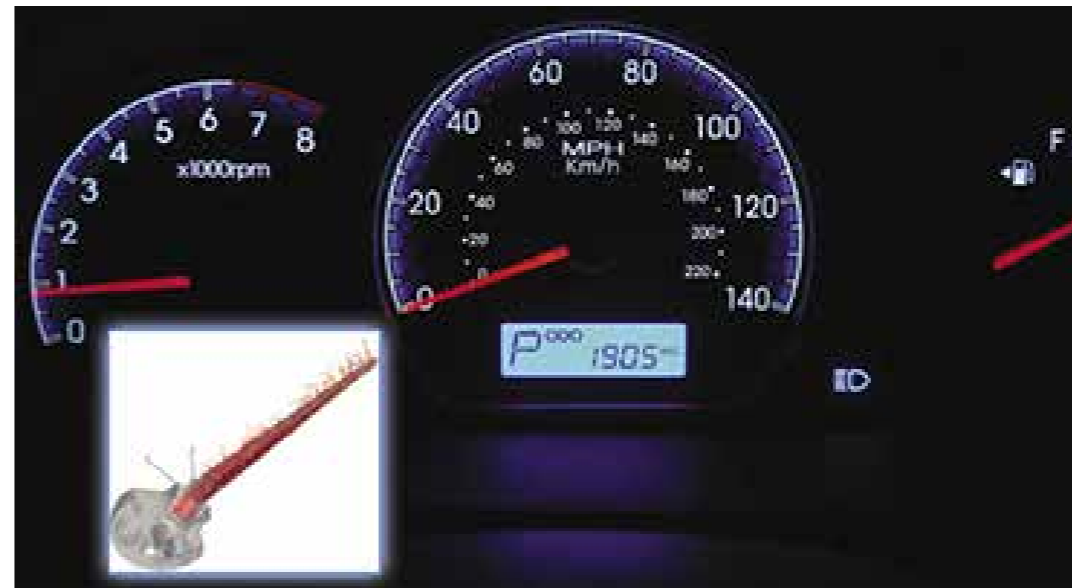
Automakers use TracePro to model dashboard displays. In the inset, the program predicts the behavior of light rays through a computer-aided design of a speedometer needle.
