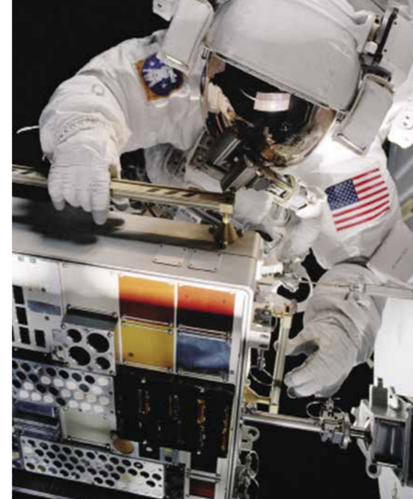
An astronaut installs a Materials International Space Station Experiment (MISSE) facility on the exterior of the ISS during a spacewalk in 2001. Future iterations of MISSE, handled by Alpha Space, will be installed and maintained via robotic arm, eliminating reliance on spacewalks.
