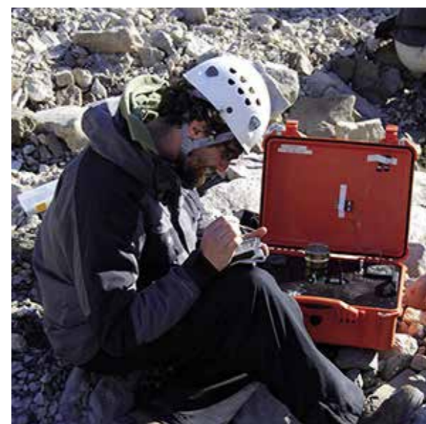
The easy sample preparation requirements—knock a rock fragment loose and crush it with a small hammer—plus the portability, low cost, and one-button operation have made the Olympus TERRA and BTX II Benchtop XRD devices popular in the oil and gas industry, as well as with pharmaceutical companies and drug watchdog groups.
