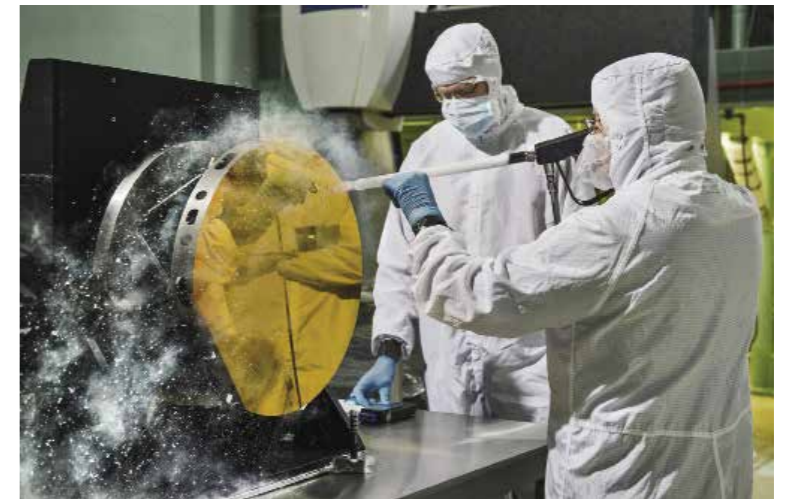
Engineers at Goddard Space Flight Center use carbon dioxide "snow" to clean a test mirror for the James Webb Space Telescope. Because they're cold, components like mirrors and lenses, which have to be completely clean and flawless in space imagers, are among the first places any volatile compounds outgassed from a spacecraft's materials will condense, causing fogging. To prevent this, all materials used in spacecraft have to demonstrate extremely low outgassing.
