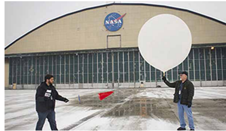
Glenn Research Center icing expert Michael King (left) prepares to launch a weather balloon equipped with a supercooled liquid water sensor designed by Anasphere Inc. Results from balloon launches such as this one will help verify whether a ground-based NASA system can effectively predict icing conditions aloft.
