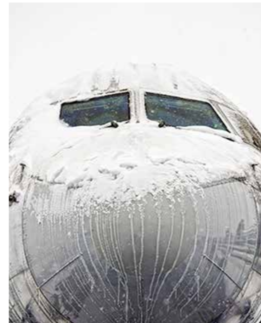
Ice poses a significant hazard to planes in the air, where it can accumulate on wings and engines. NASA is studying ways to better predict when icing conditions are particularly dangerous, and one tool it is using to test its research, a lightweight, inexpensive sensor, is proving useful outside the agency as well.
