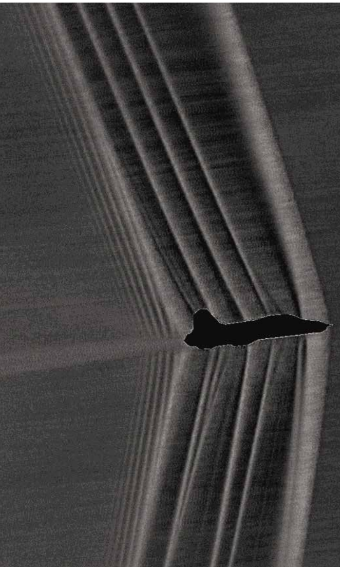
This photo, taken to help NASA engineers working on making sonic booms quieter, shows the air flow around an airplane as it surpasses the speed of sound—a visual representation of breaking the sound barrier.
