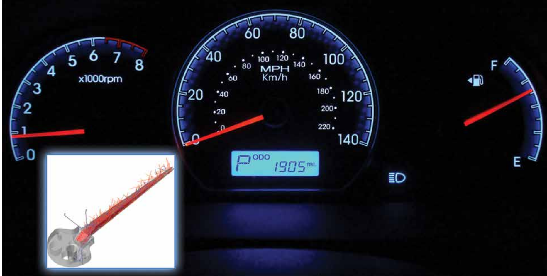
Automakers use TracePro to model dashboard displays. In the inset, the program predicts the behavior of light rays through a computer-aided design of a speedometer needle.
