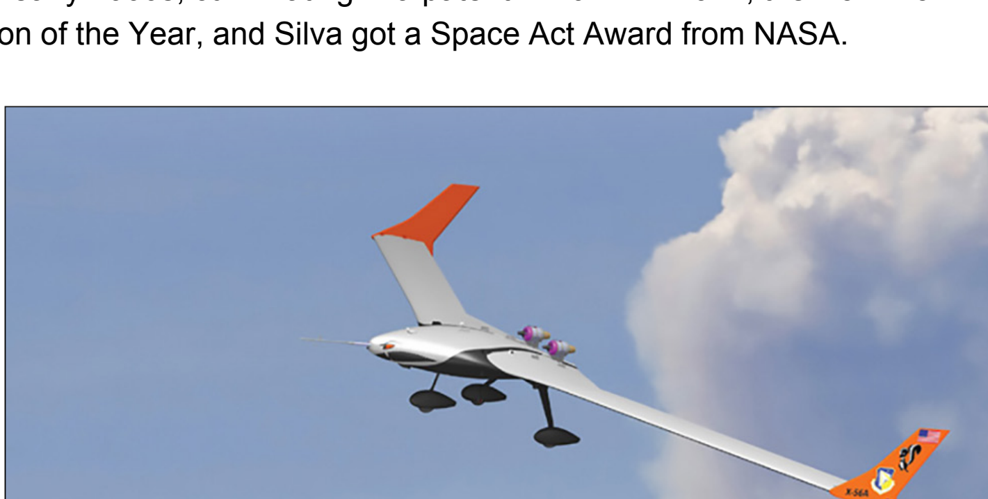
CFD Research Corporation used Silva's Reduced Order Modeling software in a project to design aircraft with an extra-long wing span to increase fuel efficiency. Designs were tested on the X-56 MUTT, which stands for multi-use technology test bed.
