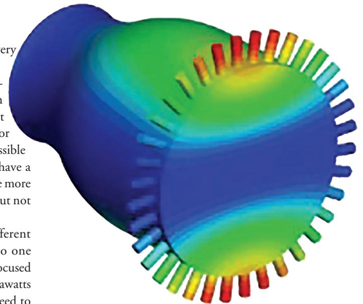
Gloyer-Taylor Laboratories (GTL) has created a software toolkit that models and analyzes structures for combustion instability, calculating the bulk flow of energy and then continuing on in layers, analyzing acoustics, vorticity, and then the thermal entropic energy. The company received multiple SBIR contracts from NASA to help design and test the toolkit, including the acoustics component called Resonance, which generated the image here.
