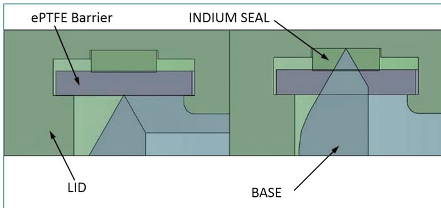
This diagram shows a lid specially designed for a Mars sample return mission. To ensure no Mars dust interferes with the seal, the edge of the base first pushes through an extruded ePTFE barrier to wipe it clean, before it sets in a layer of soft indium metal, which ensures nothing gets in or out.
