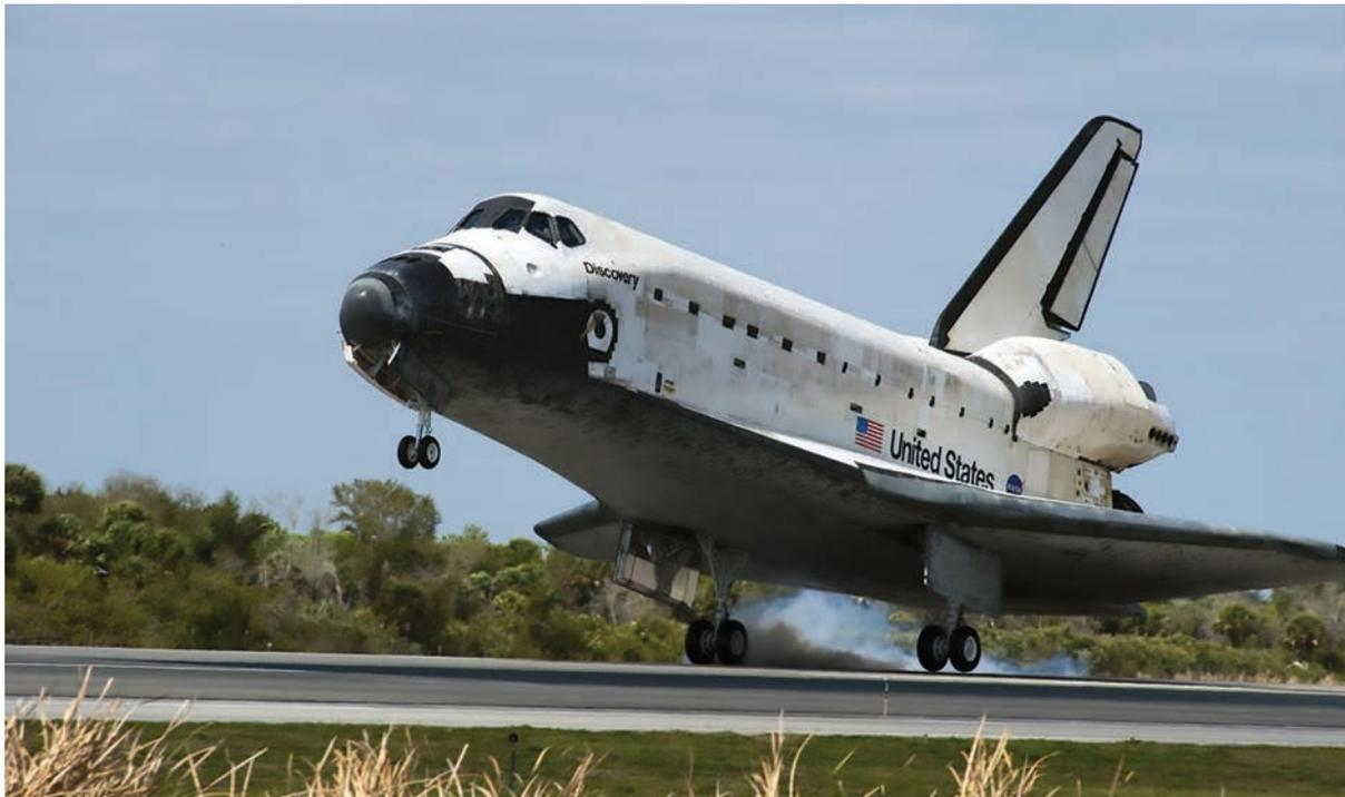
Proper tire pressure is crucial for a safe landing, but in the early days of the Space Shuttle Program, there was no good way to accurately gauge pressure in flight. Instead, engineers relied on extensive pre-flight ground tests to measure air loss over time.
