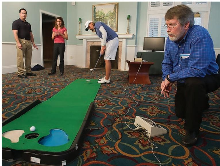
Langley Research Center engineer Alan Pope, right, built and patented a mechanical putting green that works as a biofeedback training device, teaching subjects to control their state of mind. The green undulates, with its hole expanding and contracting and the sighting laser moving back and forth until the user's brainwave readings indicate a quiet, empty mind.
