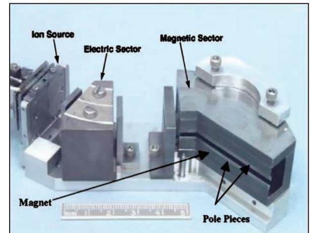
In the Mattauch-Herzog mass spectrometer configuration, ions are deflected first by an electrical field and then by a magnetic field to sort them by weight before they strike a focal plane that detects all the ions simultaneously. The CCD-based prototype created at JPL accomplished this within a small, rugged, inexpensive, energy-efficient device.
