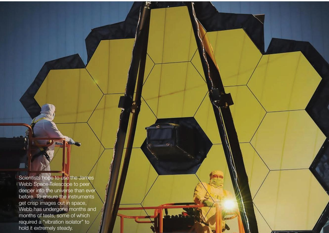
Scientists hope to use the James Webb Space Telescope to peer deeper into the universe than ever before. To ensure the instruments get crisp images out in space, Webb has undergone months and months of tests, some of which required a "vibration isolator" to hold it extremely steady.
