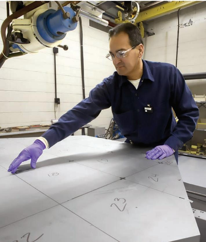
A radiographer at Brush Wellman, now Materion Corporation, prepares a beryllium mirror blank for an X-ray radiograph. The slab was later machined down to create a mirror for the James Webb Space Telescope.
