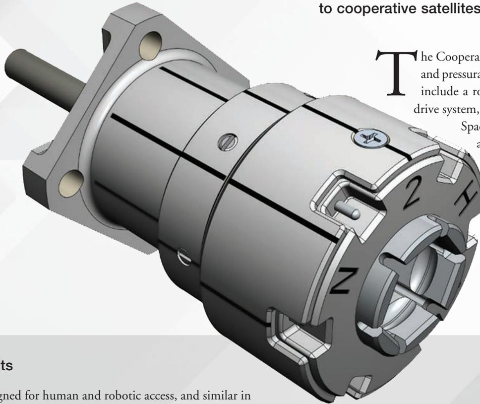
The Cooperative Service Valve (CSV) facilitates the resupply of media, such as propellants and pressurants, to satellites, replacing a standard spacecraft fill-and-drain valve. Advantages include a robotic interface, three individually actuated seals, a self-contained anti-back drive system, and built-in thermal isolation.
