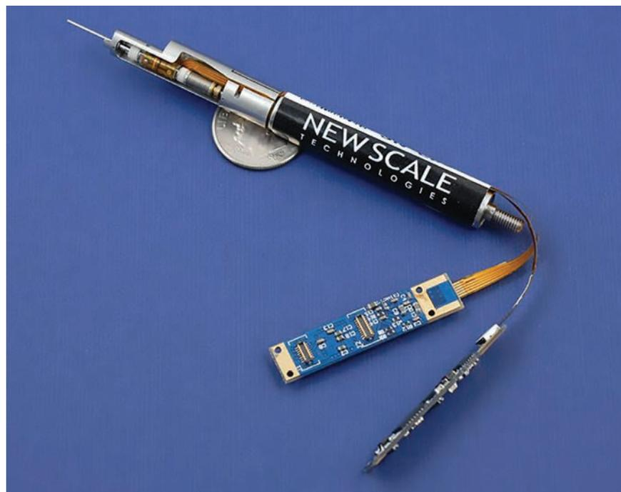
Each of nearly 2,400 fibers on the fiber-fed spectrograph must move independently and needs a range of motion that can cover any point on the image. New Scale Technologies designed and manufactured an extremely tiny, low-voltage positioner that combines two rotary motors. The company now uses the technology on many of its products, including ones that turn up in medical instruments, like a portable blood analyzer that tests for HIV.
