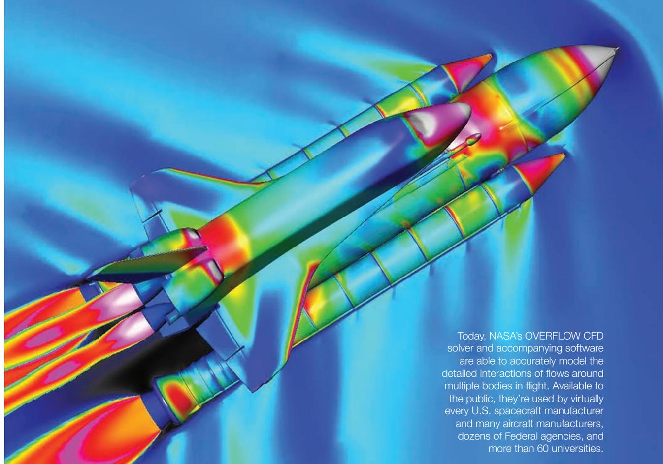
Today, NASA’s OVERFLOW CFD solver and accompanying software are able to accurately model the detailed interactions of flows around multiple bodies in flight. Available to the public, they’re used by virtually every U.S. spacecraft manufacturer and many aircraft manufacturers, dozens of Federal agencies, and more than 60 universities.
