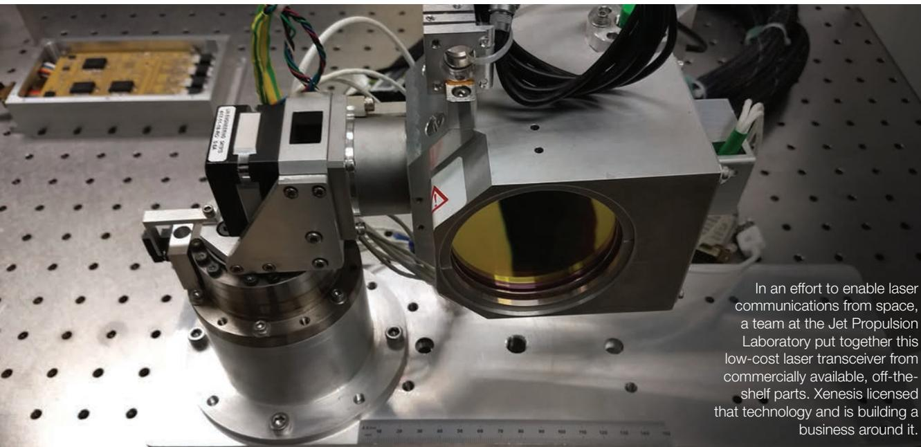
In an effort to enable laser communications from space, a team at the Jet Propulsion Laboratory put together this low-cost laser transceiver from commercially available, off-the-shelf parts. Xenesis licensed that technology and is building a business around it.
