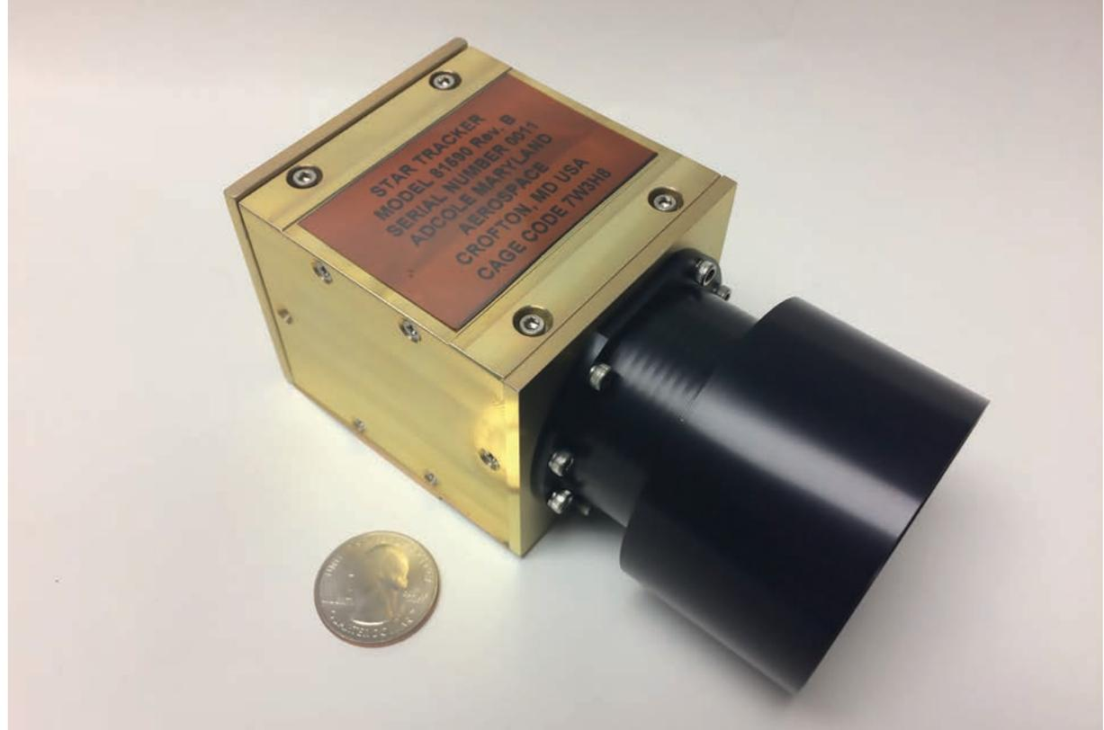
This tiny device fits inside a CubeSat and contains all the hardware and software to precisely point the miniature satellite—within 0.1 degrees of error. Developed by Adcole Maryland Aerospace with funding from several SBIR contracts, it is at least an order of magnitude more precise than previous pointing devices for CubeSats.
