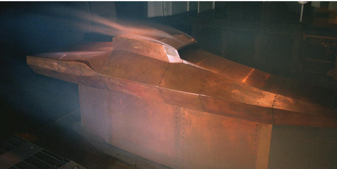
Langley Research Center funded Tao Systems’ efforts to make the first constant voltage anemometers (CVA) in the early 1990s, primarily for high-speed wind tunnel testing. Here, the experimental X-43 hypersonic aircraft undergoes testing in Langley’s eight-foot, high-temperature wind tunnel. Tao Systems is still the only company producing CVAs, which provide highly accurate wind velocity and temperature readings.
