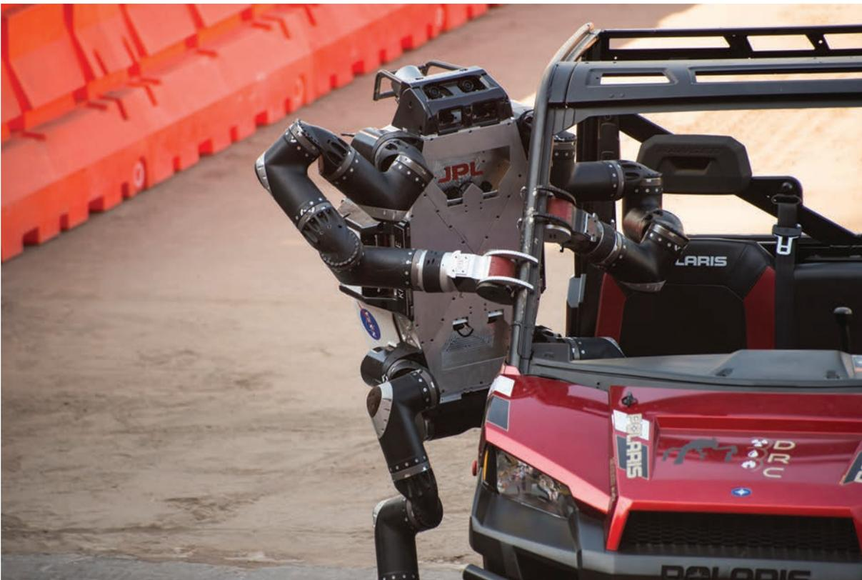
Jet Propulsion Laboratory (JPL) engineers built RoboSimian to compete in the 2015 DARPA Robotics Challenge, where it had to perform tasks like clearing a path through rubble, traversing a heap of cinderblocks, and driving a vehicle. Even before the competition’s final rounds, the entire robot was available for license as a package.
