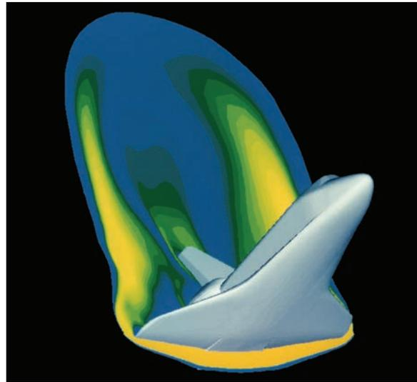
NASA uses a variety of tools to create simulations, including the computational fluid dynamics software used to simulate the aerodynamics of Space Shuttle descent here. The Distributed Observer Network (DON) can read and display any of those simulations.
