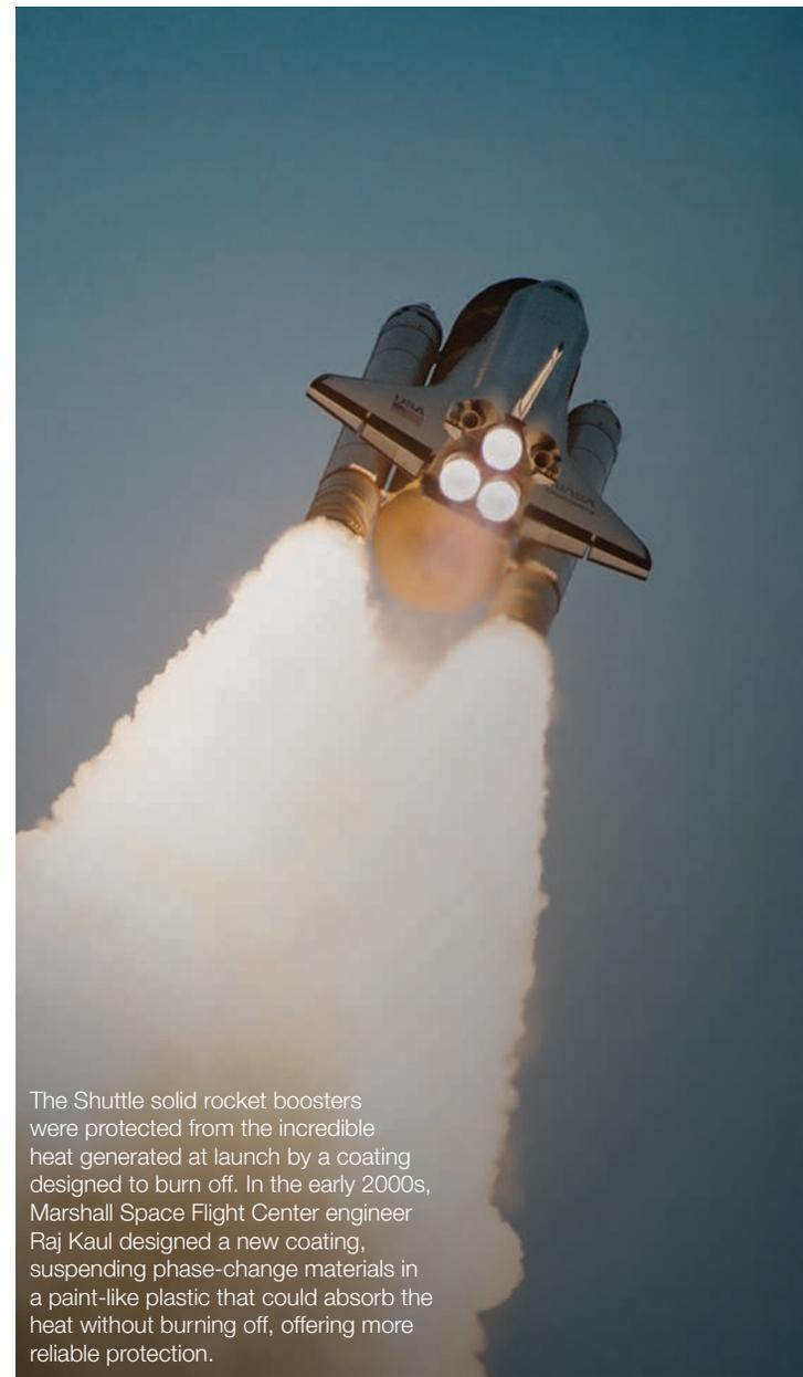
The Shuttle solid rocket boosters were protected from the incredible heat generated at launch by a coating designed to burn off. In the early 2000s, Marshall Space Flight Center engineer Raj Kaul designed a new coating, suspending phase-change materials in a paint-like plastic that could absorb the heat without burning off, offering more reliable protection.
