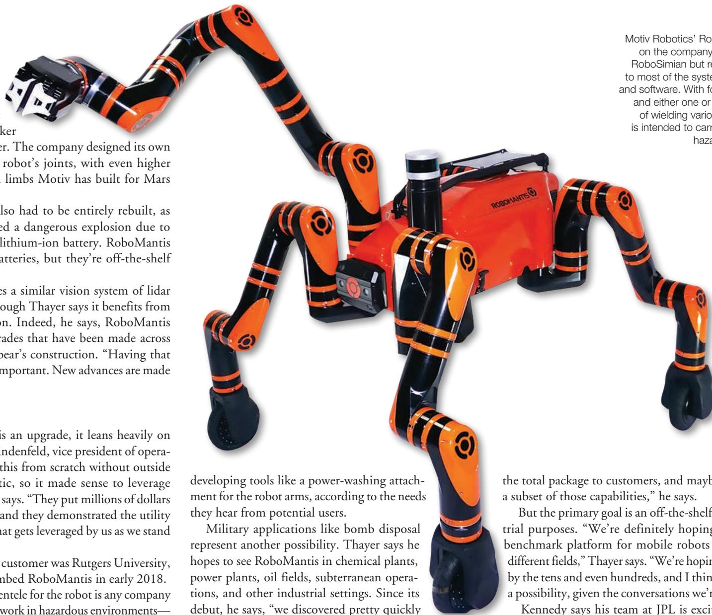
Motiv Robotics' RoboMantis is based on the company's license for JPL's RoboSimian but represents updates to most of the systems, components, and software. With four legs on wheels and either one or two arms capable of wielding various tools, the robot is intended to carry out jobs that are hazardous to humans.
