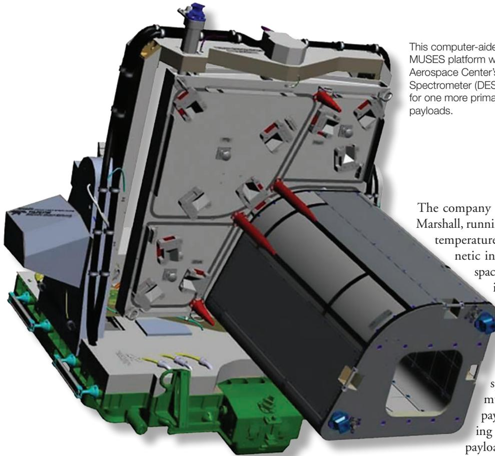
This computer-aided design drawing shows the MUSES platform with its first tenant, the German Aerospace Center's DLR Earth Sensing Imaging Spectrometer (DESI). There is room remaining for one more primary payload and two secondary payloads.
