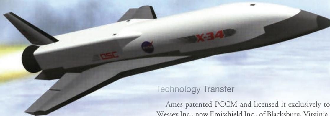
The planned X-33 and X-34 experimental spaceplanes, which would fly at up to 15 times the speed of sound, required even more robust thermal protection systems than existing spacecraft. Ames Research Center scientists responded by creating the flexible, paper-thin, highly emissive Protective Coating for Ceramic Materials (PCCM), capable of withstanding temperatures up to 3,000 °F.
