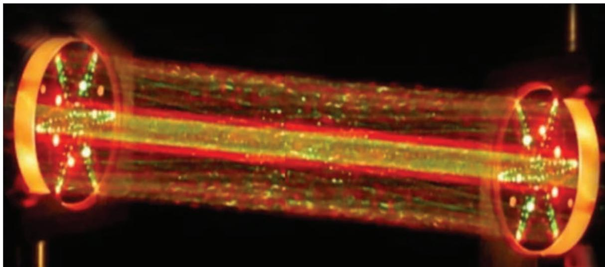
The Tunable Laser Spectrometer (TLS), installed on the Curiosity rover, was designed to measure traces of methane, carbon dioxide, and water vapor. It works by shooting lasers into a measurement chamber filled with Martian air and measuring absorption of light at specific wavelengths. This demonstration of the spectrometer used visible lasers, as opposed to the infrared lasers on the real device.
