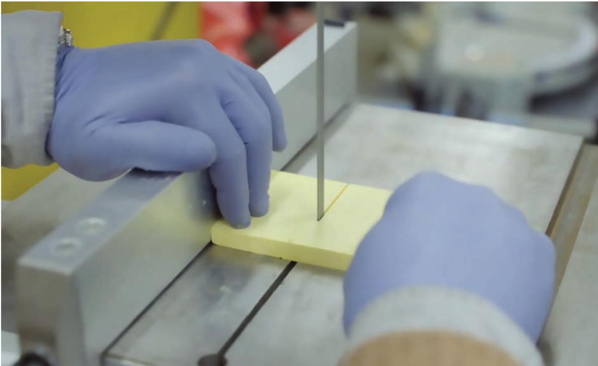
Aerogel Technologies, thanks to internal research and development as well as several technologies it has licensed from Glenn, manufactures a class of aerogels it has branded Airloys. They can be made with a variety of properties, including high temperature tolerance, transparency, and varying degrees of flexibility and stiffness, and can be cut and machined into any shape.
