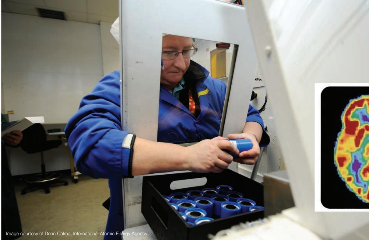
A technician packages radioactive pharmaceuticals into shielded containers. One possible application for Applied Spectra's Laser Ablation Molecular Isotopic Spectrometry technology is in nuclear medicine, where it could be used to remotely inspect radioactive materials.
