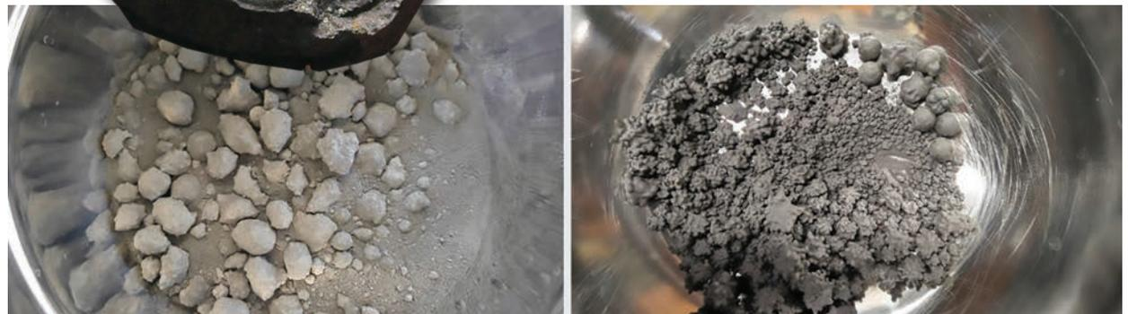
DSI customers can buy raw asteroid simulant powders or mixes of a range of grain sizes.
