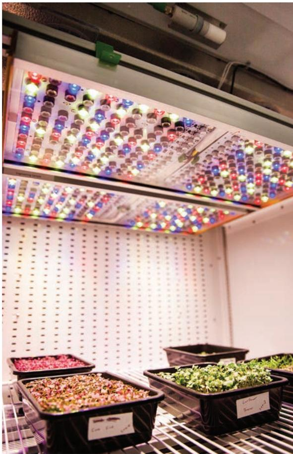
The Phytofy system's lighting capability and range of choice allow NASA researchers on Earth to simulate the lighting capabilities of the Advanced Plant Habitat, a growth chamber that astronauts began using on the ISS in early 2018.
