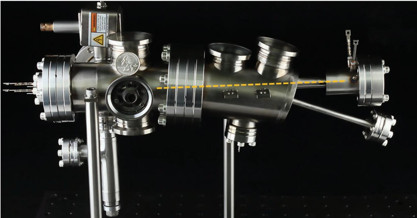
This laser-cooled atomic source “powers” an optical atomic clock. Unlike lab-size versions, this source consumes less than five watts and fits in a shoebox, while actually outperforming its larger predecessors.
