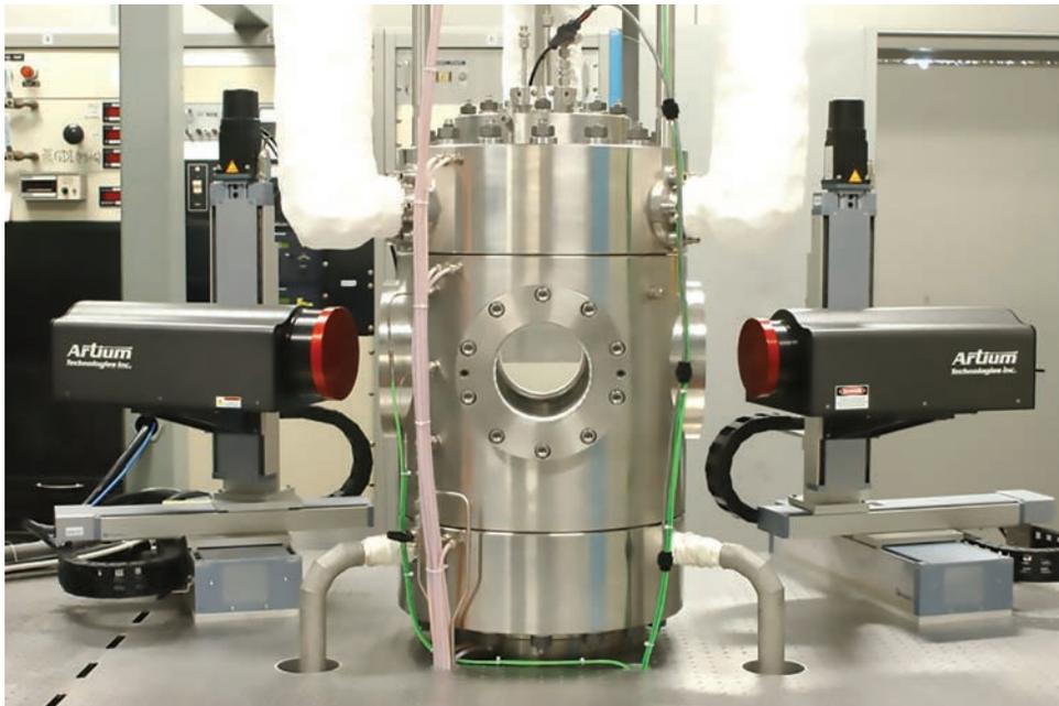
Artium's Phase Doppler Interferometer is used to test fuel injectors at a General Motors facility. Most automakers use Artium technology, which was originally created to test rocket and jet engines.
