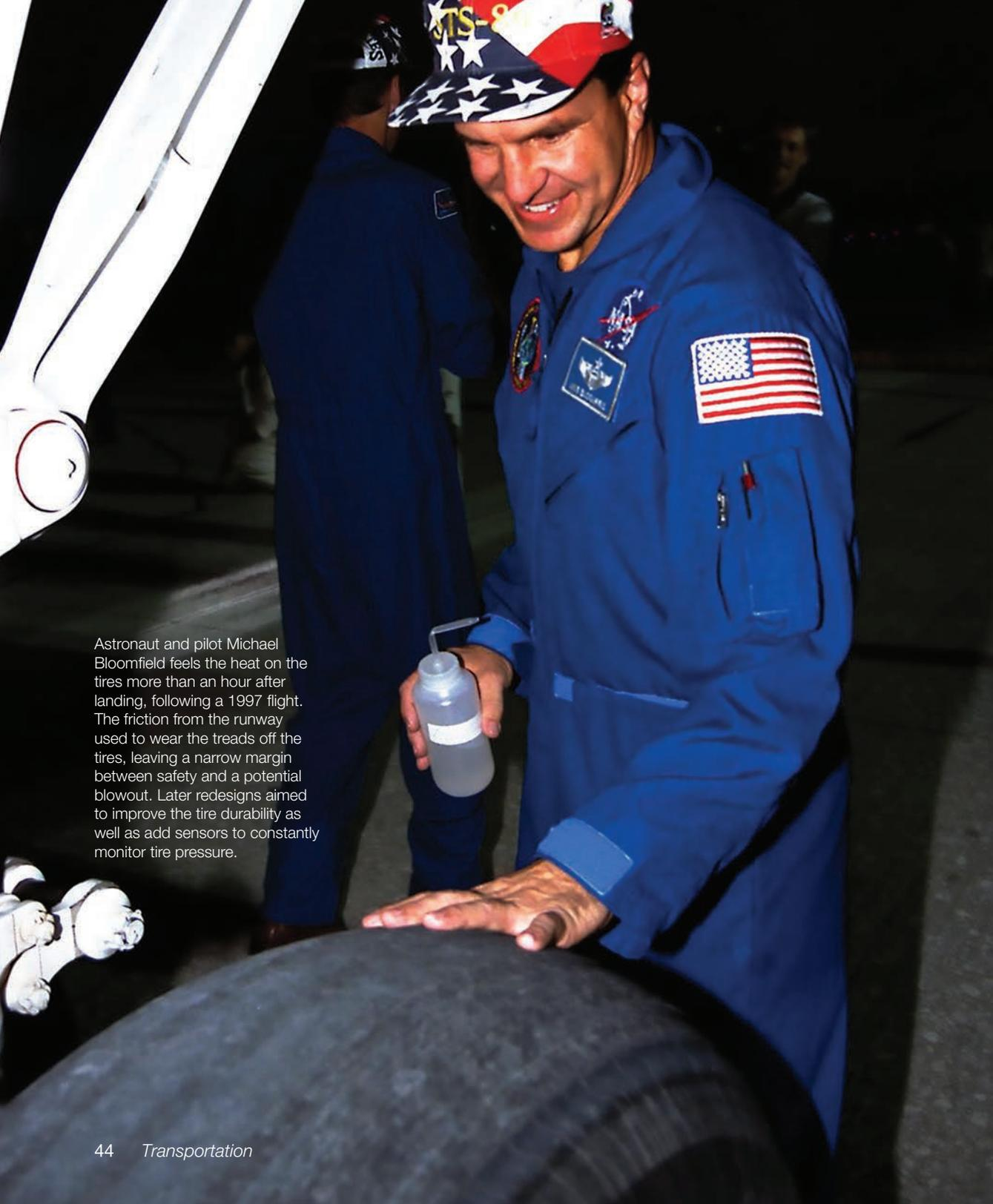
Astronaut and pilot Michael Bloomfield feels the heat on the tires more than an hour after landing, following a 1997 flight. The friction from the runway used to wear the treads off the tires, leaving a narrow margin between safety and a potential blowout. Later redesigns aimed to improve the tire durability as well as add sensors to constantly monitor tire pressure.
