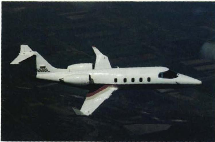
program, the winglet is an aerodynamic innovation designed to reduce fuel consumption and generally improve airplane performance. Gates Learjet was the first manufacturer to use the winglet design in production-type jets, initially on the Longhorn 28/29 models introduced to service in 1979. Several other plane builders are taking advantage of the NASA technology.
