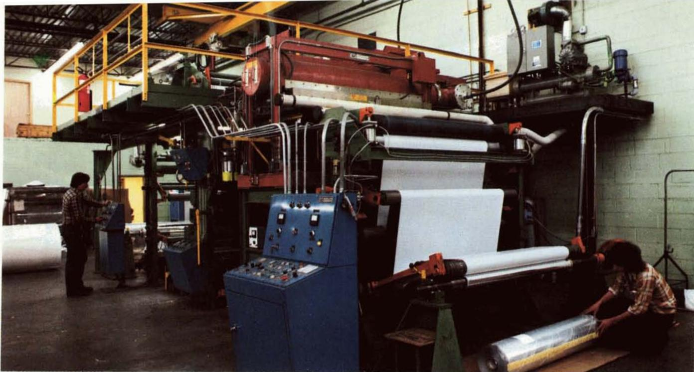
*This sophisticated King-Seeley equipment is employed in a new electron beam processing technique for curing—instantly drying—solid coatings; the coatings are exposed to streams of electrons and cured in five-thousandths of a second. The machine also laminates sheets of material for greater strength and quick-cures the laminating adhesive.*
