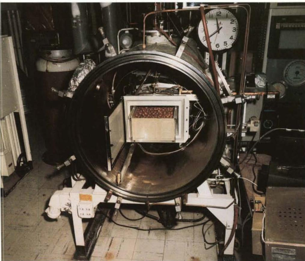
*In early trials, McDonnell Douglas Corporation used this space environment simulator to test the feasibility of vacuum-drying farm produce.*
