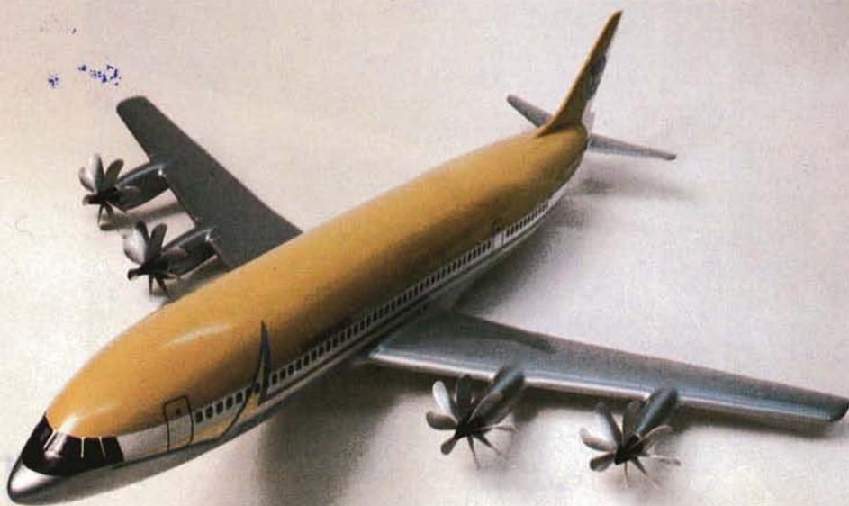
*Advanced technology turbine-driven propellers with reshaped blades could provide jetlike speeds with sharply reduced fuel consumption. The*
