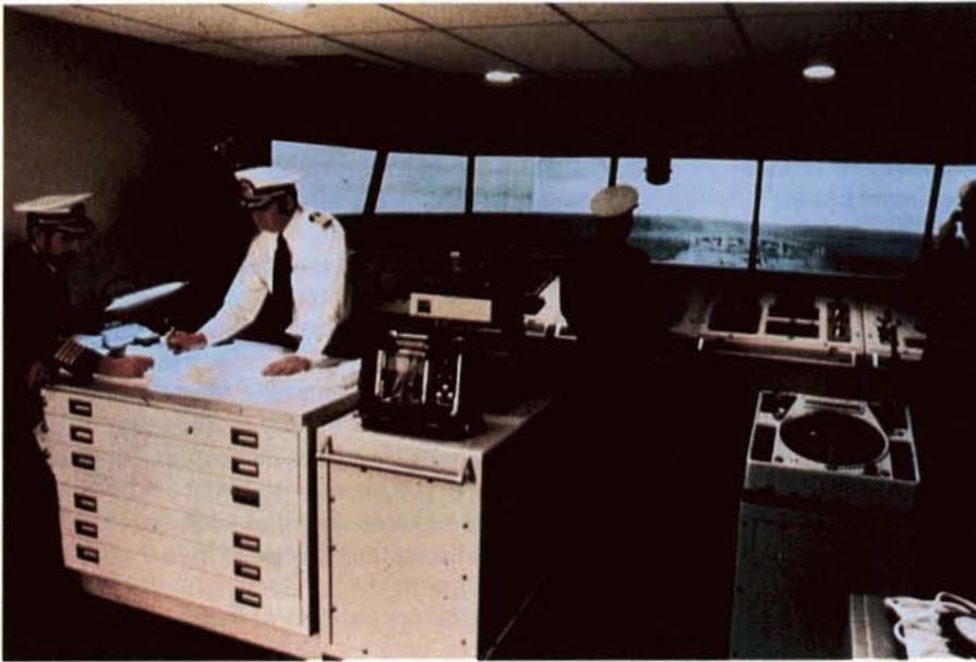
A companion system to CAORF is the Sperry Shiphandling Simulator, similar in operation and capability but designed for training where CAORF is used as a research tool. Located at New York's LaGuardia Airport, the Shiphandling Simulator is operated by Marine Safety International, Inc., a commercial firm which trains deck officers for shipping companies.
