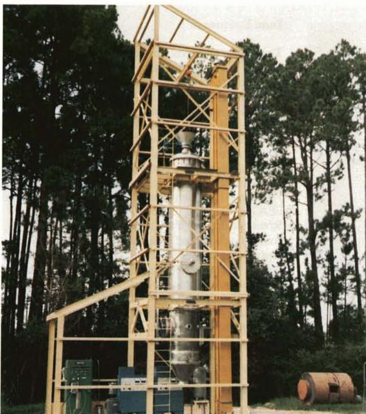
Successful initial crop drying experiments led to development of the Microwave Vacuum Drying System (MIVAC). At left is an interior view. The long cylinder is the vacuum chamber; wet crops enter through the top funnel and emerge dried through the exit hatch near bottom. At surface level is the microwave generating equipment.
