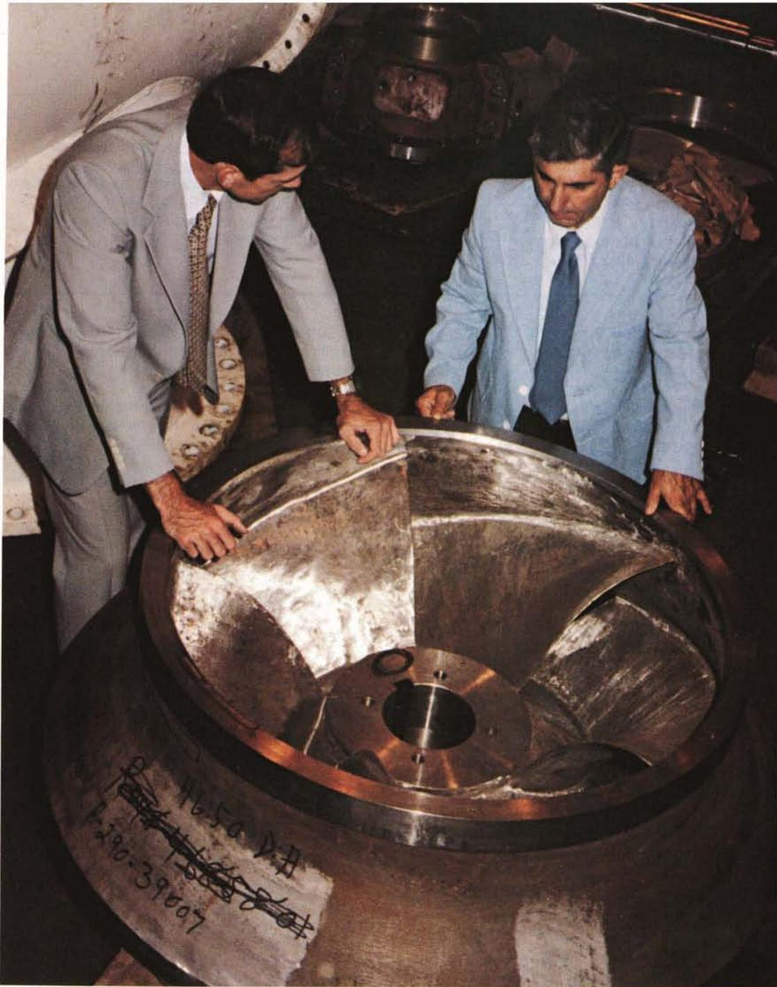
COSMIC-supplied computer program known as MERIDL. The program makes flow analysis calculations that permit designers to evaluate the performance and efficiency characteristics that can be expected from the pump's impeller. MERIDL also provides information that enables a trained hydraulic engineer to make design improvements.
