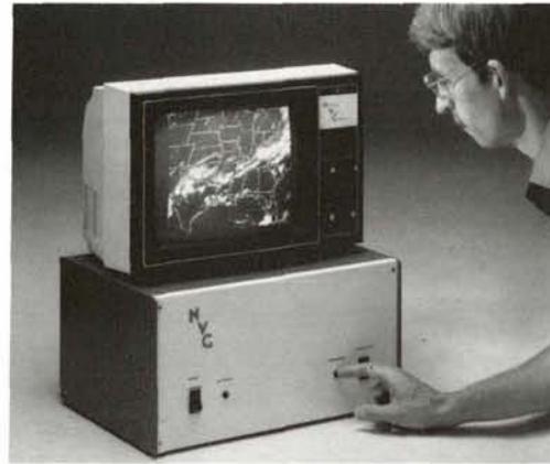
Video Fax consists of a two-meter diameter antenna (below) whose design is based on technology developed by Goddard Space Flight Center; a receiver; a microprocessor-controlled display computer; and a video monitor (above). The computer stores data from the satellites and converts it to an image which is displayed on the monitor. The weather map can be preserved as signal data on tape or it can be stored in a video cassette as a permanent image.
