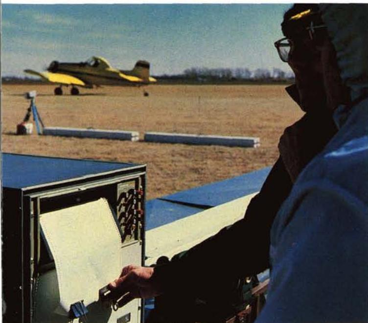
of nozzles. In the latter case, the applicator can make on-the-spot adjustments (right) and recheck his pattern. Other users of the OSU system include agricultural aircraft manufacturers seeking to develop or improve dispersal systems for their aircraft.
