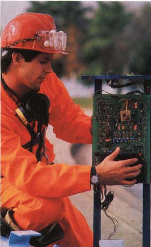
*A technician checks out the electronic circuitry of the QuadraScan sewer monitor. An individual monitor continually measures water depth at a particular location in a sewer; a number of monitors, each reporting its findings to a central computer, provides information important to city managers on overall sewer flow, flow in any section of the city, location and severity of leaks and warning of potential overload.*
