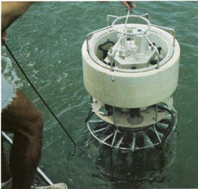
The monitor demonstrated its ability to provide voluminous water quality data in a seven-day field test at Saginaw Bay, an eastern Michigan arm of Lake Huron. In these tests, the system used only one-third of its battery energy supply, indicating that it could function well beyond the design goal of two weeks. On completion of the field tests, the monitor was turned over to EPA's Large Lakes Research Station, Grosse Ile, Michigan.
