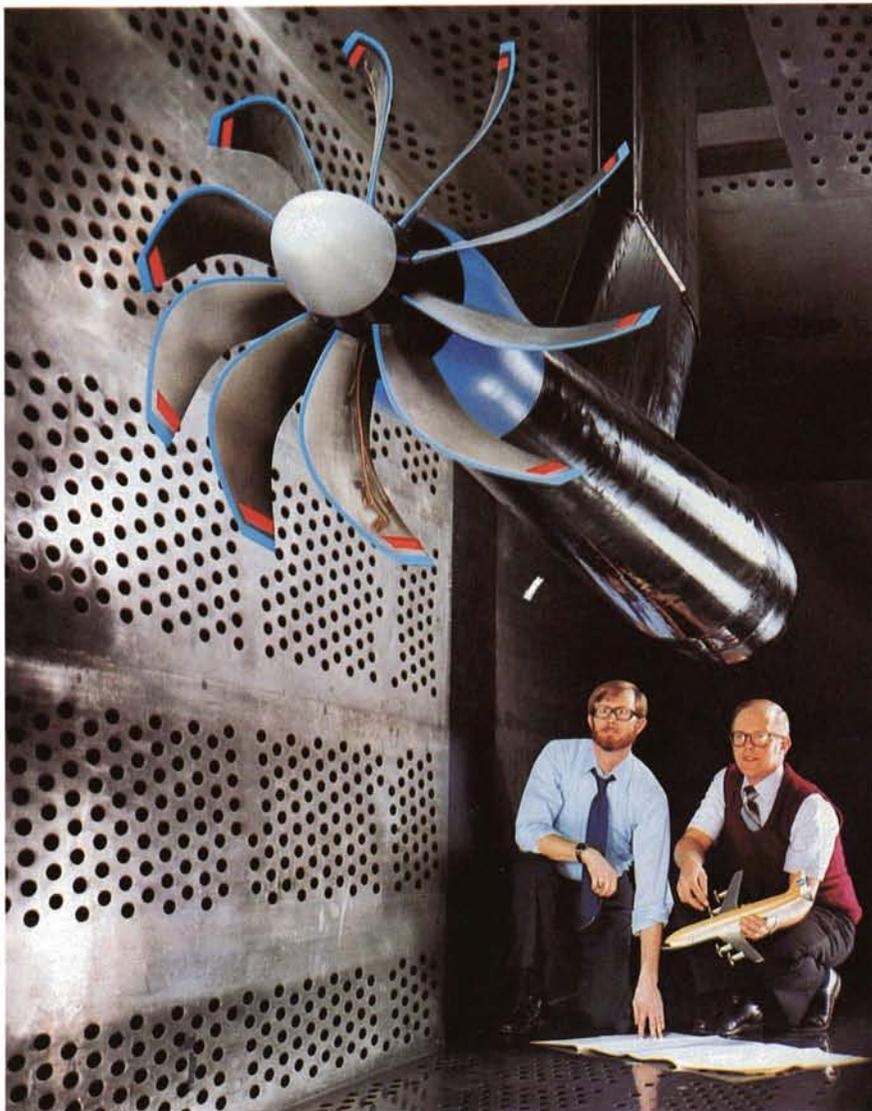
*This is a wind tunnel test model of an advanced turboprop featuring multiple swept-tip propeller blades. Research indicates that redesigned turboprops can drive transport aircraft at jetlike speeds with sharply reduced fuel consumption.*
