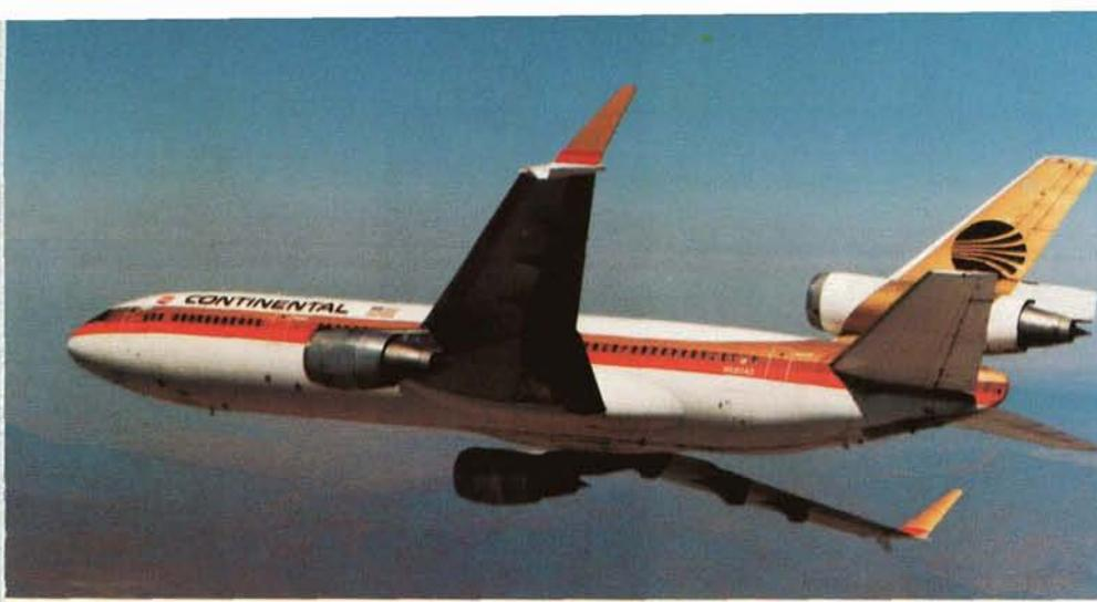
*Shown undergoing evaluation aboard a McDonnell Douglas DC-10, NASA-developed winglets reduce drag and save fuel by smoothing air turbulence that builds up at the wingtips of a high speed airplane.*
