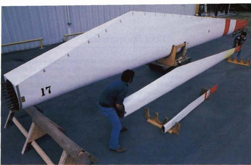
The large blade in the picture is a 60-footer developed for NASA; the smaller blades are Gougeon products manufactured for commercial wind turbines that provide electricity for homes, farms, apartment complexes and small utilities.
