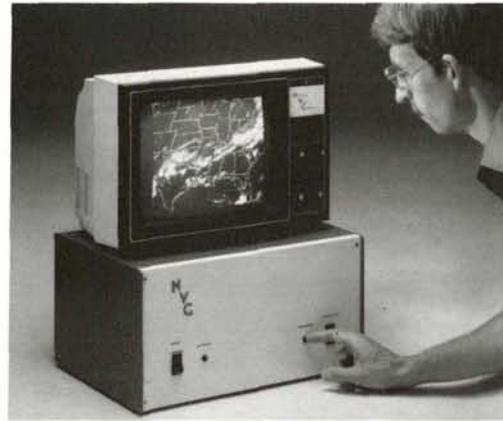
Video Fax consists of a two-meter diameter antenna (below) whose design is based on technology developed by Goddard Space Flight Center; a receiver; a microprocessor-controlled display computer; and a video monitor (above). The computer stores data from the satellites and converts it to an image which is displayed on the monitor. The weather map can be preserved as signal data on tape or it can be stored in a video cassette as a permanent image.
