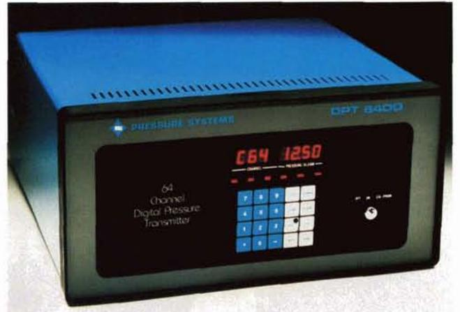
plant's process control computer. The DPT 6400 serves that function; by employing solid-state pressure-sensing transducers whose errors are automatically corrected by a microprocessor, it is capable of highly accurate pressure measurements; above, the digital reading (in red) indicates the channel number and the pressure, in pounds per square inch, at the loop being sensed. The basic DPT 6400 has 64 channels, but the system can be expanded to 256 channels by addition of "slave" units.
