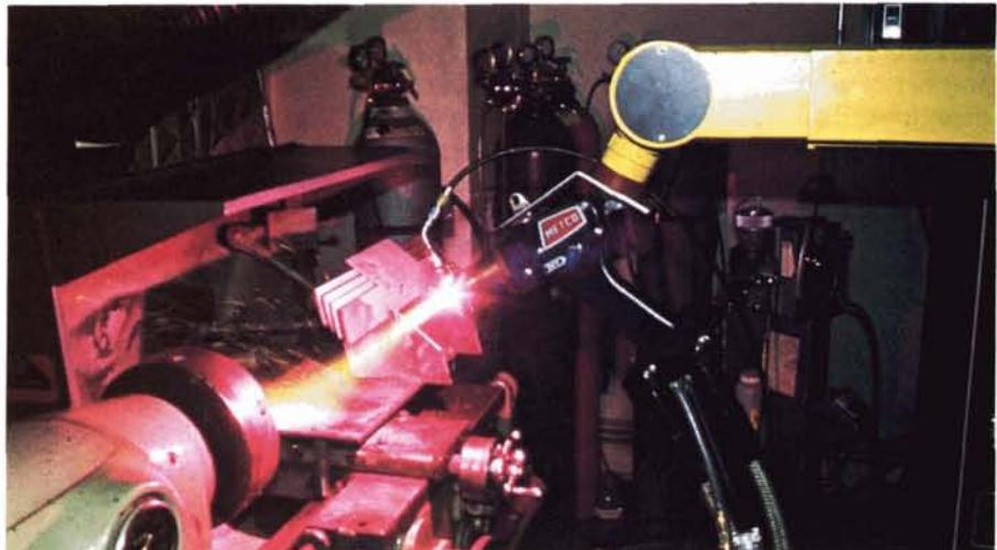
**Ceramic research is one area of NASA/Deere cooperation; Deere is testing ceramics to determine their impact on the drag and wear resistance of tillage equipment. Here a robotic arm is spraying hot ceramic onto a tool at the John Deere Technical Center.**
