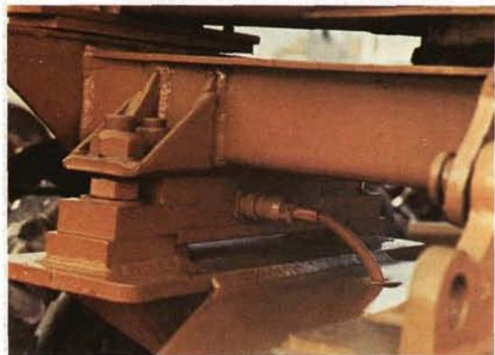
Shown above is a LODEC load cell (bar with connector attached) that supports the bridgebeam on a logging trailer. Within the load cell, tiny strain gages (at right below) sense and measure the increased weight as logs are added to the trailer. An indicator in the cab of the truck (center photo) converts signals from the load cell into weight information and displays it to the driver.
