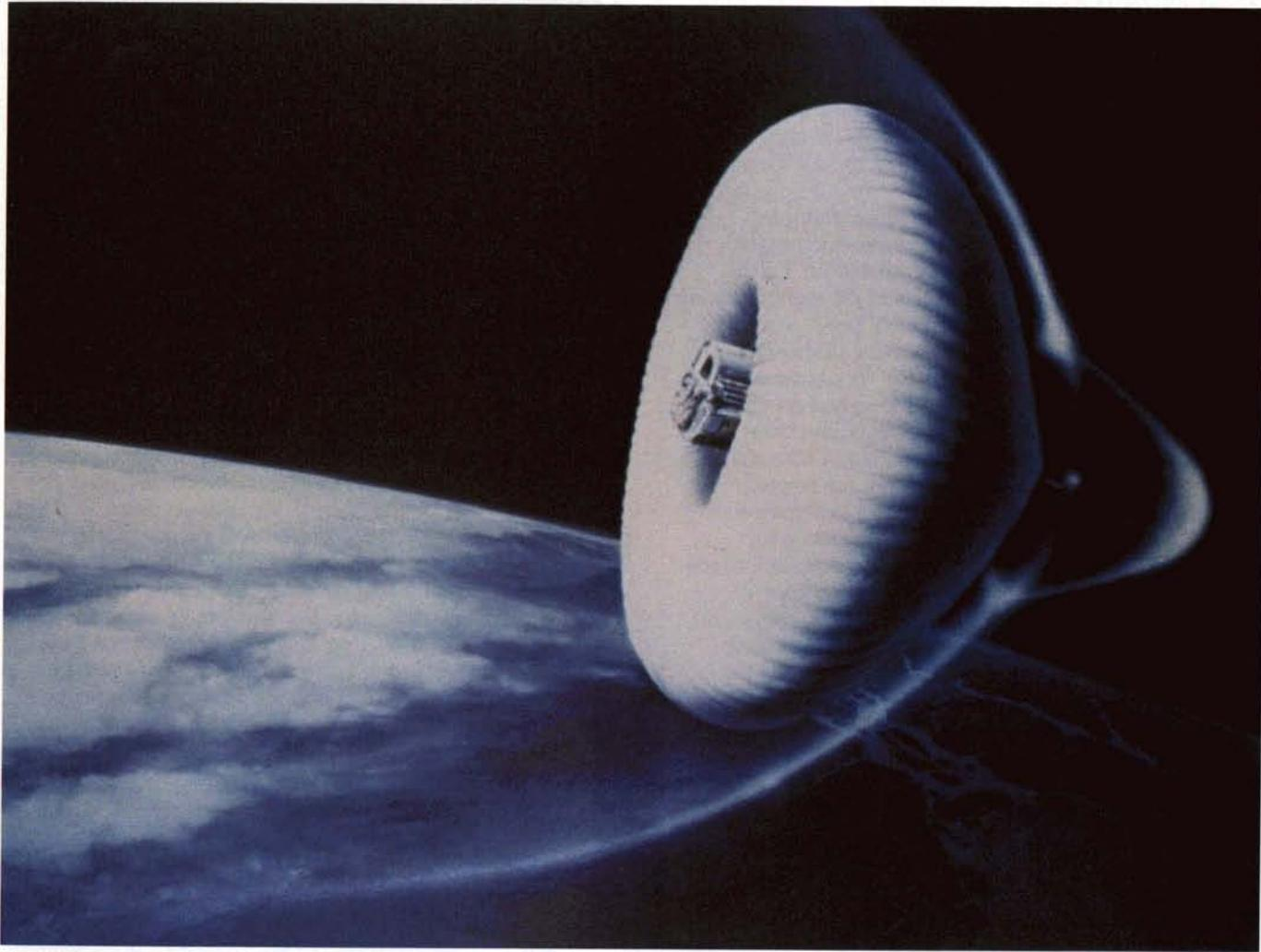
the payload is deployed from the Shuttle Orbiter in low Earth orbit (LEO), then boosted to higher altitude by unmanned upper stage propulsion units. Existing upper stages, however, are not reusable, nor can they retrieve satellites from GEO.
