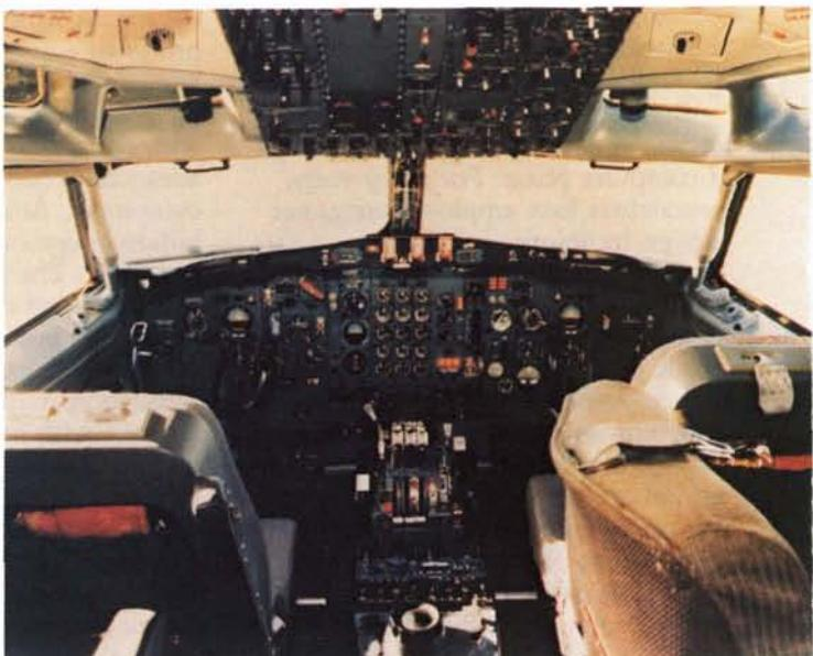
large numbers of interactive aircraft in a given airspace on different headings and at different speeds and altitudes. This simulation permits evaluation of new three-dimensional cockpit displays of traffic information (CDTI) jointly developed by NASA and the FAA. Tests are aimed at determining how quickly and accurately aircrews respond to CDTI displays and what improvements might be incorporated in the displays.
