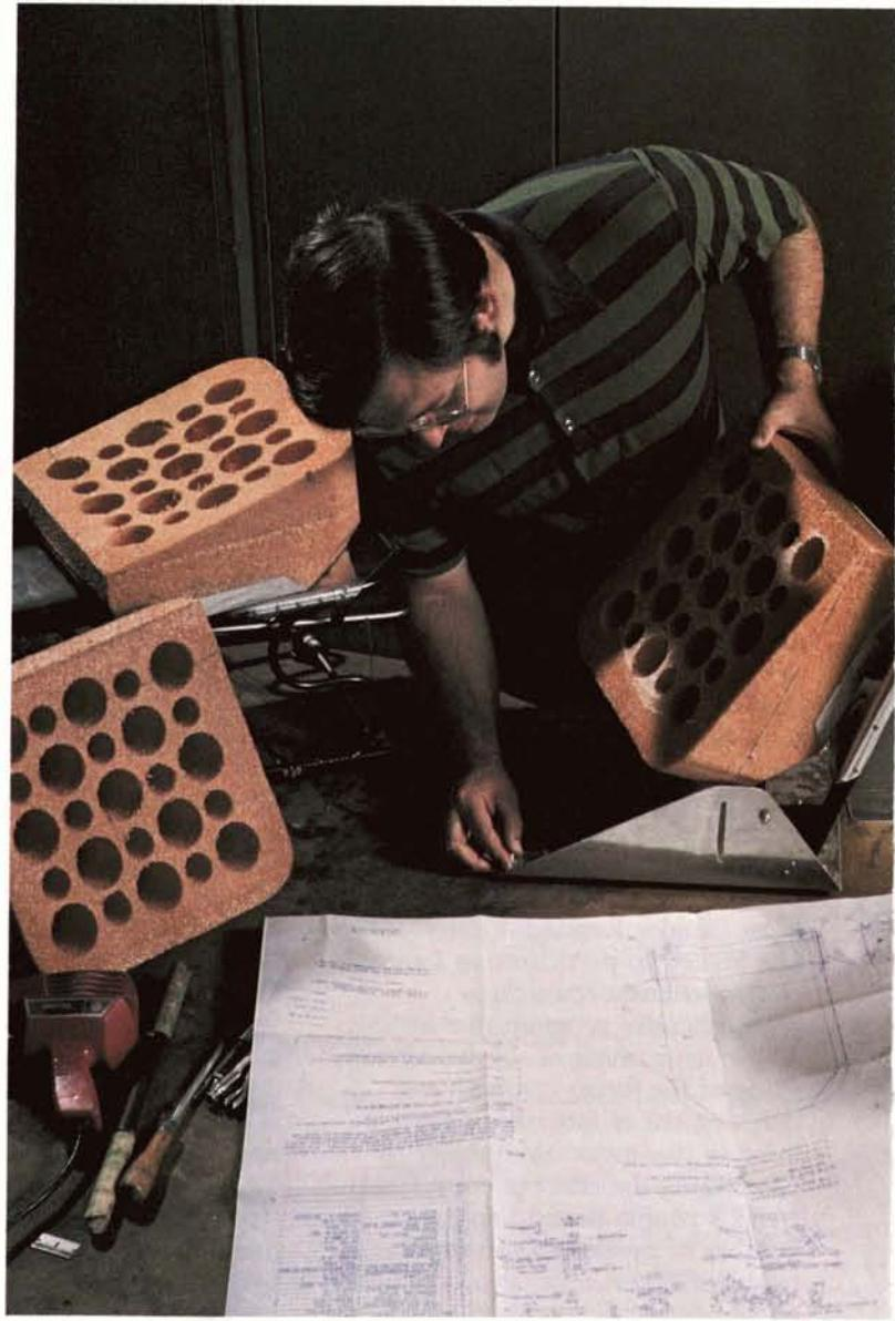
Additional crash protection is provided by installing a special type of impact absorbing foam block over a solid metal seat pan. The holes drilled in the foam block are another way of reducing crash impact.
