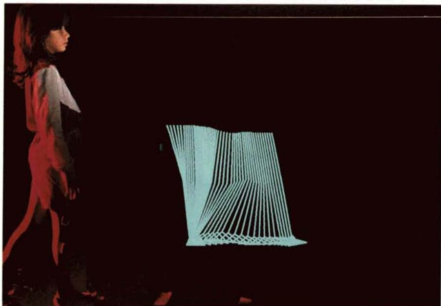
The motion Analysis Laboratory of Children's Hospital at Stanford is conducting tests of walking impaired children to study muscle movement as an aid to prescribing treatment. The laboratory uses a telemetry system to measure the degree and location of abnormal muscle activity. Leg sensors, shown at far right, send wireless signals to a computer, which develops pictures of gait patterns for use by physicians and therapists.
