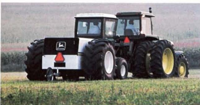
**The Dyna-Cart (above) was developed by Deere engineers to help them measure the effects of ballasting, tire slippage and other factors on fuel efficiency. Technical Center scientists are also studying the properties of alternative fuels (right) that may power future products.**
