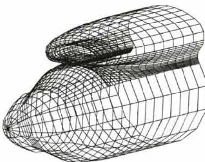
**The above illustration is a computer-generated drawing of an engine nacelle for an advanced turboprop aircraft design investigated by Lockheed-Georgia Company. The initial drawing has hundreds of extra lines, because the computer shows all the lines resulting from its stored input without regard for perspective. A new NASA-developed computer program automatically removes the hidden lines to produce clean, unambiguous drawings like the one below.**
