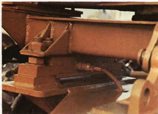
Shown above is a LODEC load cell (bar with connector attached) that supports the bridgebeam on a logging trailer. Within the load cell, tiny strain gages (at right below) sense and measure the increased weight as logs are added to the trailer. An indicator in the cab of the truck (center photo) converts signals from the load cell into weight information and displays it to the driver.
