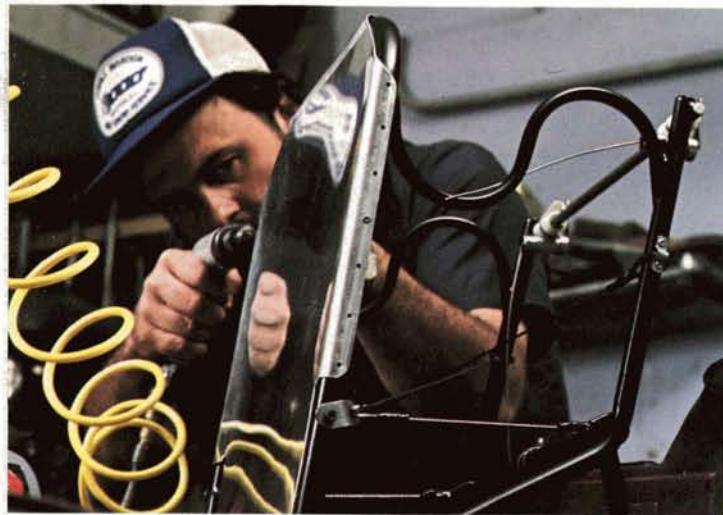
At its Waxhaw, North Carolina maintenance facility, JAARS is modifying each of the aircraft in its fleet to incorporate an innovative safety seat, designed by the Service with NASA research and testing help. In the above photo, a technician is working on a key feature of the JAARS seat: the "S-frame," in which S-shaped front legs absorb much of a crash impact so that substantially less force is transmitted to the occupant.
