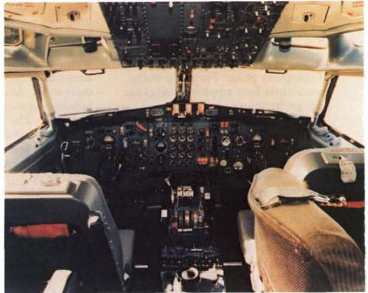
large numbers of interactive aircraft in a given airspace on different headings and at different speeds and altitudes. This simulation permits evaluation of new three-dimensional cockpit displays of traffic information (CDTI) jointly developed by NASA and the FAA. Tests are aimed at determining how quickly and accurately aircrews respond to CDTI displays and what improvements might be incorporated in the displays.
