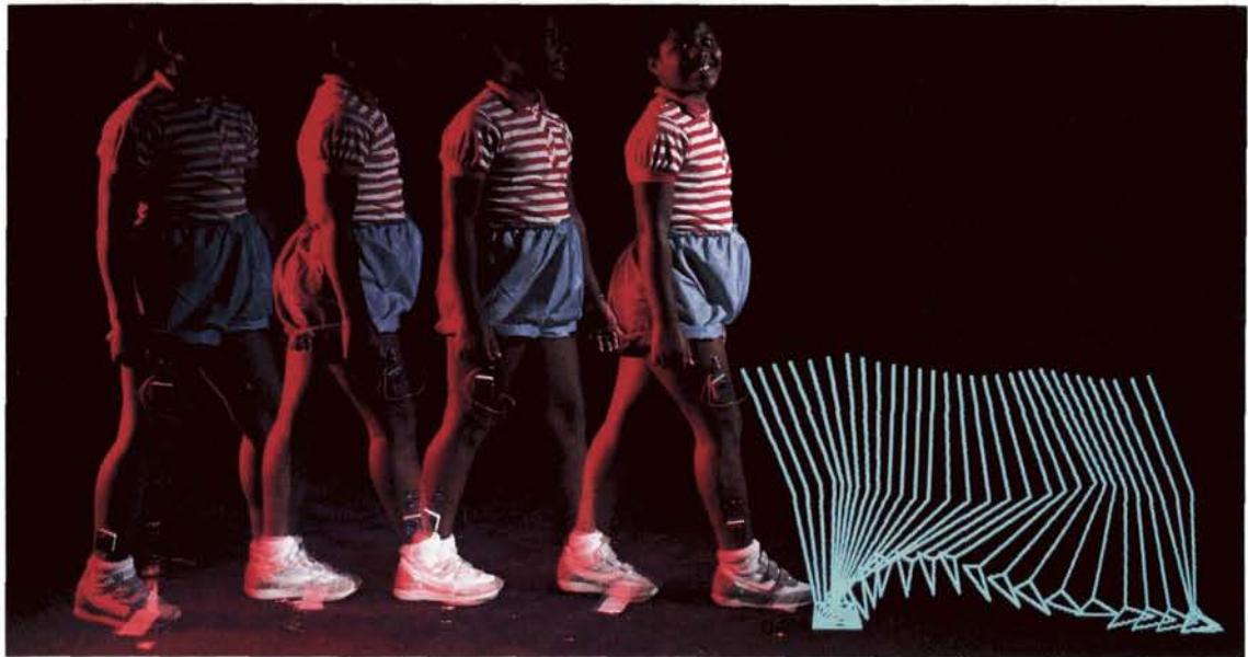
transmitters, each about the size of a half dollar, are affixed directly over the muscle group being studied. Each transmitter has its own tiny lithium battery and a pair of sensing electrodes. The muscle activity sensed—called an EMG, for electromyogram—is sent to a computer for analysis and display.
