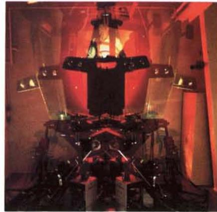
**In Deere's new human factors laboratory, engineers study how vibration and noise can affect the performance of a vehicle operator.**
