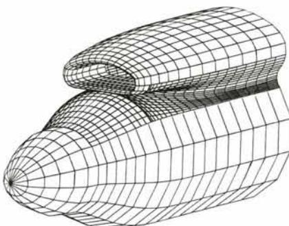
accurate method of simulating wing aerodynamics by computer. In 1981, after two years of effort, he came up with a computer program that considers whether a line in a graphic model of a three-dimensional object should or should not be visible. Known as the Hidden Line Computer Code, the program automatically removes superfluous lines and permits the computer to display an object from a specific viewpoint, just as the human eye would see it.
