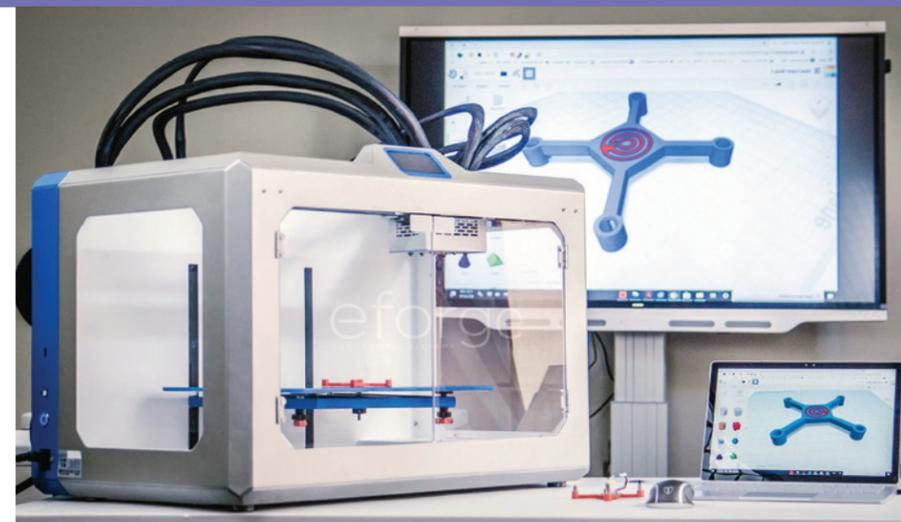
Electronic Alchemy developed the eForge 3D printer with NASA STTR and SBIR funding. The space agency was interested in 3D printing electronics in orbit and beyond.
