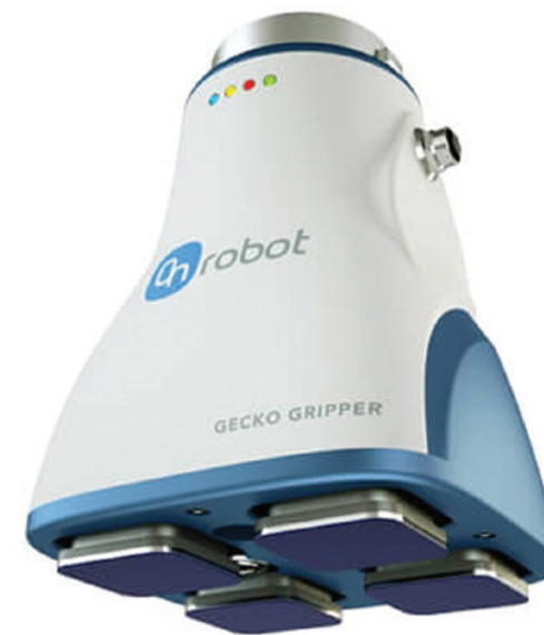
The Gecko Gripper, based directly on technology developed by NASA and Stanford University, is now available for manufacturing facilities, where it can move circuit boards, solar panels, and many other smooth objects more easily than traditional grippers. Credit: OnRobot A/S
