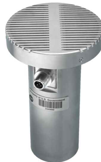
Qamar Shams and Allan Zuckerwar at Langley Research Center designed a special infrasound microphone that could pick up the ultralow frequencies generated by turbulence in the skies. This technology is now being tested on the Stratodynamics HiDRON glider for both turbulence detection and aeronautical research. Credit: NASA
