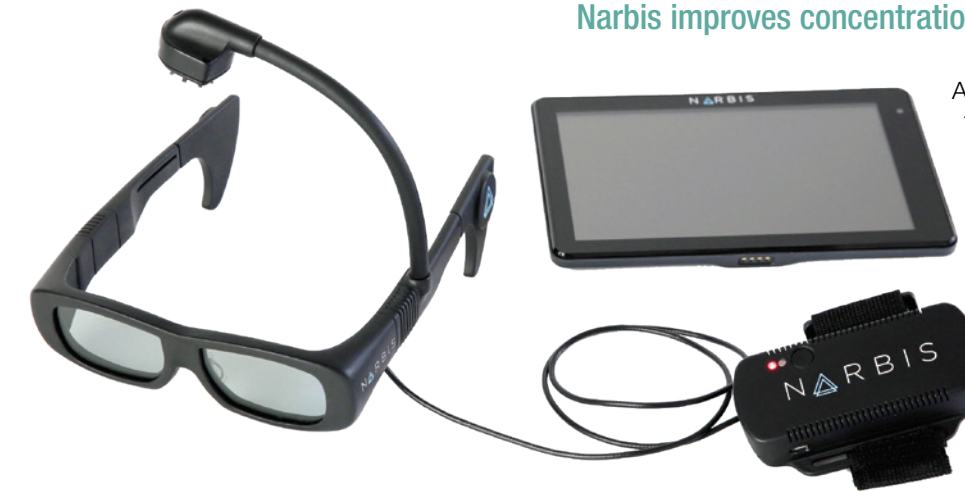
The Narbis smart glasses set includes the glasses, equipped with three brainwave sensors; a Bluetooth-enabled amplifier on an armband; and a tablet with training programs. Credit: Narbis
