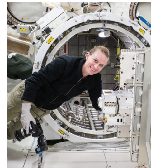
The Nanoracks LLC Bishop Airlock Module that was added to the space station has five times the capacity of the one other airlock currently in use on the station. The Japanese airlock (left) used to launch CubeSats is much smaller than Bishop (right). The privately funded airlock can accommodate significantly more satellites and autonomous experiments. Credit: NASA/Nanoracks
