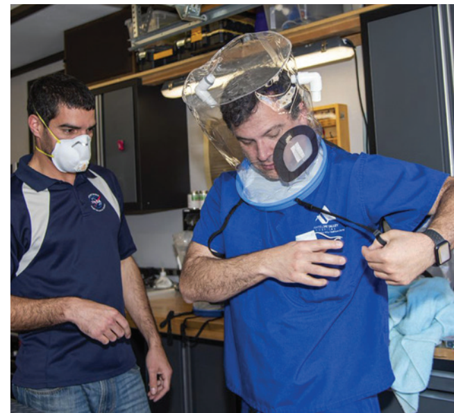
Armstrong Flight Research Center engineer Mike Buttigieg, left, led a team that came up with a low-cost oxygen helmet for COVID-19 patients. The design includes a magnetically sealed port, which the center has licensed out. Here, Dr. Daniel Khodabakhsh of Antelope Valley Hospital tries one on. The hospital was part of a task force that helped with the effort. Credit: NASA
