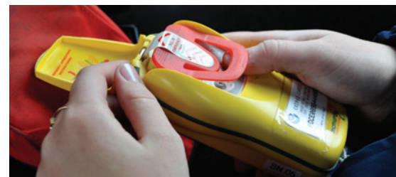
Medium-Earth orbit satellites added to the SARSAT system over the last decade or so have dramatically reduced the time it takes to respond to signals from emergency beacons like this one. Credit: U.S. Coast Guard
