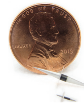
Created with the help of SBIR funding, the ferrite cores inside a Micro Harmonics isolator are small enough to be used in both sensors on satellites and instruments on the ground. Credit: Micro Harmonics
