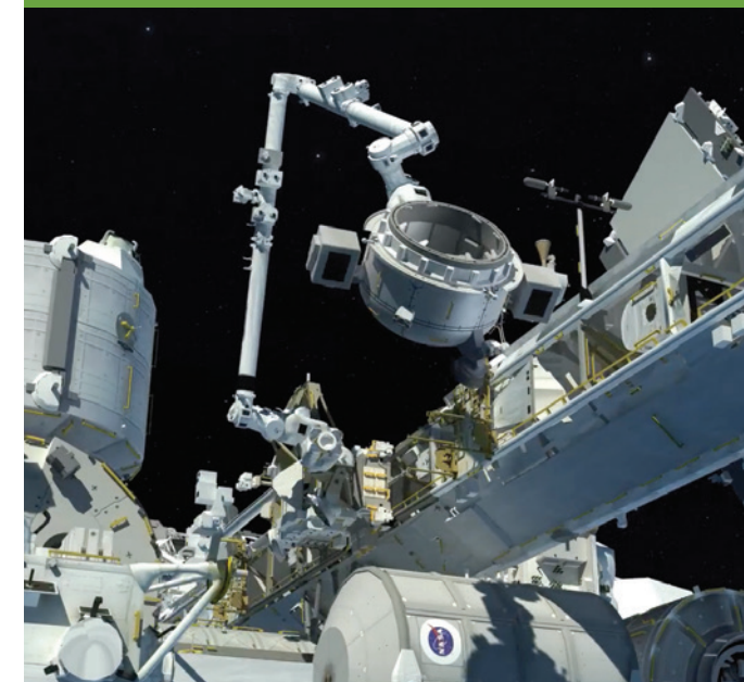
The Nanoracks Bishop Airlock can be attached to Node 3 and opened to space to release satellites and run experiments. It can also be detached and moved to different locations. Taking advantage of the opportunity to expose experiments to different elements such as sunlight or atomic oxygen, this flexibility enables a wide range of research possibilities. Credit: Nanoracks
