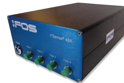
An Intelligent Fiber Optic Systems (IFOS) Multi-Channel Interrogator takes readings from micro-holograms etched into optical fibers and translates it into data. Credit: Intelligent Fiber Optic Systems Corporation
