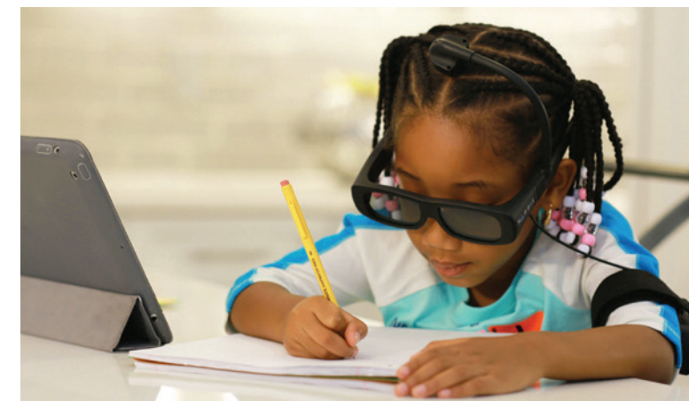
Narbis glasses train the user to focus by darkening when attention wanders and clearing up when focus resumes. They can be used while performing virtually any task. Credit: Narbis
