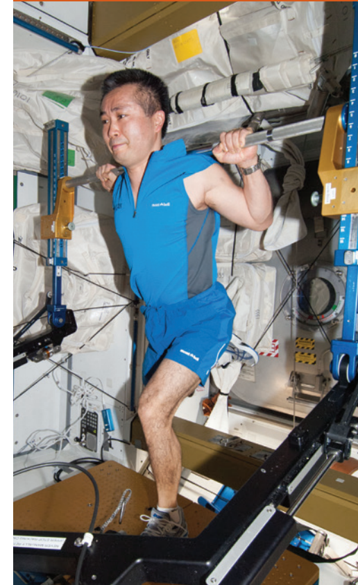
Japanese Aerospace Exploration Agency astronaut Koichi Wakata works out on the Advanced Resistive Exercise Device (ARED) on the space station. Maintenance procedures for the ARED have been digitized to work with the ProX virtual reality guidance technology developed by Tietronix Software Inc. Credit: NASA
