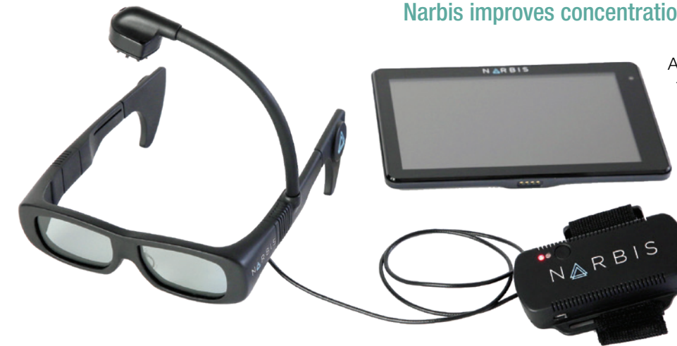
The Narbis smart glasses set includes the glasses, equipped with three brainwave sensors; a Bluetooth-enabled amplifier on an armband; and a tablet with training programs. Credit: Narbis
