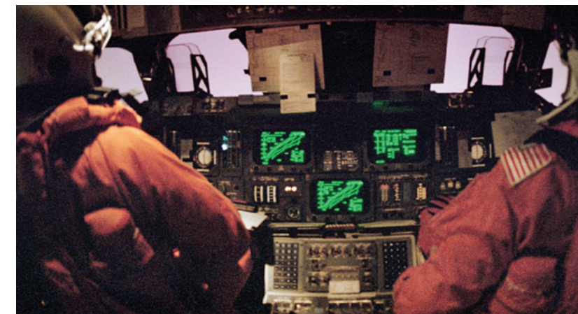
This cabin view of the space shuttle during STS-42 reentry shows the color of atmospheric plasma. Due to the compression and friction of the air, the molecules generate a very hot plasma which glows in the red-orange spectrum. NASA conducts tests on the heat shield and materials on spacecraft to make sure they'll deflect the damaging heat. InEnTec used some of the agency's research to design a plasma-assisted gasification process. Credit: NASA
