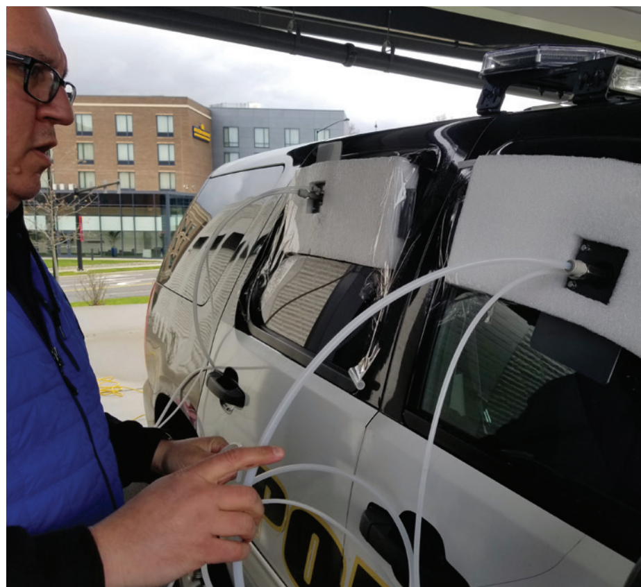
Jason Thompson of EP+R tests a new system that lets the AMBUstat G2 fogging device quickly sterilize small spaces, like the inside of a police car. Credit: Emergency Products and Research
