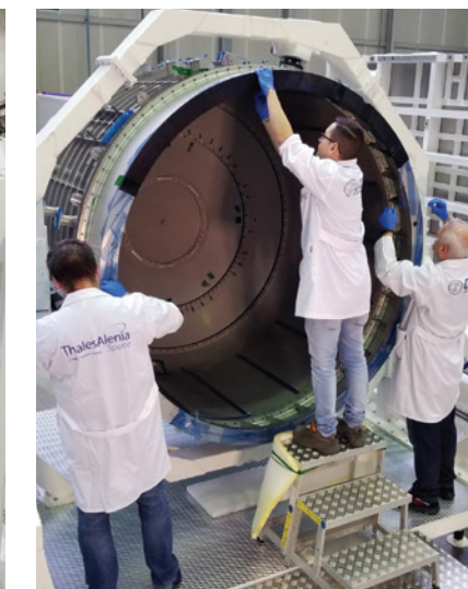
The Nanoracks LLC Bishop Airlock Module that was added to the space station has five times the capacity of the one other airlock currently in use on the station. The Japanese airlock (left) used to launch CubeSats is much smaller than Bishop (right). The privately funded airlock can accommodate significantly more satellites and autonomous experiments. Credit: NASA/Nanoracks
