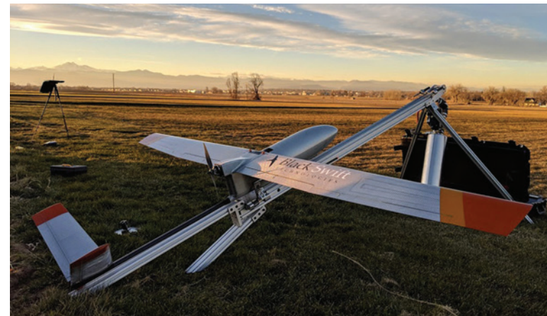
The S2 is a remotely piloted vehicle that uses a modular design for easy sensor replacement in the field. Designed to meet NASA atmospheric measurement needs, the drone, made by Black Swift Technology Inc., is now used by universities for research and by industry for site surveys and more. Credit: Black Swift Technologies Inc.
