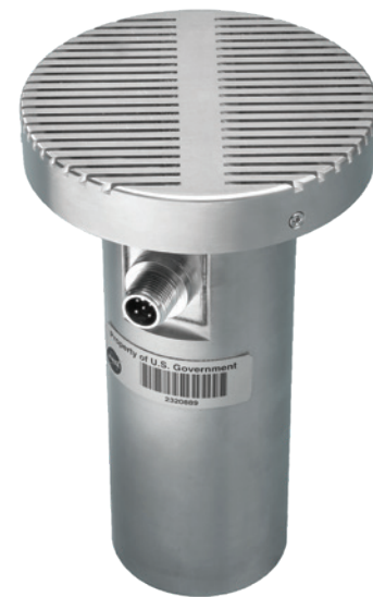
Qamar Shams and Allan Zuckerwar at Langley Research Center designed a special infrasound microphone that could pick up the ultralow frequencies generated by turbulence in the skies. This technology is now being tested on the Stratodynamics HiDRON glider for both turbulence detection and aeronautical research. Credit: NASA
