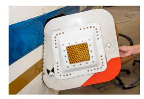
NASA designed a lightweight antenna using an aerogel that consisted primarily of air. The materials created flexible antennas with improved gain, bandwidth, and efficiency. The small, single unit combined 64 small antennas that outperformed the functionality of one large antenna, and it led to a new kind of aerogel created by Blueshift Materials, known as AeroZero. *Credit: NASA*
