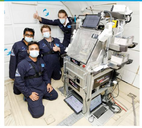
Space Foundry's Ram Prasad Gandhiraman, Dennis Nordlund, and senior engineers Pranay Doshi and Daniel Gutierrez testing the company's plasma 3D printing technology on a NASA-funded parabolic flight. Such flights create microgravity conditions without going to space. *Credit: Space Foundry*
