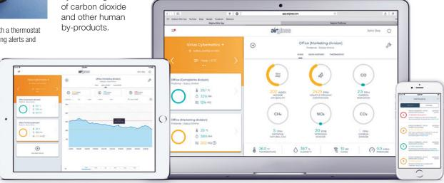
Airgloss sensors measure volatile organic compounds, carbon monoxide, carbon dioxide, nitrogen dioxide, methane, humidity, and even ambient noise and lighting to generate detailed reports that they deliver to devices via WiFi. Credit: Airgloss
