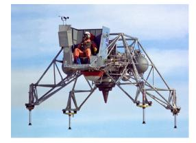
This 1967 NASA Lunar Landing Research Vehicle, similar to the Lunar Module used during Apollo missions, was a flying machine that replicated descent to the lunar surface. New navigation systems will make landings safer. *Credit: NASA*
