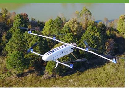
The Hybrid Advanced Multi-Rotor aircraft uses a small combustion engine paired with batteries and electric motors to achieve flight times far greater than those powered by batteries alone. Bill Fredericks credits his work with NASA on the Greased Lightning project for enabling its development. Credit: Advanced Aircraft Company
