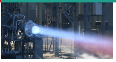
In this hot fire test at Marshall Space Flight Center, a nozzle printed from a NASA-developed superalloy metal is used inside the combustion chamber. The nozzle's surface was polished by Southington, Connecticut-based REM Surface Engineering, with a process and tools developed under SBIR funding from Marshall. *Credit: NASA*
