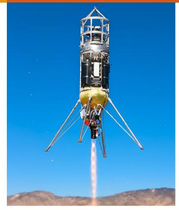
Technology for spaceflight requires testing on Earth. Masten Space Systems built Xodiac to test terrain-relative navigation and hazardavoidance systems for landings on Mars, the Moon, and more. *Credit: Masten*
