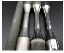
Building rocket parts using 3D printing is less expensive than traditional manufacturing methods and can facilitate complex shapes without joints. But the technique leaves rough surfaces (left) that could cause turbulence, corrosion, and accelerated wear if not perfectly polished (right). *Credit: NASA*
