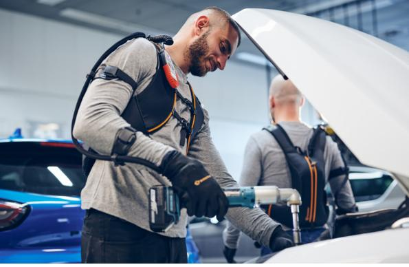
Swedish company Bioservo Technologies' Ironhand, based on a set of patents from NASA and GM's Robo-Glove, is the world's first industrialstrength robotic glove for factory workers and others who perform repetitive manual tasks. Credit: Bioservo Technologies/Niklas Lagström
