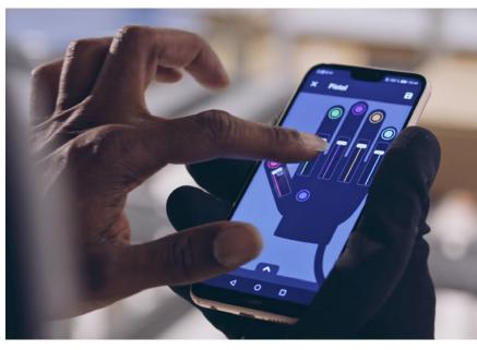
The Ironhand glove can be adjusted to user preferences and task-specific motions, with combinations of force, sensitivity, finger balance, and locking tendency saved as profiles and controlled with the IronConnect Pro app, shown here, or a remote control worn on the chest. Credit: Bioservo Technologies/Niklas Lagström
