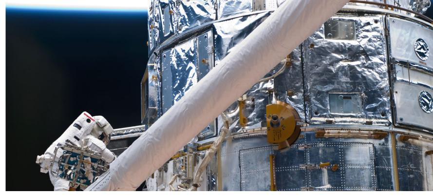
In May 2009, astronaut John Grunsfeld works on repairs to the Hubble Space Telescope, including replacing three thermal blankets protecting the telescope's electronics. This multi-layer reflective thin-film insulation, also known as radiant barrier, manages temperatures in almost all NASA spacecraft and spacesuits and is also one of the agency's most ubiquitous spinoffs, appearing in countless products, including new lightweight jackets from 13-One. Credit: NASA
