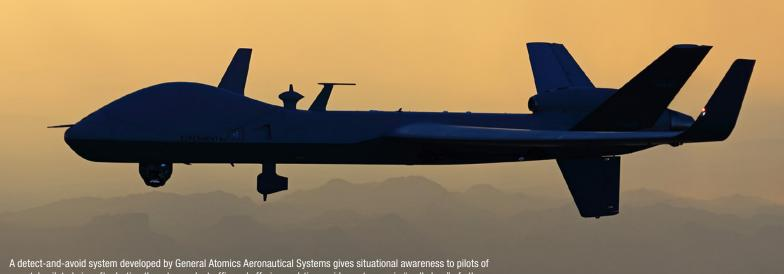
remotely piloted aircraft, alerting them to nearby traffic and offering real-time guidance to remain "well clear" of other aircraft. The system will fly on the company's newest remotely piloted aircraft, the MQ-9B SkyGuardian, pictured here. Credit: General Atomics Aeronautical Systems Inc.
