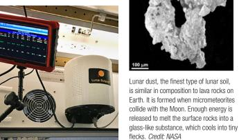
Ahead of future lunar missions, NASA wanted a sensor to act like a canary in a coal mine, warning inhabitants if the level of dust gets dangerous. Lunar Outpost developed the Space Canary, an air-quality sensor, shown here in a lunar habitat prototype designed by Lockheed Martin. Credit: Lockheed Martin Corporation
