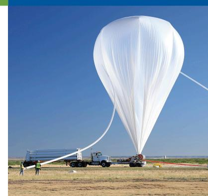
Miniaturized sensors that fly on a zero-pressure balloon collect data and take pictures that are as expansive as satellite images but are more precise. Denver-based Urban Sky leveraged SBIR funding from NASA to create sensors lighter than off-theshelf options.
