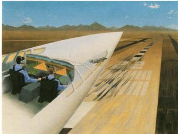
*Future jetliners may employ a design technique that eliminates forward-facing cockpit windows and substitutes a 3D computer-generated color display to give the pilots "synthetic vision" on takeoffs and landings. Already flight tested, this system could save thousands of pounds of weight that could be more productively used.*
