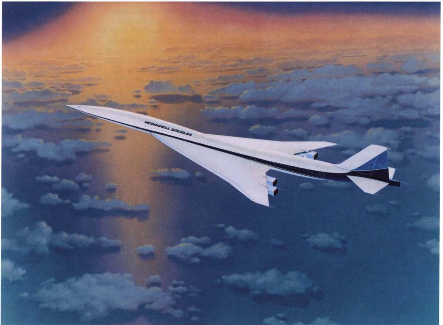
*This McDonnell Douglas conceptual design for a Mach 2.4 (1600 miles per hour) supersonic transport is sized to carry about 300 passengers over a distance of 5,000 nautical miles. A NASA/industry High Speed Civil Transport research effort is a first step toward determining whether such a plane can be economically viable and environmentally acceptable.*
