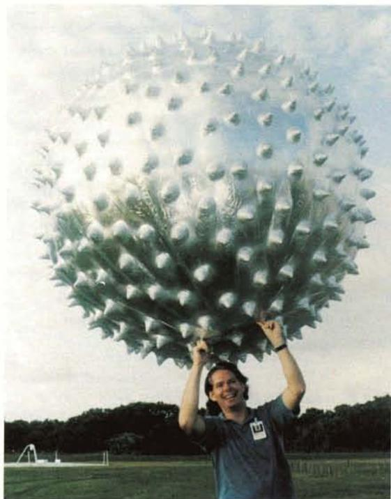
*The Jimsphere wind measurement balloon is made of lightweight radar-reflective materials.*
