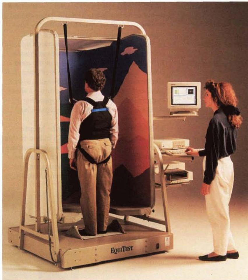
*Above: The EquiTest System evaluates balance under dynamic test conditions.*
