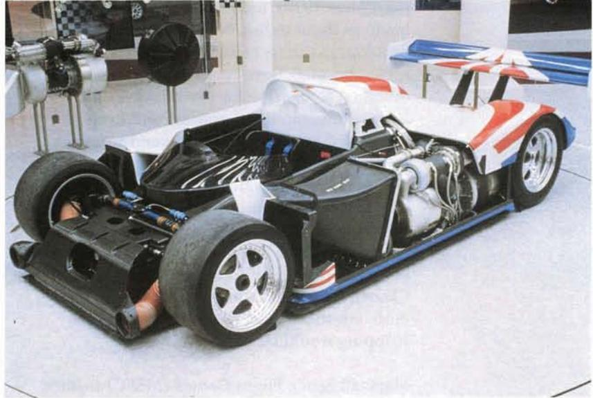
*Flywheel Energy Storage technology developed for NASA by SatCon Technology Corporation plays a role in the drive train of experimental hybrid-electric automobiles.*
