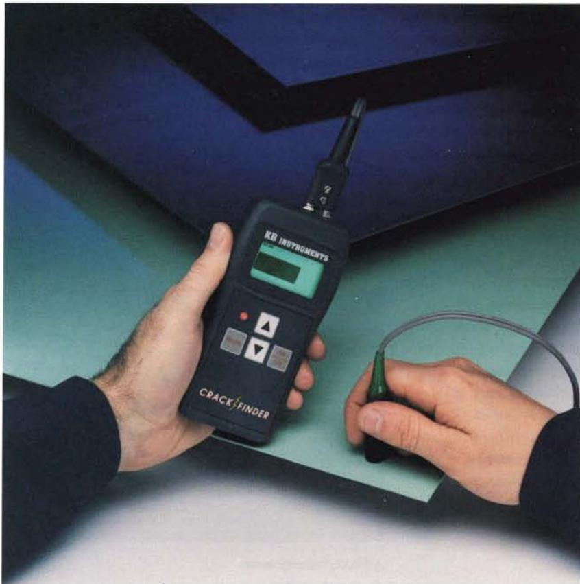
*Developed to scan aircraft skins for surface breaks, the CrackFinder is available for industrial use in fatigue detection.*
