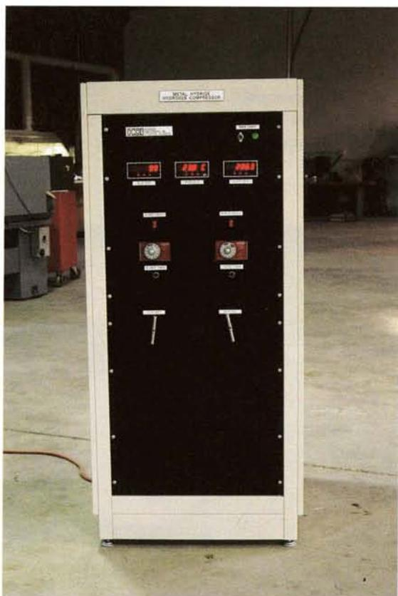
Among the properties of metal hydrides is their ability to store hydrogen in a solid state, an area that has not been widely exploited. Since hydrogen is a common spacecraft propellant, but difficult to store, NASA was interested in the potential of metal hydrides as a means of storing hydrogen in solid state and thus avoiding the hazards of compressed gas or the complexity and boiloff of liquid hydrogen.
