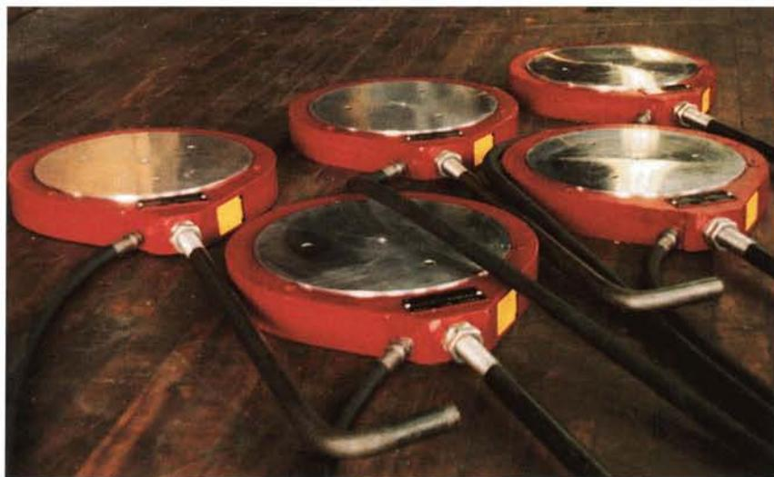
*A group of Dudgeon 700-ton load cells/hydraulic jacks, each of which weighs only 79 pounds.*
