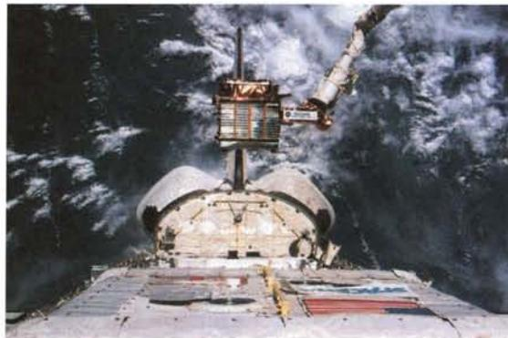
*This view of the Orbiter Endeavour's stern shows the Spartan 207 free flyer being recaptured after a day-long research trip away from the Orbiter. It is being jockeyed toward its stowage berth by an astronaut operating the remote manipulator system.*
