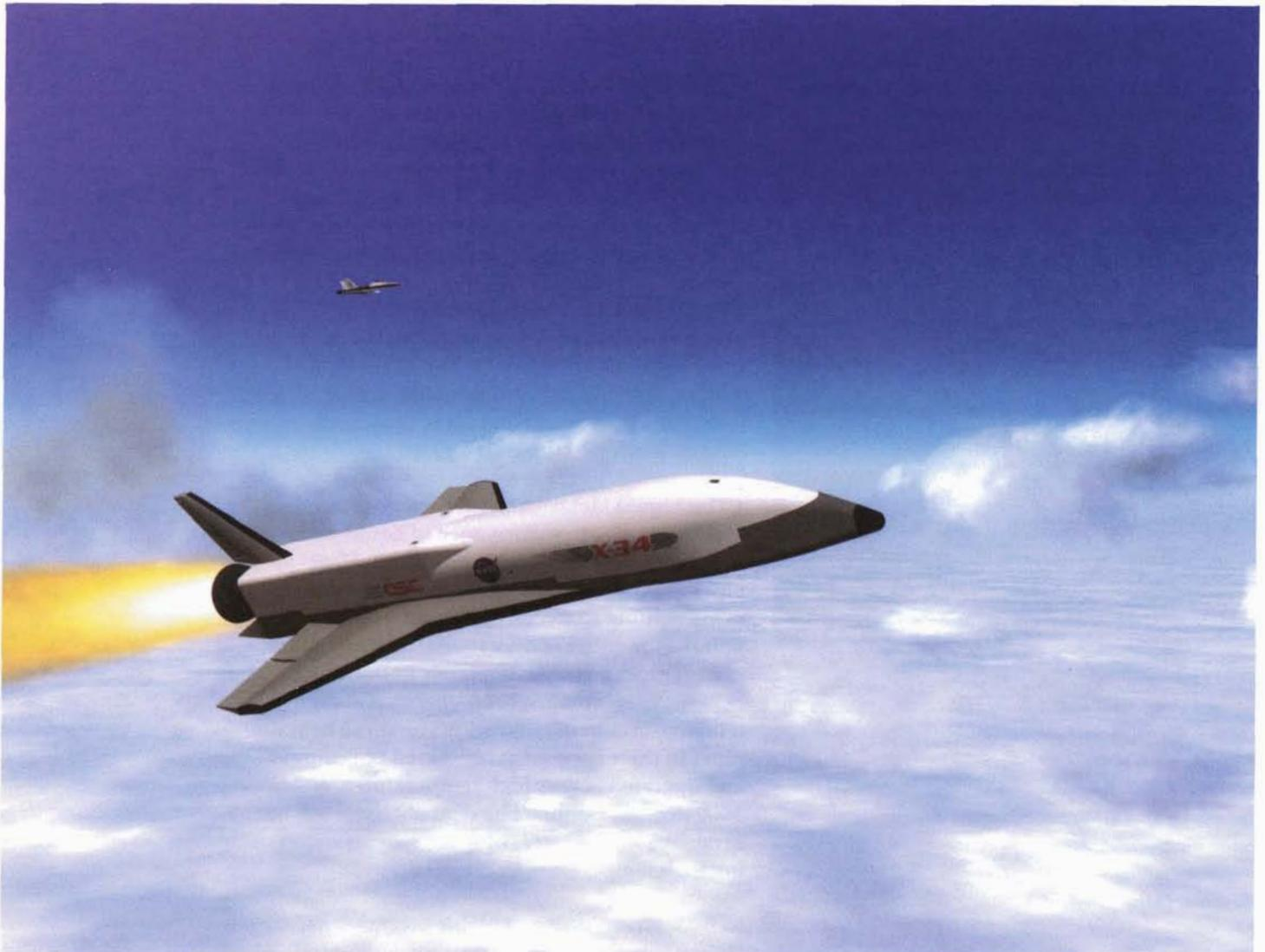
*Under development by Orbital Sciences Corporation is the X-34, an experimental vehicle for testing technologies for a single-stage-to-orbit launch vehicle. First flight is targeted for 1998.*
