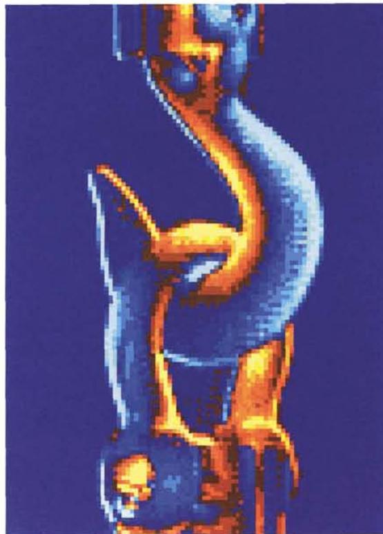
*Used in nondestructive evaluation of materials and structures, the system images temperature changes that correspond to dynamic stresses in a structure.*
