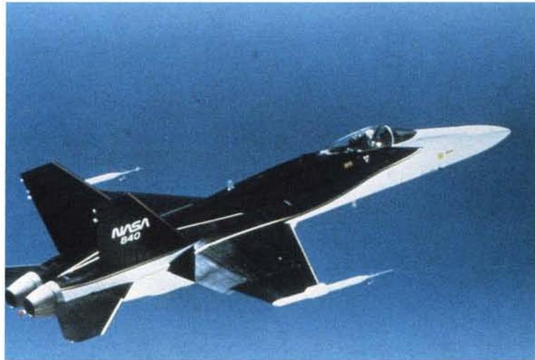
*NASA's veteran F-18 HARV research aircraft concluded a decade-long flight test program that explored aircraft maneuverability and controllability at high angles of attack.*
