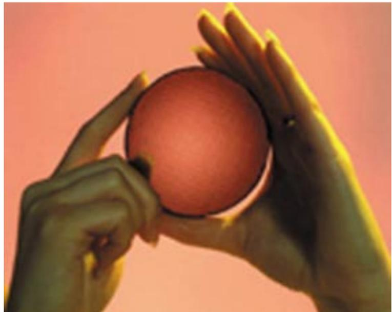
*STC Catalysts, Inc.'s catalyst has the ability to remove carbon monoxide and formaldehyde from the air in enclosed spaces.*
