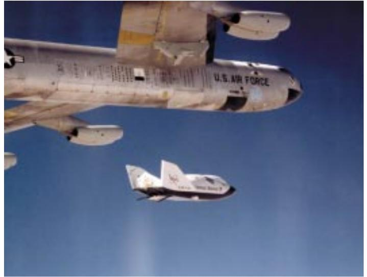
*The X-38 Crew Return Vehicle is released from high altitude, so the project team can conduct aerodynamic verification maneuvers, among other tests.*
