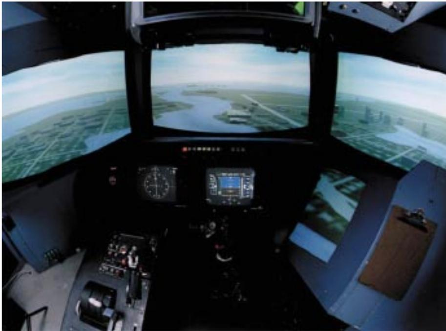
*The VMS is controlled by large digital computers that are programmed to represent the aircraft and the external environment.*
