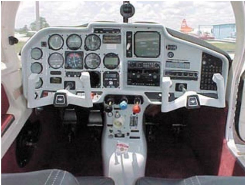
*Mod Works, Inc., has designed an instrument panel that offers features geared toward simplification in cockpit design.*
