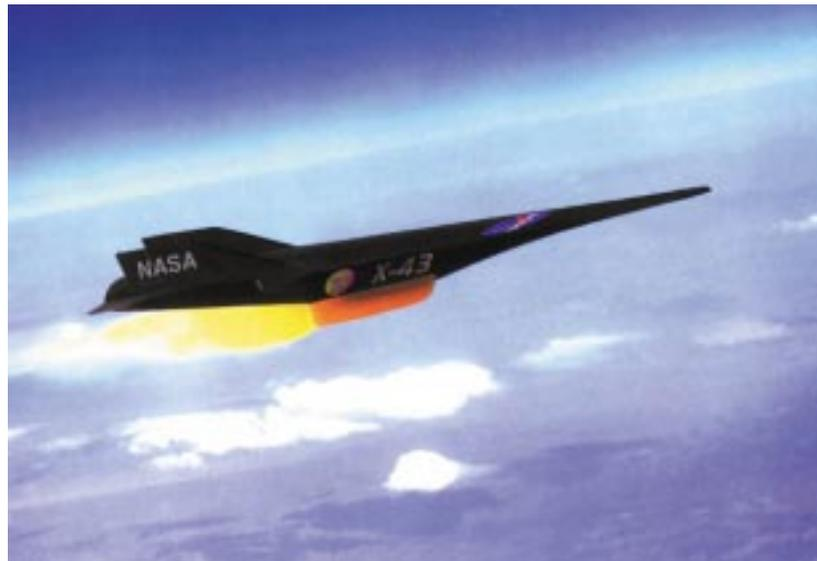
*Hyper-X program's X-43A vehicle is to be powered by air-breathing scramjet engine technologies, pushing the craft to 10 times the speed of sound.*
