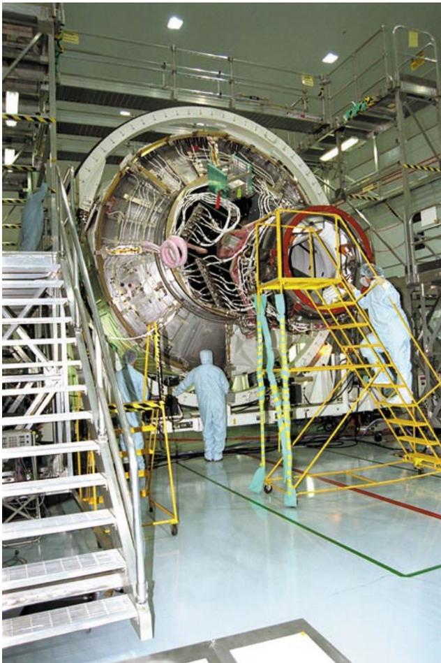
*Kennedy Space Center workers rotate the International Space Station's Node 1 and Pressurized Mating Adapter-1.*
