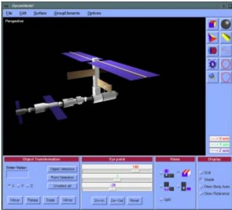
*Dynacs Engineering Company, Inc.'s Dycom is a multibody dynamics and control system simulation tool.*
