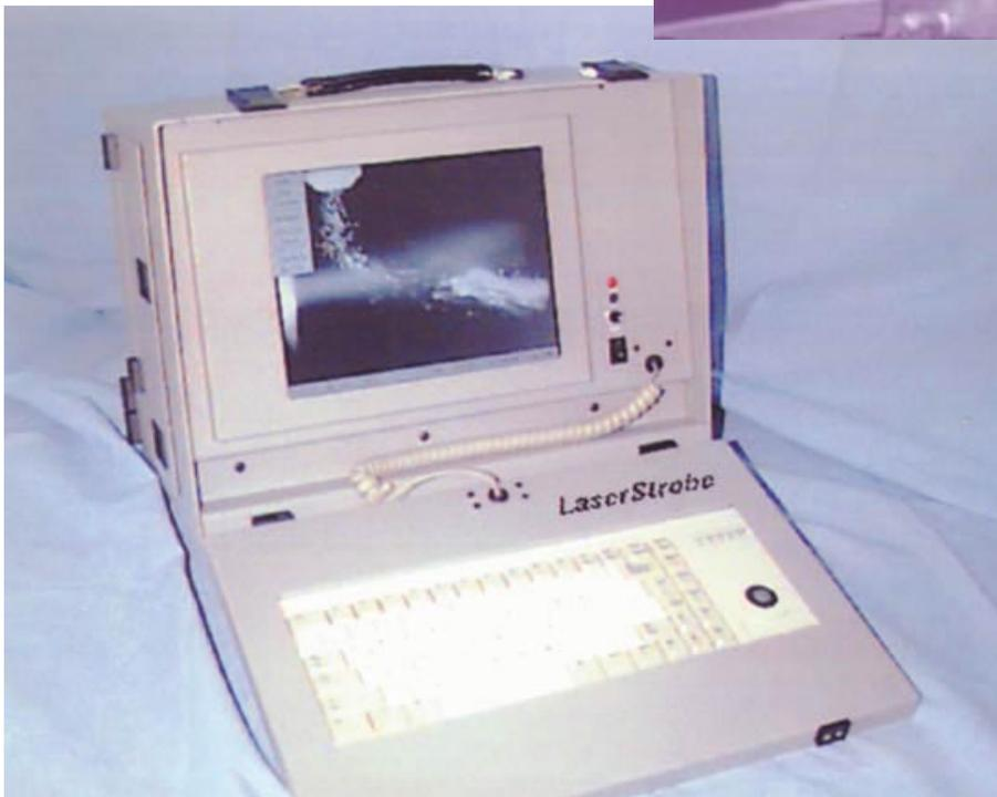
*Control Vision, Inc.'s LaserStrobe<sup>®</sup> and PyroCam<sup>®</sup> systems can yield high-resolution video images of high-energy industrial processes.*
