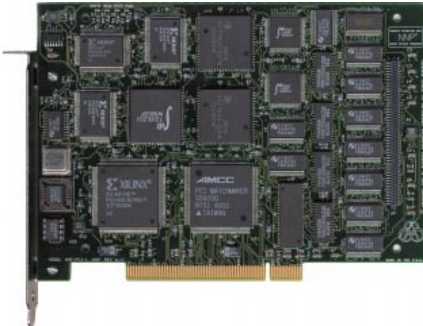
*Accurate Automation Corporation’s neural processor, the NNP<sup>®</sup>, was developed using the interconnectedness of the human brain as a model.*
