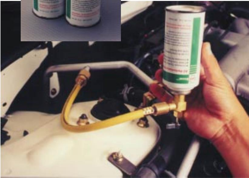
When production of ozone-depleting refrigerants was halted in the United States as part of the Environmental Protection Agency's Clean Air Act, affected units switched to another type of refrigerant. However, in doing so, these same units suffered a performance and efficiency reduction. Lower vapor-compression system efficiencies meant more electrical consumption resulting in the production of more power plant emissions.
