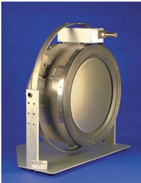
*Work in ion propulsion technology at Glenn Research Center made possible the technology validation flight of the Deep Space 1 spacecraft. The fuel-efficient ion engine was tested in space in 1998-1999, and is to be utilized on 21<sup>st</sup> century deep space missions.*
