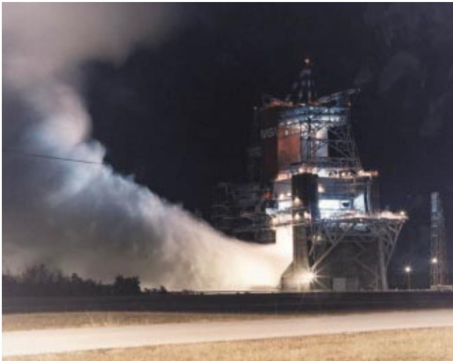
*A Space Shuttle Main Engine test lights up the night sky at Stennis Space Center.*
