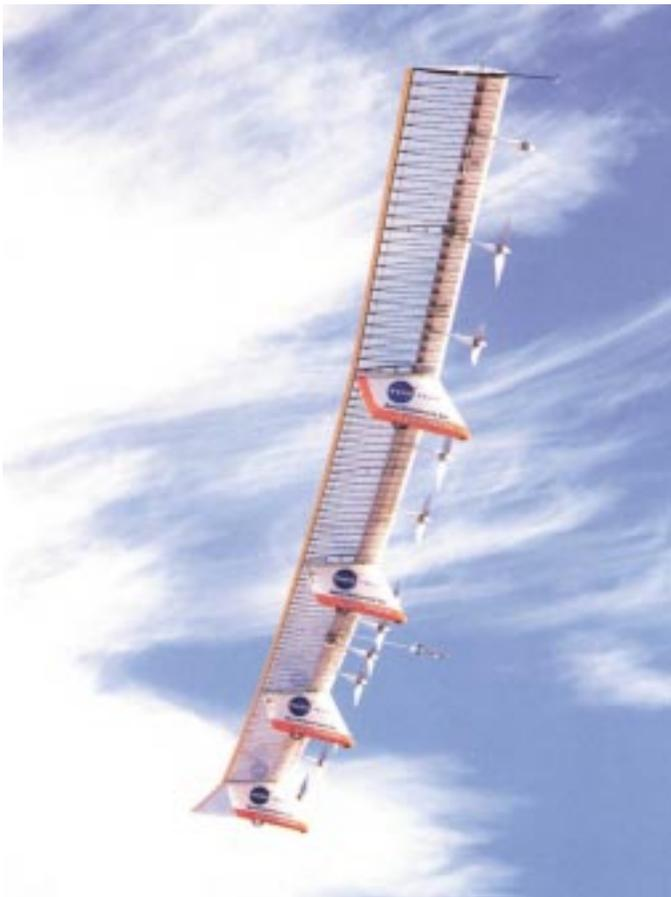
*Centurion is a remotely piloted prototype of a solar-powered airplane that can fly to high altitude, remaining aloft for extended periods. High above Earth, the NASA-sponsored research plane will carry science equipment to perform upper-atmosphere measurements.*
